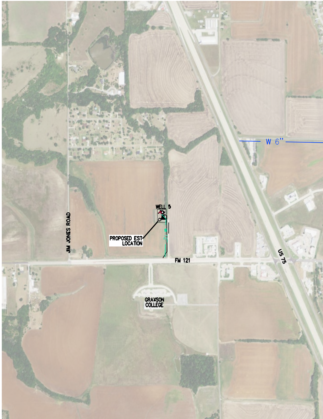
PROPOSED ELEVATED STORAGE TANK LOCATION WELL SITE #5 (NTS)
