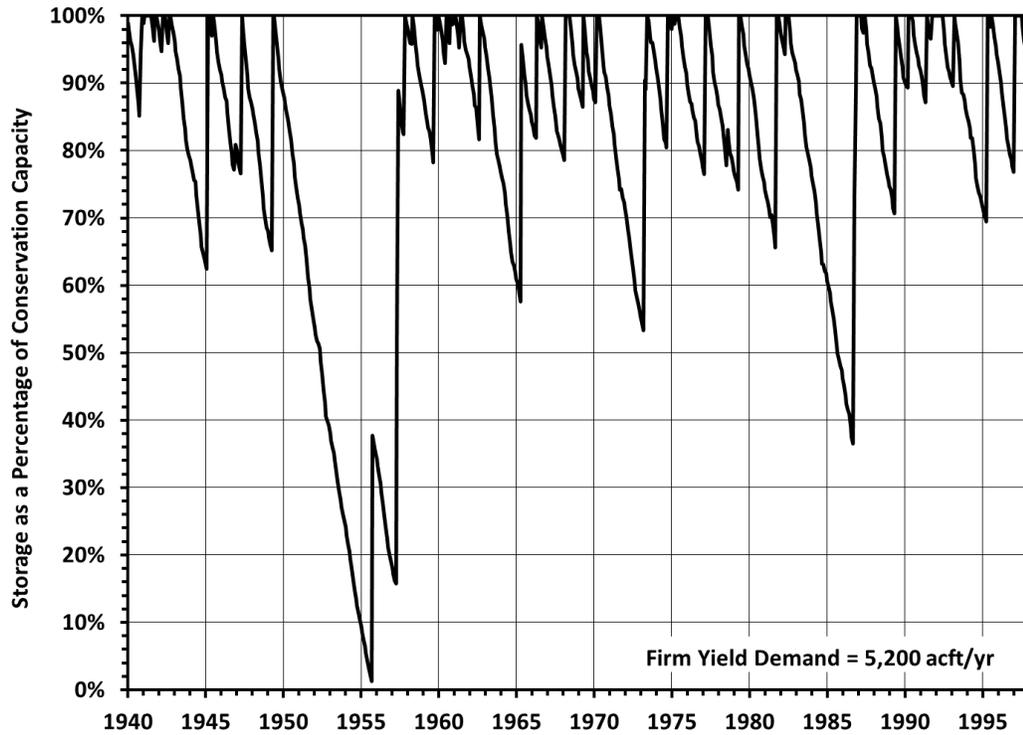
**Figure 10.4-6. Storage Frequency associated with Firm Yield**
