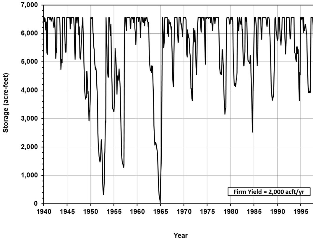
Figure 4.2-3. Storage Frequency Curve for Brushy Creek Reservoir
