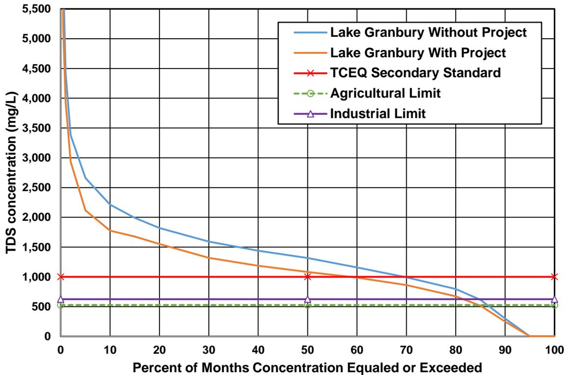
Figure 11-14. Model-Predicted TDS Concentration-Duration Curve at Lake Whitney
