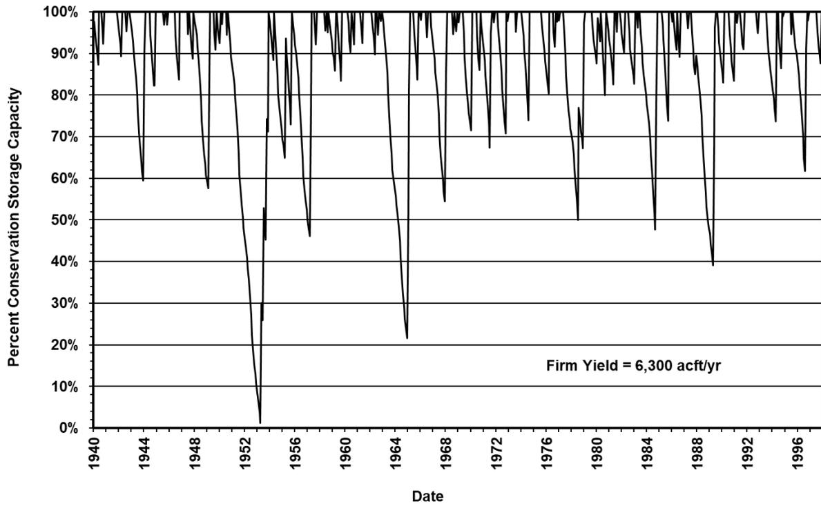
Figure 4.1-4. Hopes Creek Off-Channel Reservoir Storage Frequency
