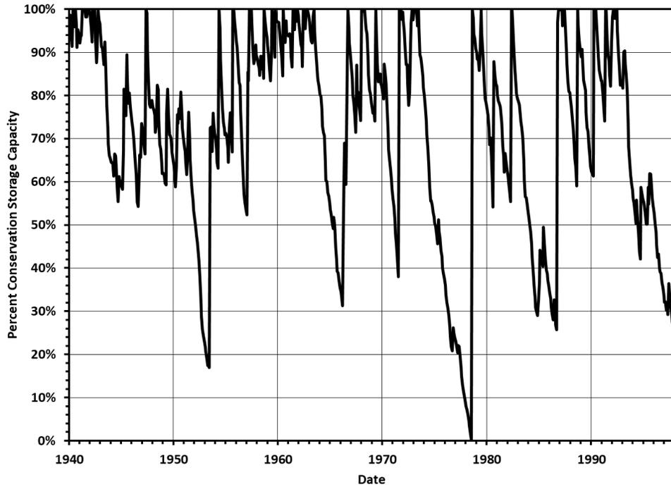
**Figure 10.5-5. Millers Creek Reservoir Firm Yield Storage Frequency with Canal Diversion**
