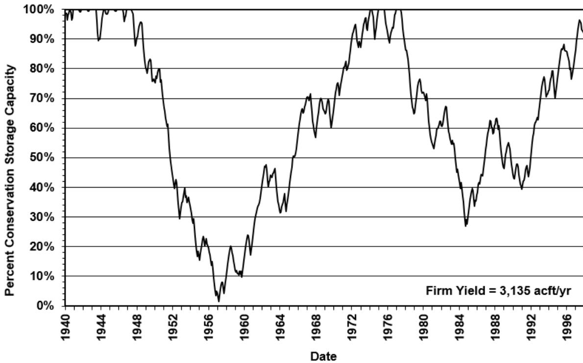
Figure 4.4-4. Coryell County Off-Channel Reservoir Storage Frequency at Firm Yield
