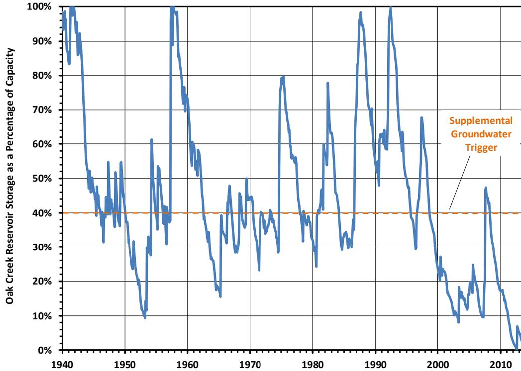
**Figure 7.2-4. Oak Creek Reservoir Simulated Storage Frequency under Conjunctive Use Operations**
