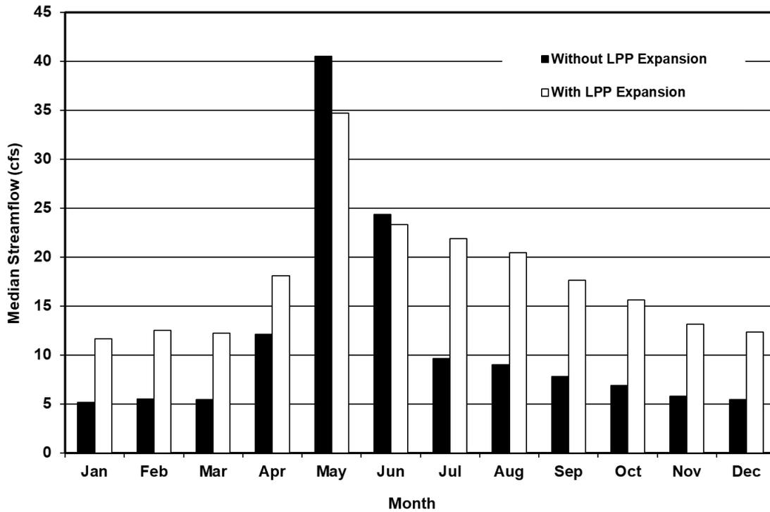
Figure 4.11-6. Streamflow Frequency Comparison at Turkey Peak Dam
