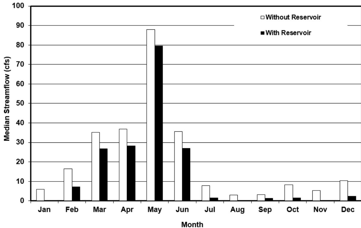
Figure 4.4-6. Cowhouse Creek Diversion Streamflow Frequency Comparison
