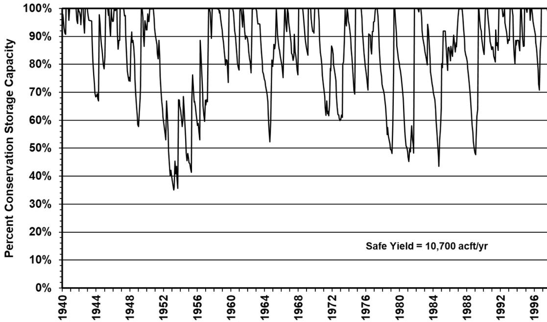
Figure 4.11-3. Expanded Lake Palo Pinto Reservoir Storage Frequency
