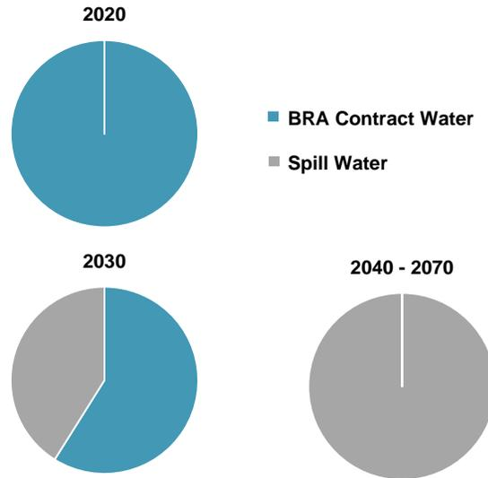
Figure 8.3-4. Simulated Timeline of Recharge by Planning Decade
