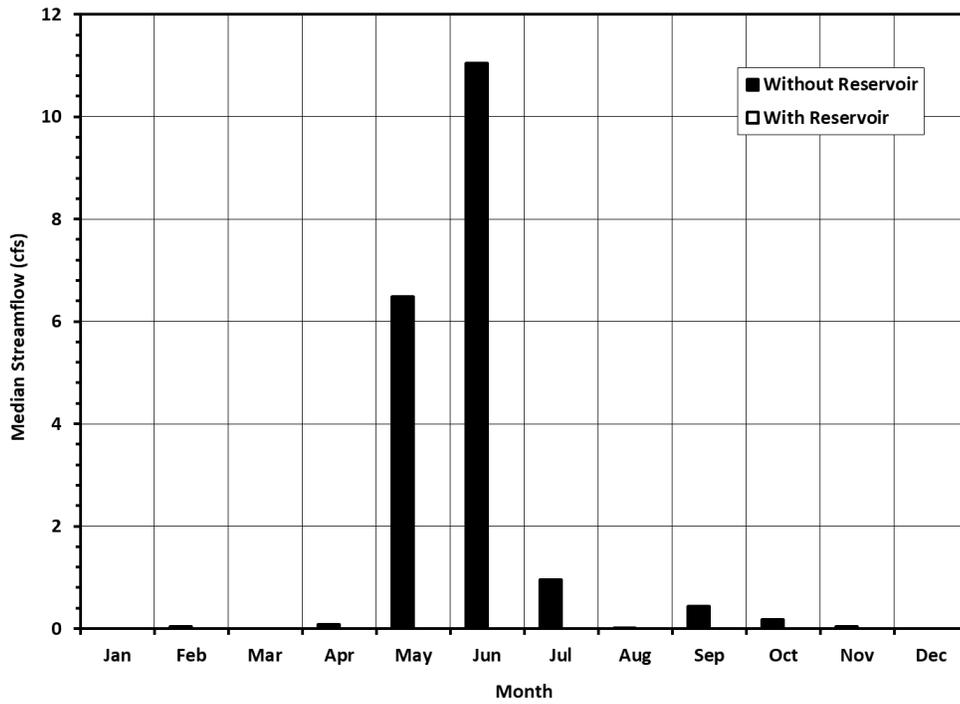
Figure 4.7-7. Lake Creek Streamflow Frequency Comparison
