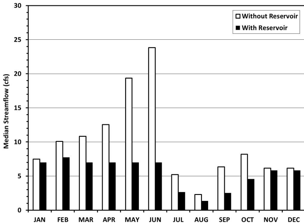
**Figure 4.3-5. Cedar Ridge Reservoir Streamflow Frequency Comparison**
