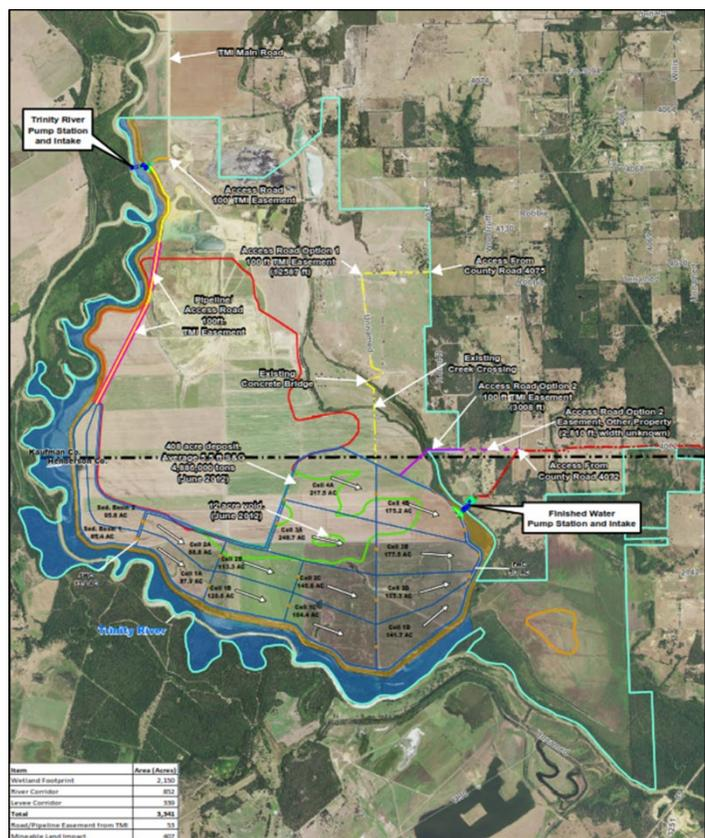
This strategy addresses the development of a reuse project at Cedar Creek Reservoir, which includes a new diversion structure, created wetlands, and infrastructure necessary to discharge the treated return flows into Cedar Creek Reservoir. The wetlands will be constructed adjacent to the Trinity River, east of the City of Ennis as shown. The reuse supplies would then be diverted from the lake and transported by the Integrated Pipeline (see Integrated Pipeline Technical Memorandum).
