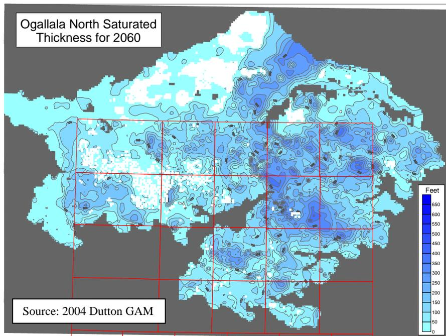
**Figure 3-10 Projected Northern Ogallala Aquifer Saturated Thickness in 2060 with Unrestricted Projected Pumpage**
