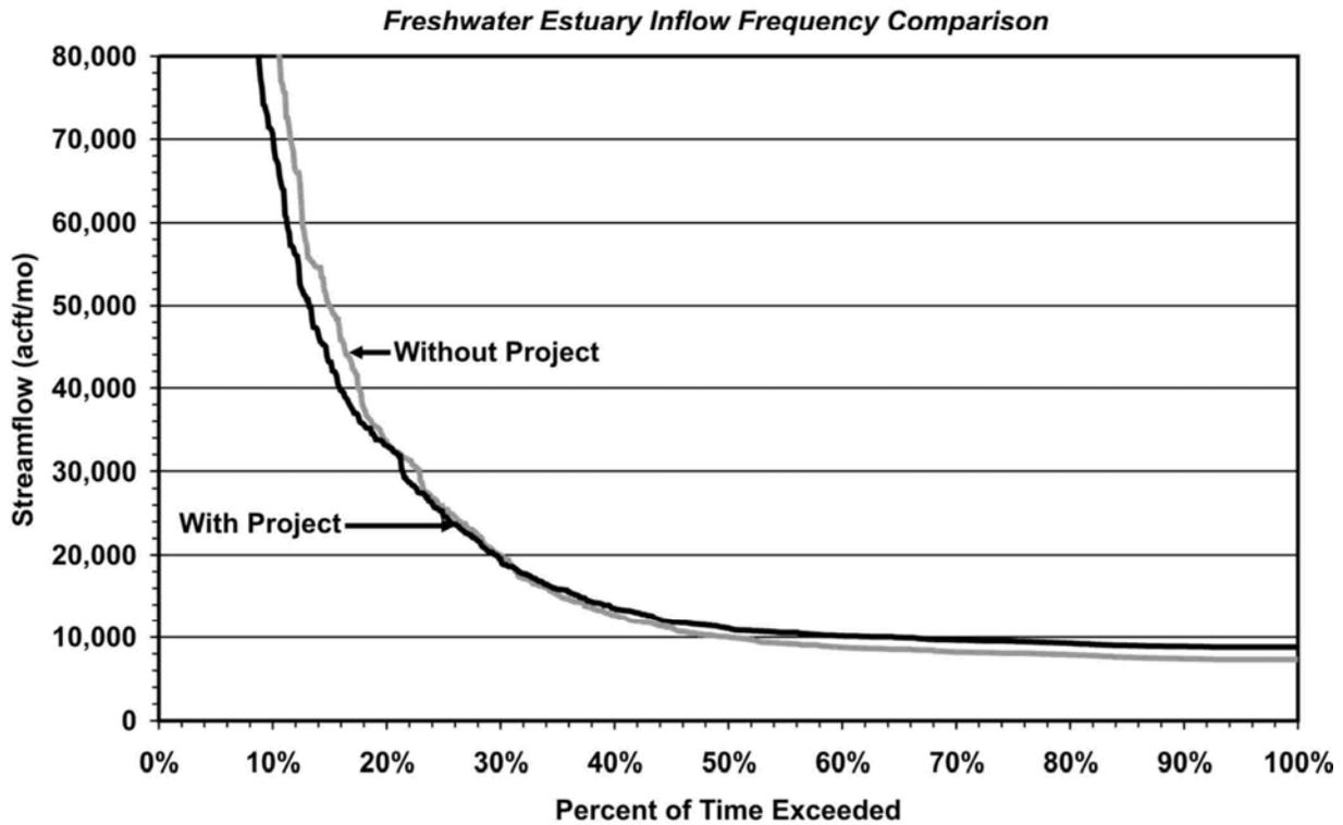
Results based on Phase IV operating policy, 2060 sediment conditions, the 2001 Agreed Order, 750 cfs pipeline delivery rate, 200,000 acft reservoir, and demand of 168,500 acft/yr without project and 202,500 acft/yr with off-channel reservoir.
