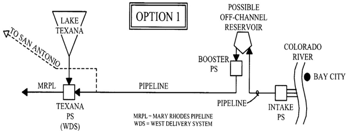
**Figure 4C-14.2 Delivery Option 1 – Combined Facilities with LCRA/SAWS**
