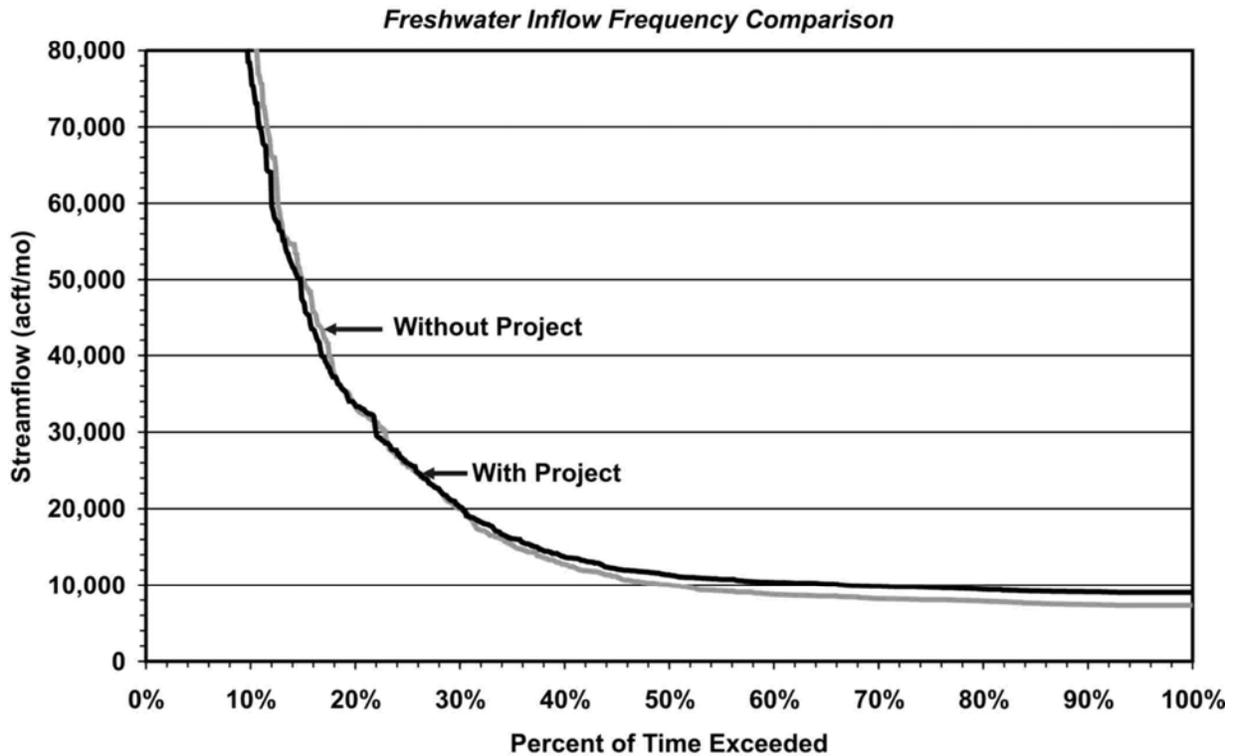
Results based on Phase IV operating policy, 2060 sediment conditions, the 2001 Agreed Order, 300 cfs pipeline delivery rate, and a demand of 168,500 acft/yr without project and 208,000 acft/yr with CCR/LCC Pipeline.
