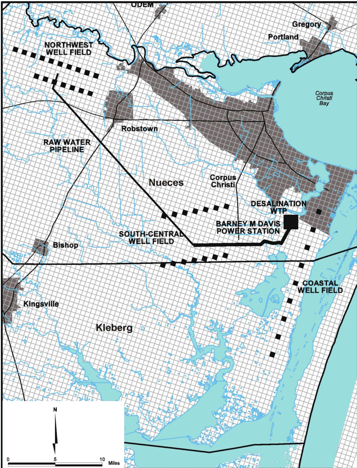
**Figure 4C.17-1. Combined Seawater and Brackish Groundwater Desalination at Barney M. Davis Power Plant**
