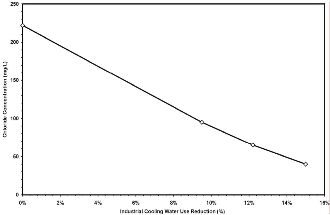
**Figure 4C.3-11. Potential for Manufacturing Water Use Savings Based on Reduction in Chlorides**
