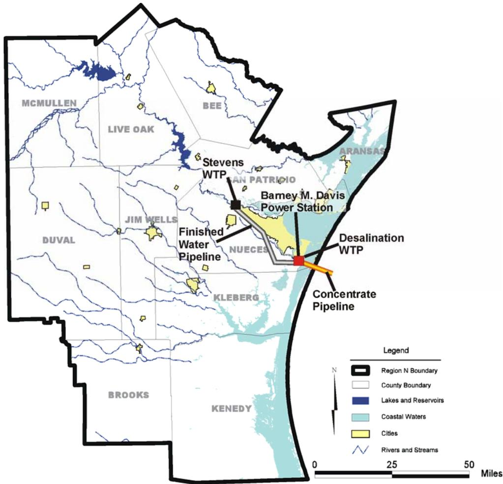
**Figure 4C.17-2. Desalination Plant Location and Pipeline Route**
