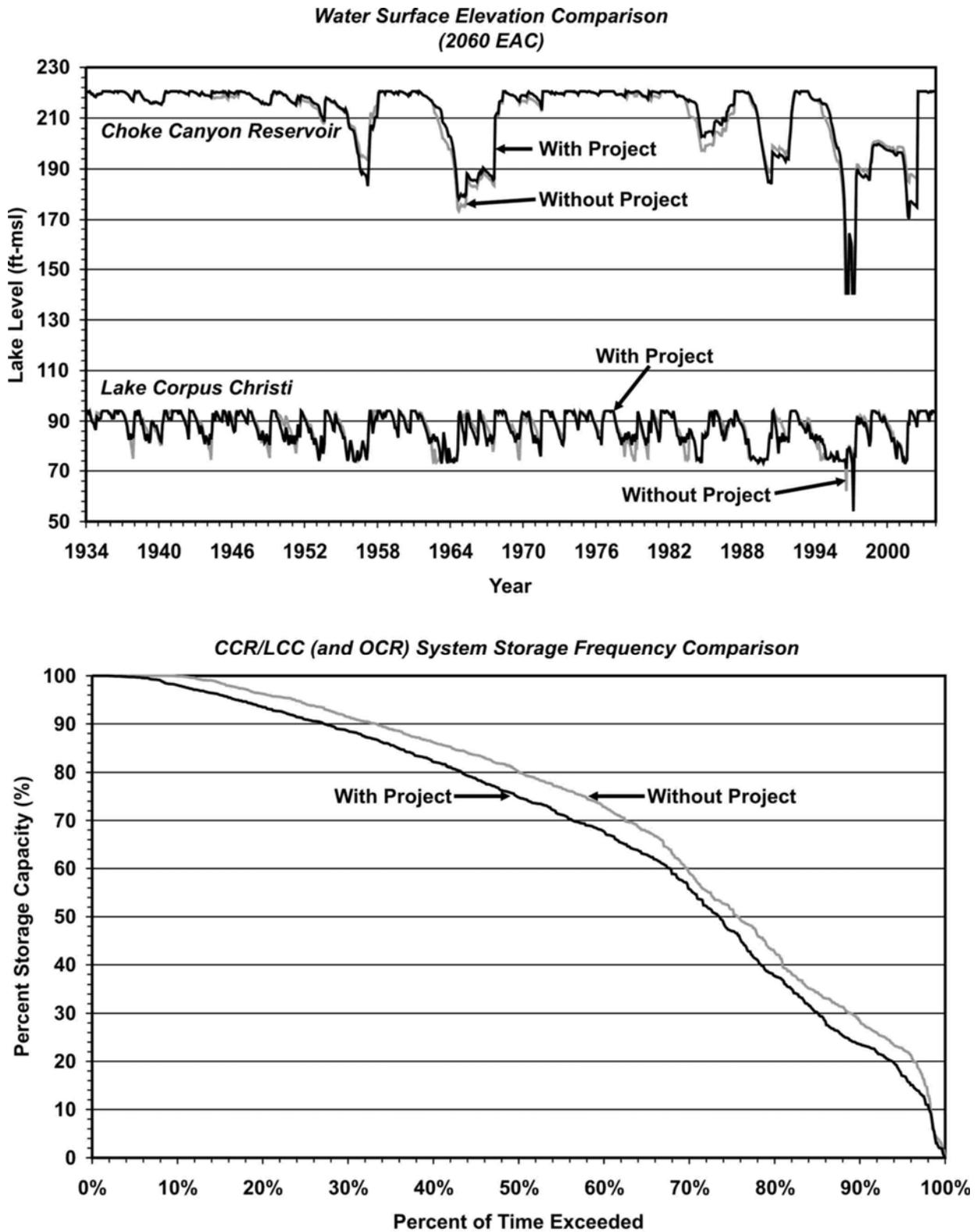
Results based on Phase IV operating policy, 2060 sediment conditions, the 2001 Agreed Order, 750 cfs pipeline delivery rate, 200,000 acft reservoir, and demand of 168,500 acft/yr without project and 202,500 acft/yr with off-channel reservoir.
