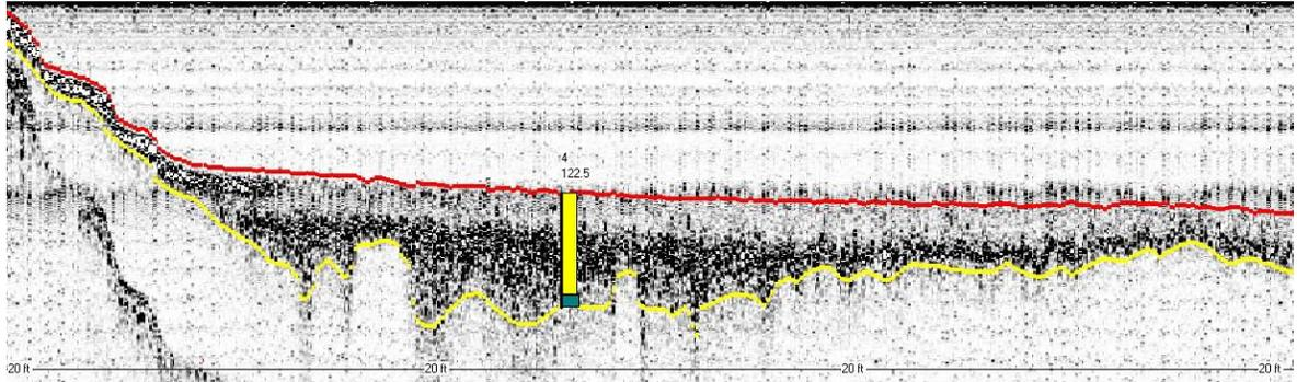
**Figure 10.** Cross-section of data collected during 2009 survey, displayed in DepthPic (50 kHz frequency), correlated with sediment core sample T-4 and showing the current surface in red and pre-impoundment surface in yellow
