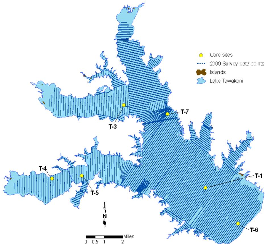
**Figure 3. Locations of sediment core samples relative to the 2009 TWDB survey data (Note: Sample T-2 was unrecoverable due to field conditions and is not shown)**
