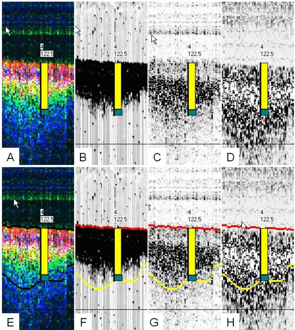
Figure 11. Comparison of sediment core T-4 with acoustic signal returns A,E) combined acoustic signal returns, B,F) 200 kHz frequency, C,G) 50 kHz frequency, D,H) 24 kHz frequency
