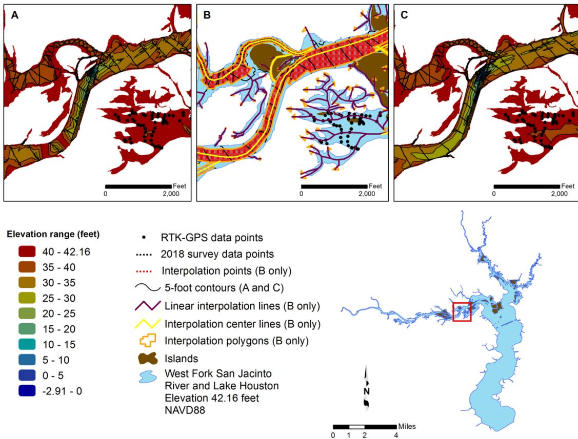
**Figure 3.** Anisotropic spatial interpolation and linear interpolation of the West Fork San Jacinto River sounding data; A) bathymetric contours without interpolated points, B) sounding points (*black*) and interpolated points (*red*), C) bathymetric contours with interpolated points.
