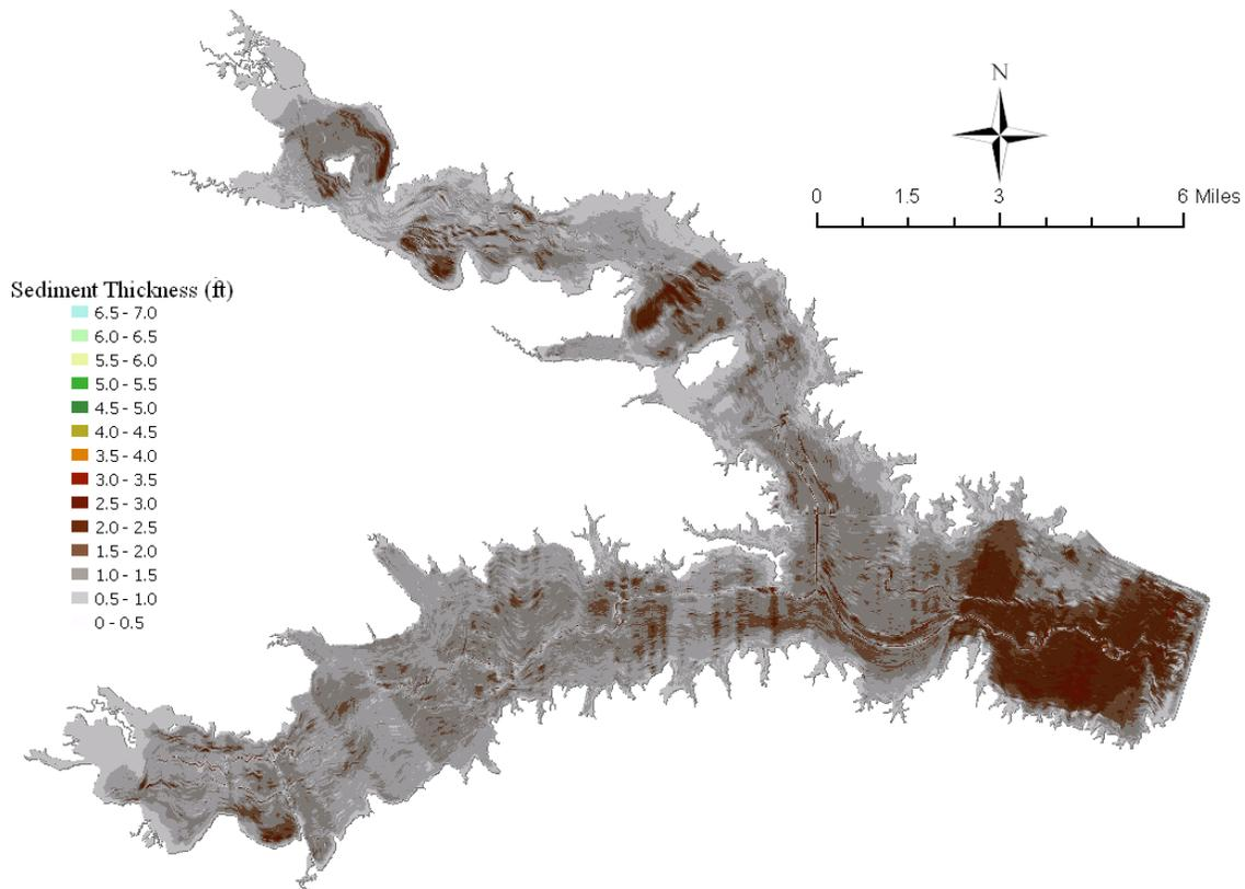
Figure D4 - Sediment thicknesses in Richland-Chambers Reservoir derived from multi-frequency sounding data.
