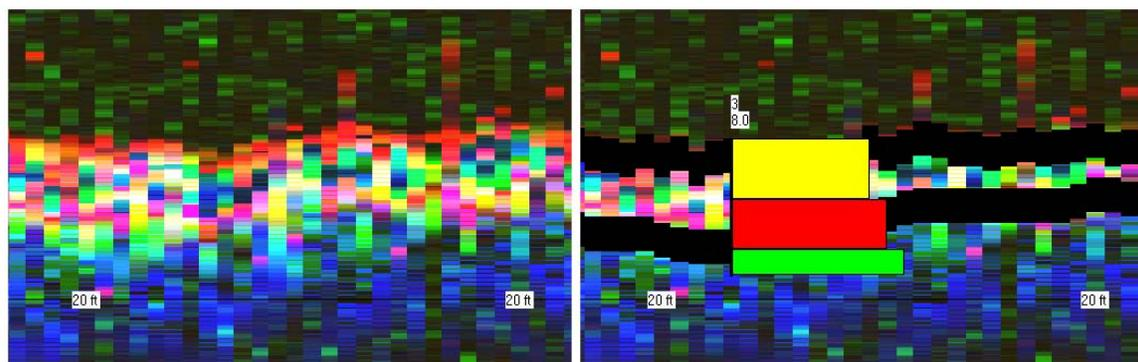
Figure D3 – DepthPic and core sample use in identifying the pre-impoundment bathymetry.
