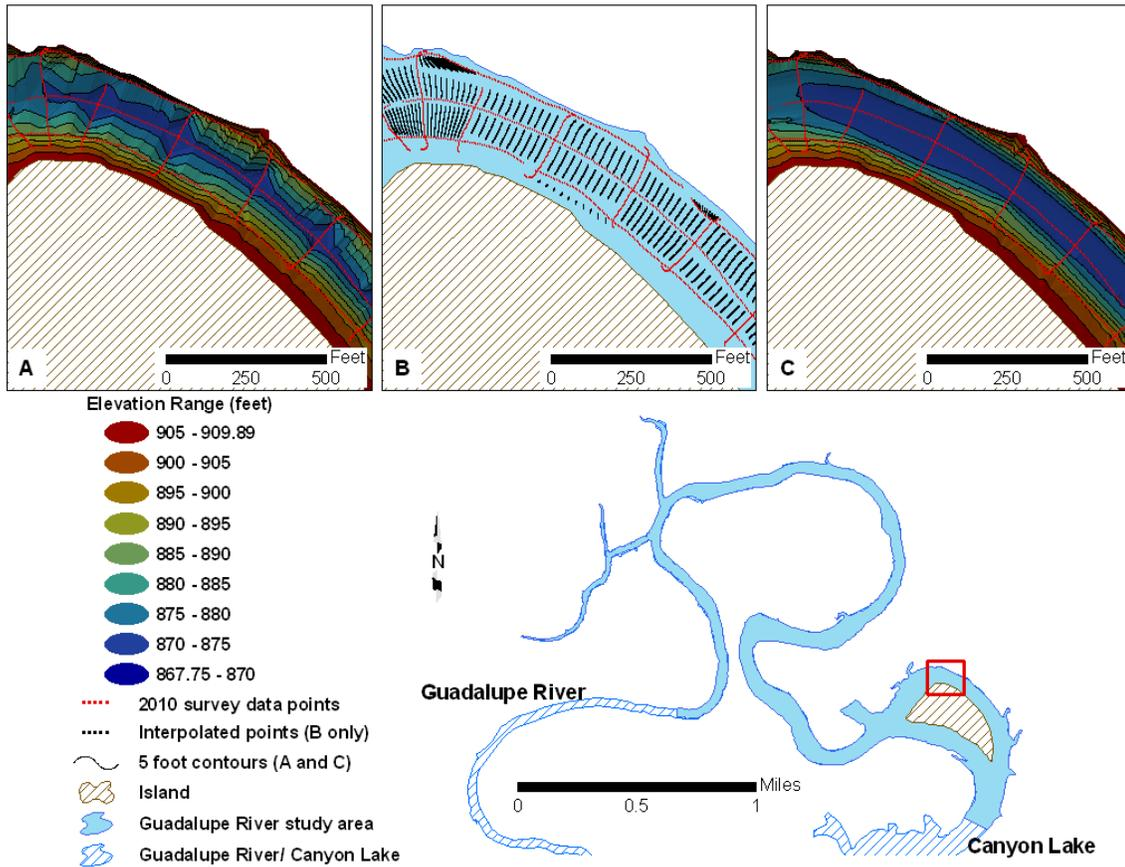
**Figure 3.** Application of the self-similar interpolation technique to the Guadalupe River sounding data – A) bathymetric contours without interpolation, B) sounding points (red) and interpolated points (black) with river boundary at elevation 909.89 feet, C) bathymetric contours with interpolation.
