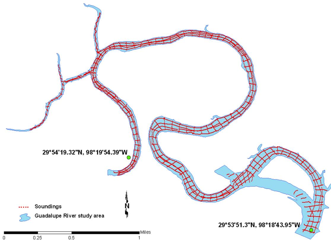
**Figure 2.** Survey data collected during 2010 TWDB survey
