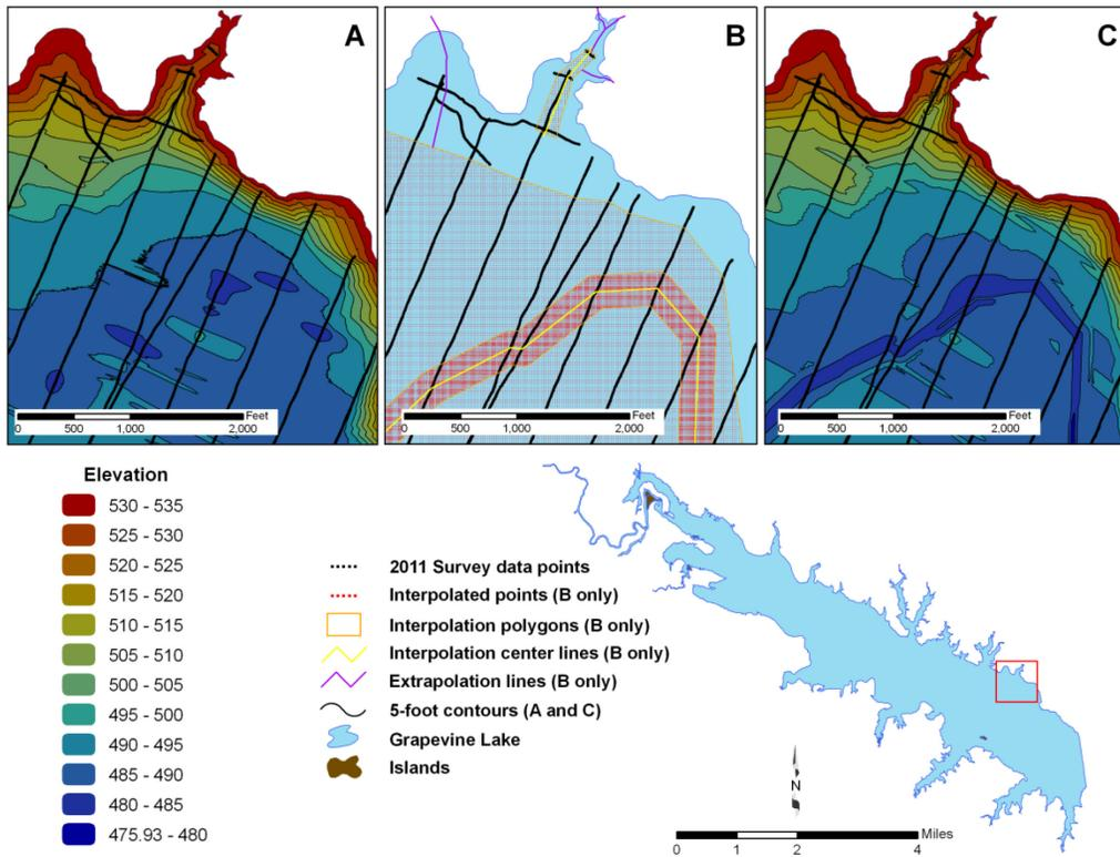
**Figure 6.** Anisotropic spatial interpolation and line extrapolation of Grapevine Lake sounding data – A) bathymetric contours without interpolated points, B) sounding points (black) and interpolated points (red), C) bathymetric contours with the interpolated points
