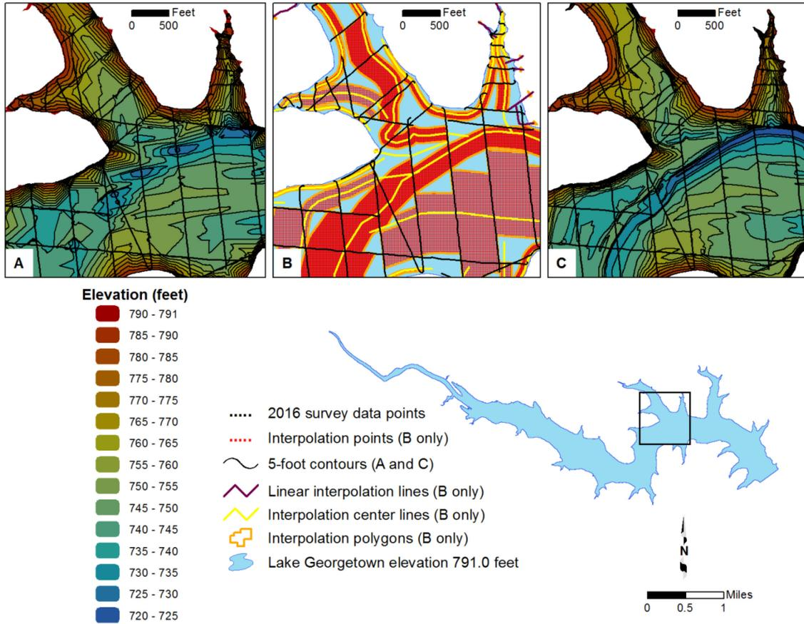
**Figure 3.** Anisotropic spatial interpolation and linear interpolation of Lake Georgetown sounding data; A) bathymetric contours without interpolated points, B) sounding points (*black*) and interpolated points (*red*), C) bathymetric contours with interpolated points.
