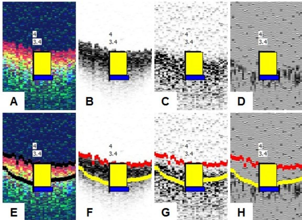
**Figure 8.** Comparison of sediment core GT-4 with acoustic signal returns A, E) combined acoustic signal returns, B, F) 208 kHz frequency, C, G) 50 kHz frequency, and D, H) 24 kHz frequency.
