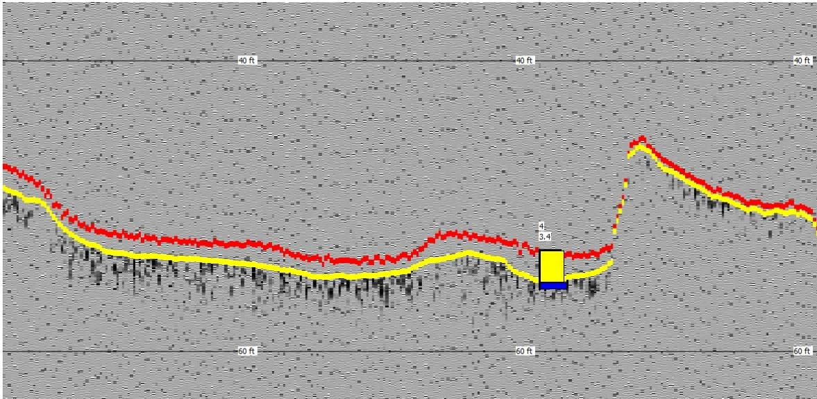
**Figure 9.** Cross-section of data collected during the 2016 survey, displayed in DepthPic© (24 KHz acoustic signal returns), correlated with sediment core sample GT-4 and showing the current surface as the top red line, and pre-impoundment surface as the bottom yellow line.
