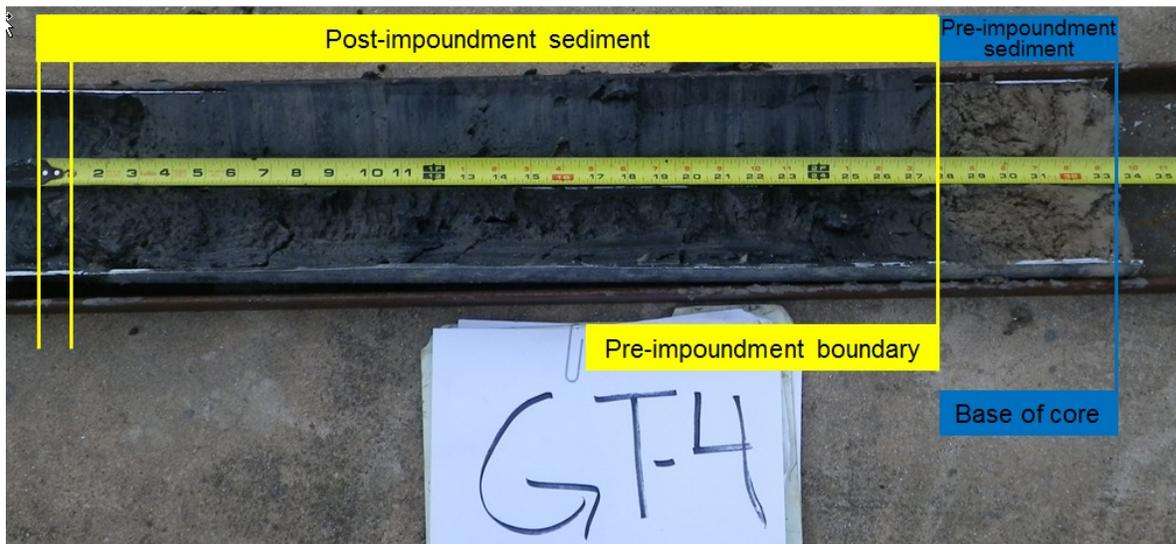
**Figure 7. Sediment core GT-4 from Lake Georgetown. Post-impoundment sediment layers occur in the top 27.75 inches of this sediment core (identified by yellow boxes). Pre-impoundment sediment layers were identified and are defined by the blue box.**
