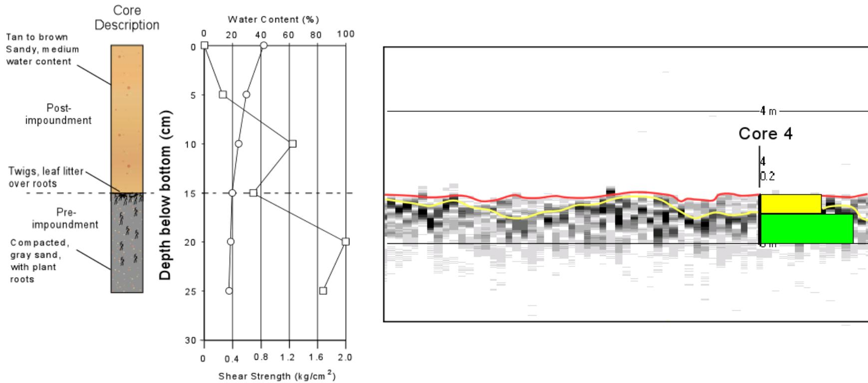
Figure 3-5. Core and acoustic results for site CKE4. (a) Physical analysis of Core 4, showing 15 cm of post-impoundment sediment over pre-impoundment. (b) Short acoustic profile showing only the 48 kHz acoustic signal. On the acoustic data, the red line marks the water bottom and the yellow line marks the interpreted pre-impoundment surface.
