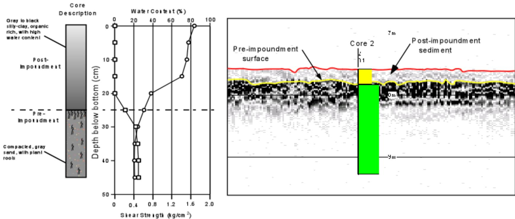
Figure 3-3. Core and acoustic results for site CKE2. (a) Physical analysis of Core 2, showing 25 cm of post-impoundment sediment over pre-impoundment. (b) Short acoustic profile showing only the 48 kHz acoustic signal. On the acoustic data, the red line marks the water bottom and the yellow line marks the interpreted pre-impoundment surface.
