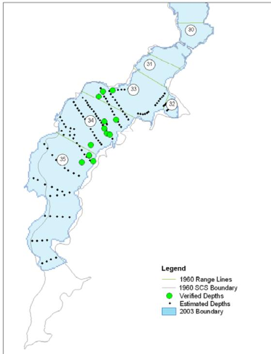
Figure 3. The figure to the left illustrates differences in surface acreage between the 1960 and 2003 boundaries. The area containing segment-35, established for the 1960 SCS report, is about 120 acres smaller in the 2003 report. Depths of 1 ft to 2 ft were assumed for an area of approximately 500 acres, contained in segments 34 and 35. Predominated by Beaver Marsh, this area contains heavy aquatic vegetation.
