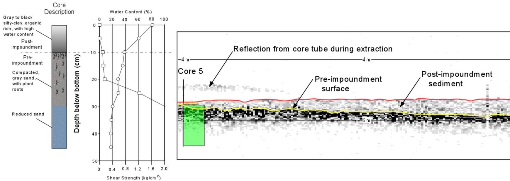
Figure 3-6. Core and acoustic results for site CKE5. (a) Physical analysis of Core 5, showing 10 cm of post-impoundment sediment over pre-impoundment. (b) Short acoustic profile showing only the 48 kHz acoustic signal. On the acoustic data, the red line marks the water bottom and the yellow line marks the interpreted pre-impoundment surface.
