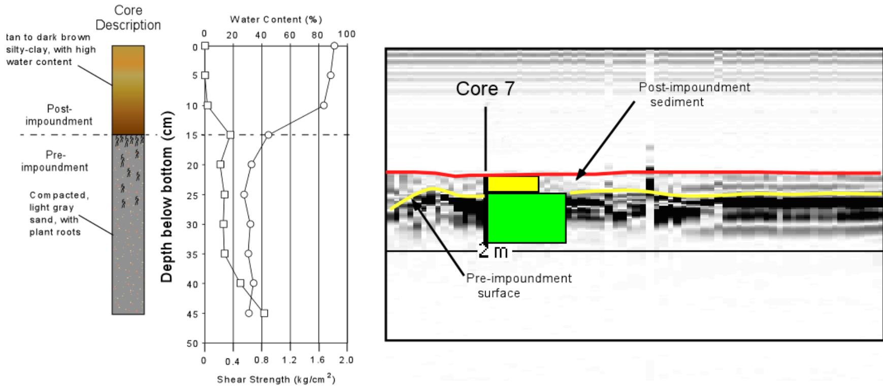
Figure 3-8. Core and acoustic results for site CKE7. (a) Physical analysis of Core 7, showing 15 cm of post-impoundment sediment over pre-impoundment. (b) Short acoustic profile showing only the 48 kHz acoustic signal. On the acoustic data, the red line marks the water bottom and the yellow line marks the interpreted pre-impoundment surface.
