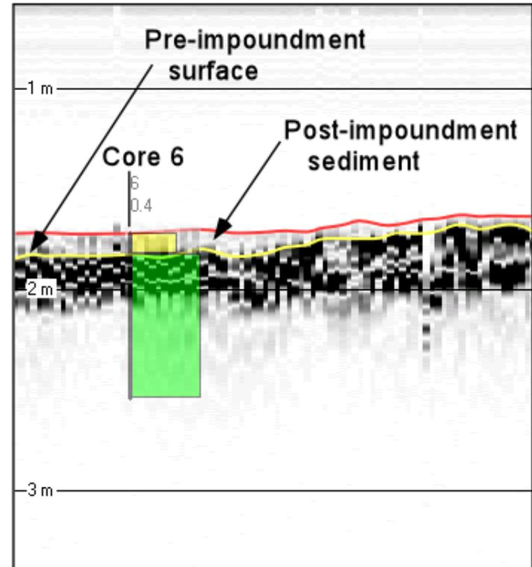
Figure 3-7. Core and acoustic results for site CKE6. (a) Physical analysis of Core 6, showing 10 cm of post-impoundment sediment over pre-impoundment. (b) Short acoustic profile showing only the 48 kHz acoustic signal. On the acoustic data, the red line marks the water bottom and the yellow line marks the interpreted pre-impoundment surface.
