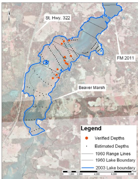
Figure 1. Upstream reach of Lake Cherokee showing range lines established in 1960 by the Soil Conservation Service (SCS). Superimposed on 1995 aerial photos are the 2003 TWDB (blue) and 1960 SCS (light gray) boundaries. The red points indicate where TWDB staff verified depths during the March visit. Smaller black points are estimated depths used in the 2003 model.
