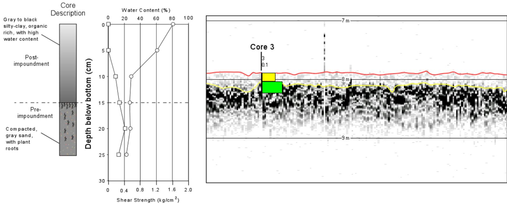
Figure 3-4. Core and acoustic results for site CKE3. (a) Physical analysis of Core 3, showing 15 cm of post-impoundment sediment over pre-impoundment. (b) Short acoustic profile showing only the 48 kHz acoustic signal. On the acoustic data, the red line marks the water bottom and the yellow line marks the interpreted pre-impoundment surface.
