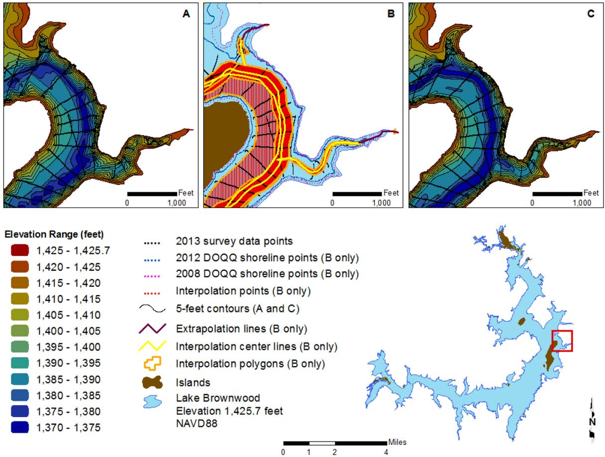
**Figure 3. Anisotropic spatial interpolation and linear extrapolation of Lake Brownwood sounding data - A) bathymetric contours without interpolated points, B) sounding points (black) and interpolated points (red), C) bathymetric contours with the interpolated points**
