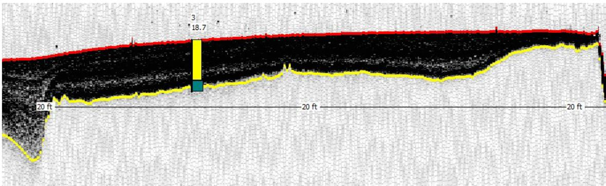
**Figure 9. Cross-section of data collected during 2013 survey, displayed in DepthPic© (200 kHz frequency), correlated with sediment core sample B-3 and showing the current surface in red and pre-impoundment surface in yellow**
