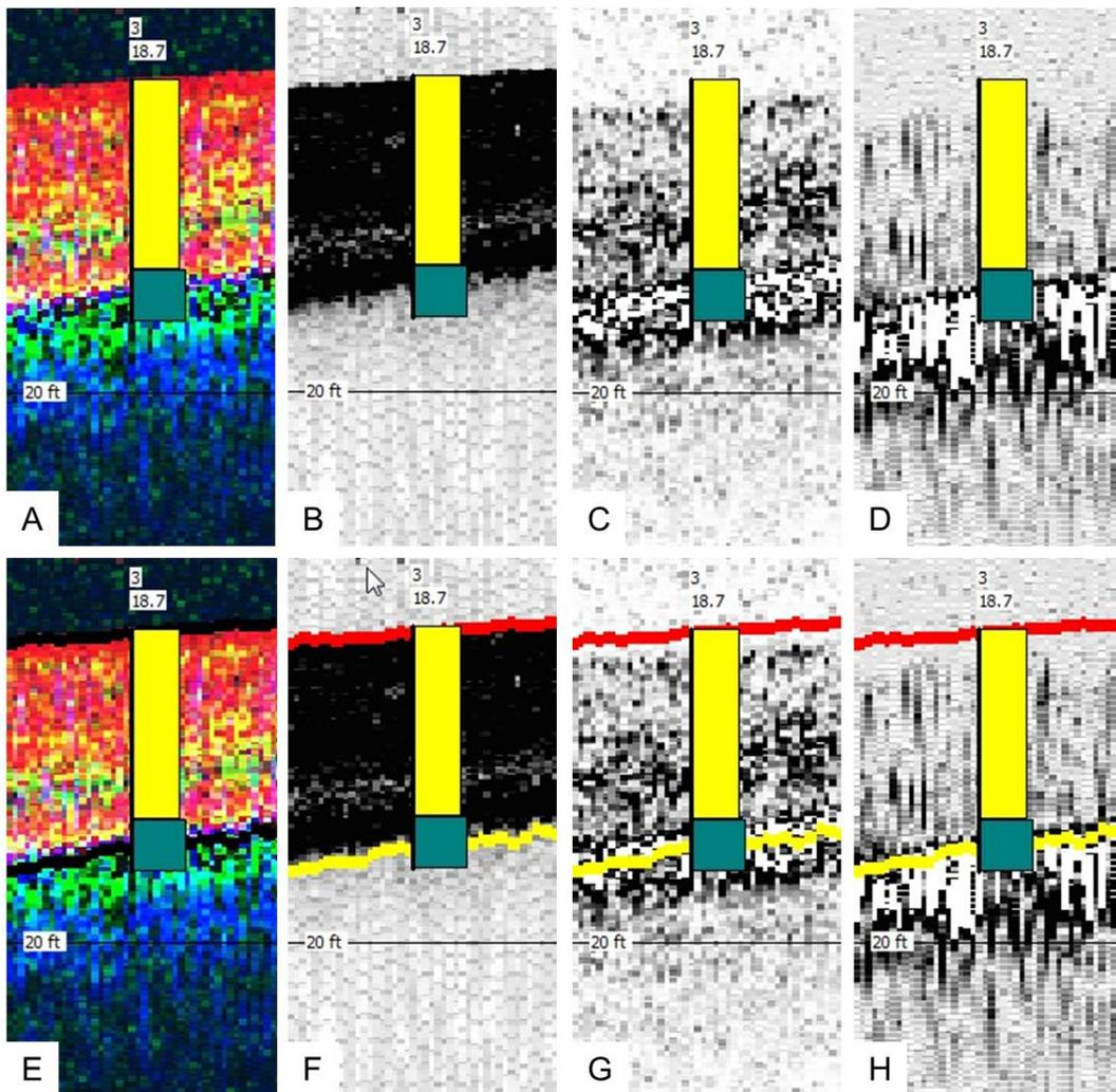
Figure 8. Comparison of sediment core B-3 with acoustic signal returns: A,E) combined acoustic signal returns, B,F) 200 kHz frequency, C,G) 50 kHz frequency, D,H) 24 kHz frequency
