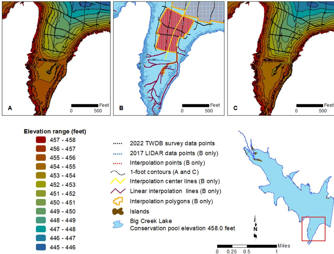
**Figure 3.** Anisotropic spatial interpolation as applied to Big Creek Lake sounding data; A) bathymetric contours without interpolated points, B) sounding points (*black*) and interpolated points (*red*), C) bathymetric contours with interpolated points.
