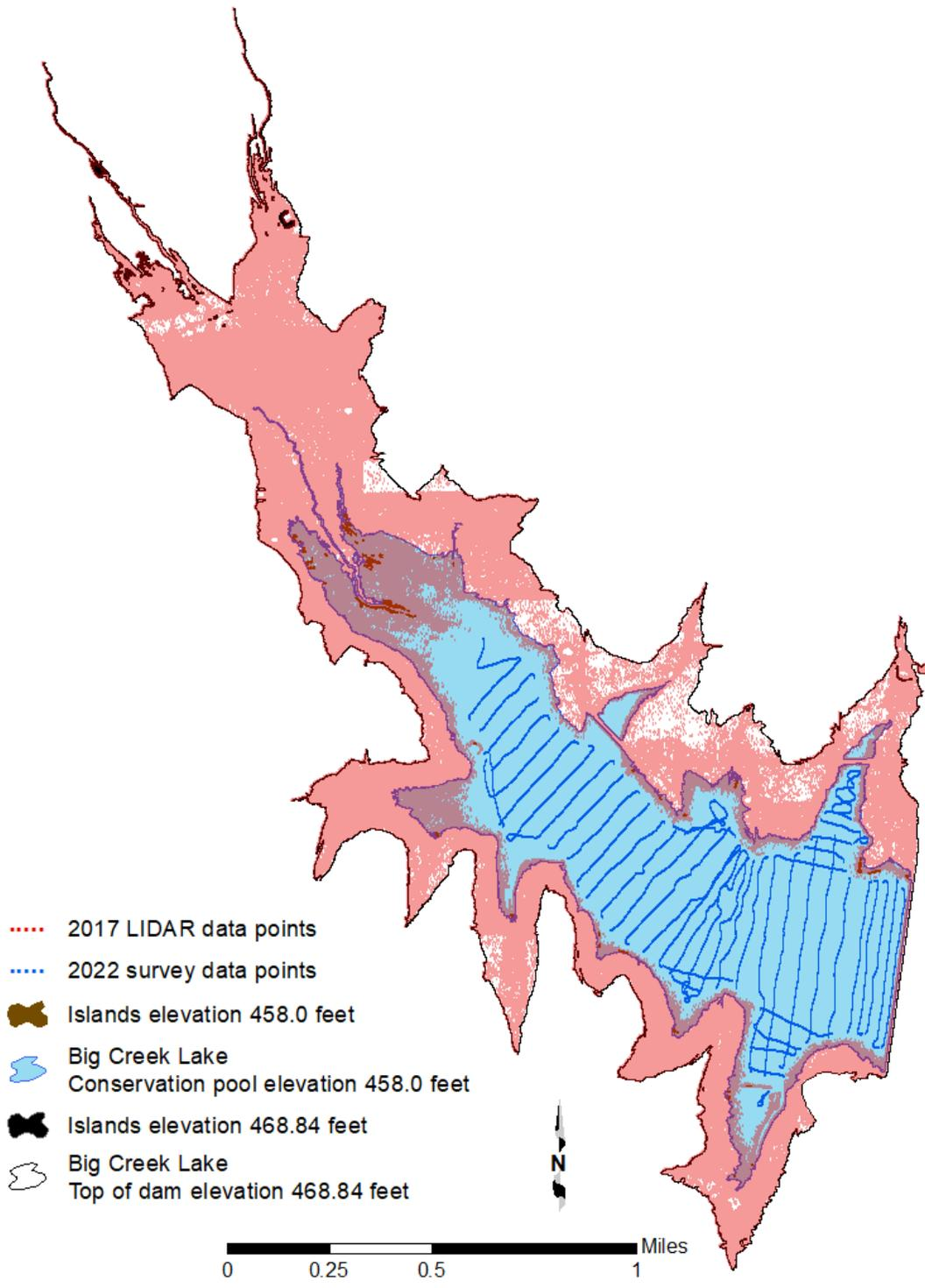
Figure 2. 2022 TWDB sounding data (blue dots) and 2017 LIDAR data points (red dots).
