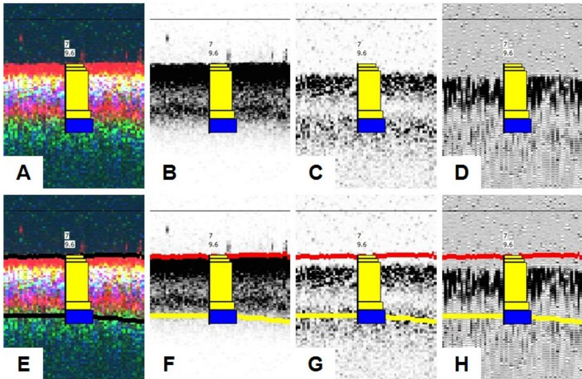
**Figure 8.** Comparison of sediment core BT-7 with acoustic signal returns A, E) combined acoustic signal returns, B, F) 208 kHz frequency, C, G) 50 kHz frequency, and D, H) 24 kHz frequency.
