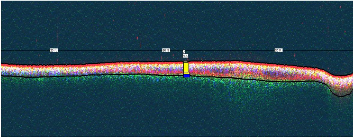
**Figure 9. Cross-section of data collected during the 2015 survey, displayed in DepthPic© (combined acoustic signal returns), correlated with sediment core sample BT-7 and showing the current surface as the top black line, and pre-impoundment surface as the bottom black line.**
