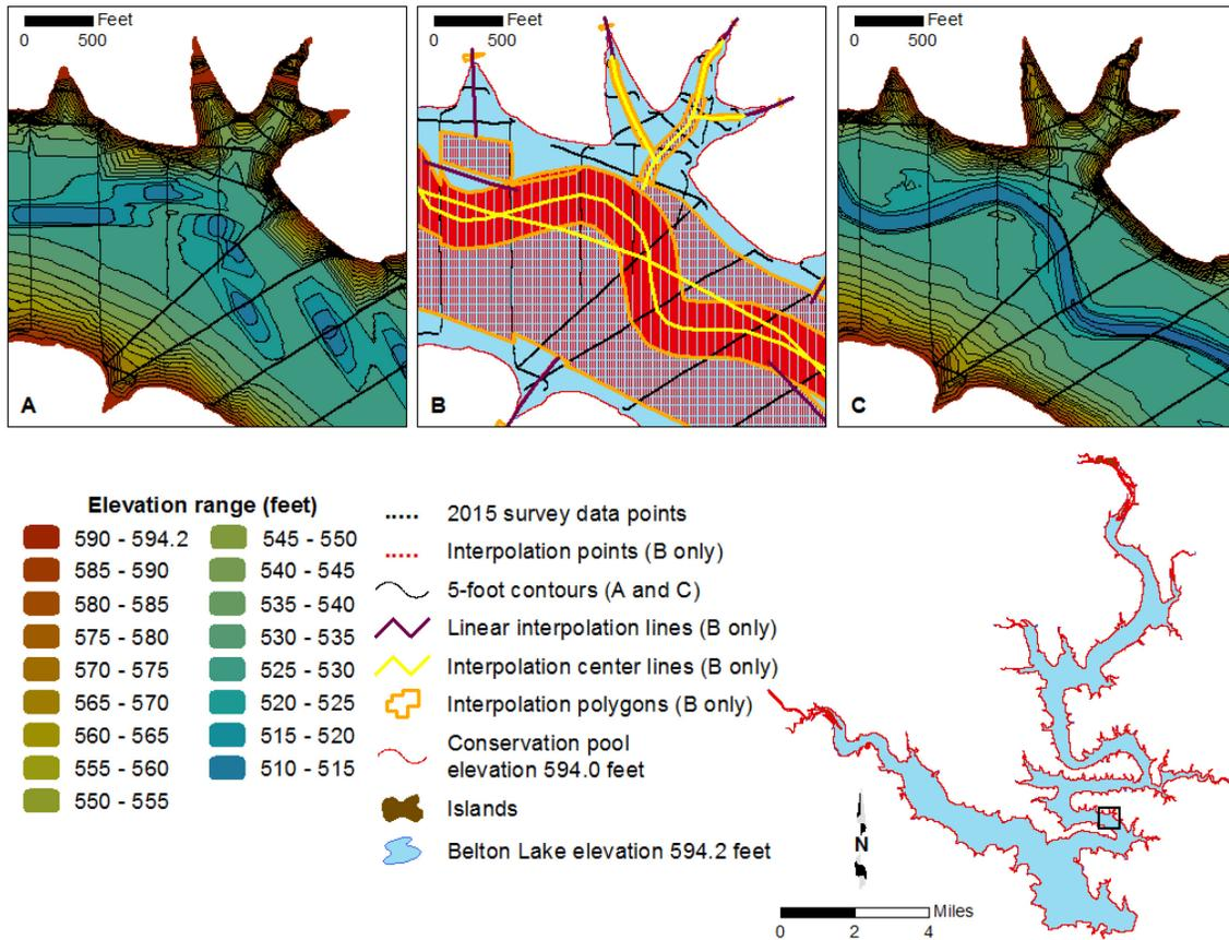
**Figure 3.** Anisotropic spatial interpolation and linear interpolation of Belton Lake sounding data; A) bathymetric contours without interpolated points, B) sounding points (*black*) and interpolated points (*red*), C) bathymetric contours with interpolated points.
