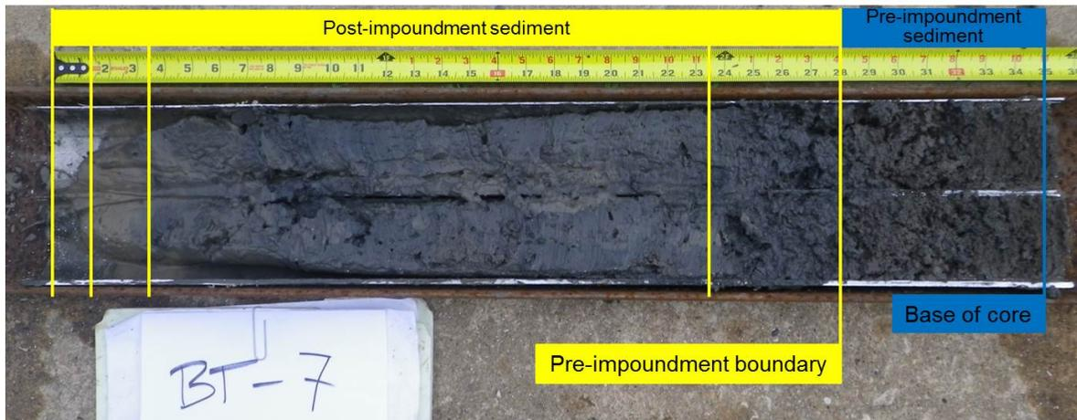
**Figure 7. Sediment core BT-7 from Belton Lake. Post-impoundment sediment layers occur in the top 28 inches of this sediment core (identified by yellow boxes). Pre-impoundment sediment layers were identified and are defined by the blue box.**
