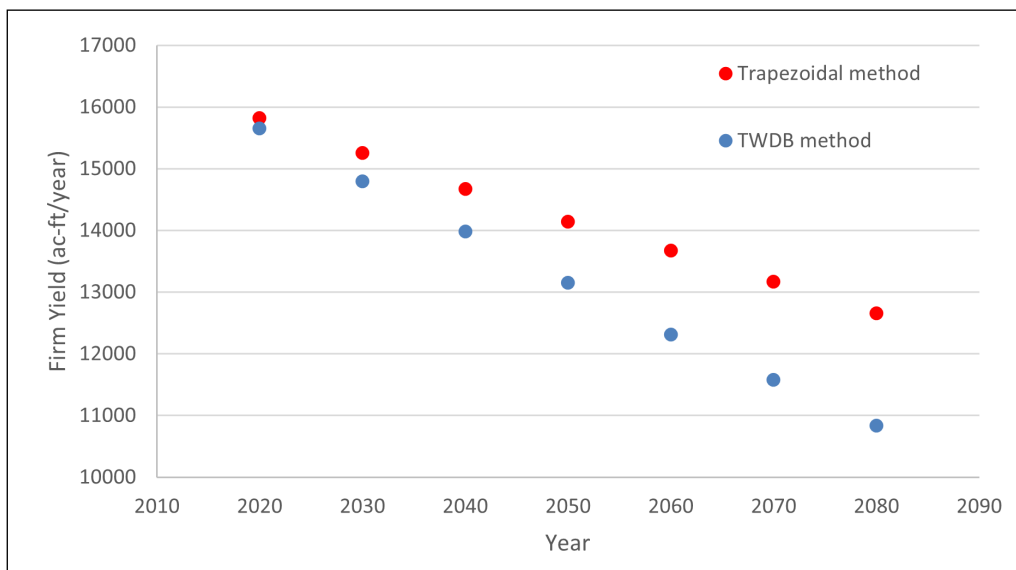
Figure 12. Granger Lake firm yields using rating curves by trapezoidal method (red points) and the volumetric elevational sedimentation rate method (blue points). By 2070, firm yield calculated by trapezoidal method is 1,589 acre-feet per year (about 14%) more than the firm yield estimated by the volumetric elevational sedimentation rate method.
