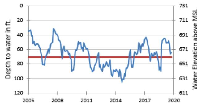
The October water-level measurement in this Edwards (Balcones Fault Zone) Aquifer well, elevation 731 feet above mean sea level, was 64.60 feet below land surface, or 666 feet above mean sea level. This was 0.10 feet below last month's measurement, 17.09 feet below last year's measurement and 17.96 feet below the initial measurement recorded in 1932.
