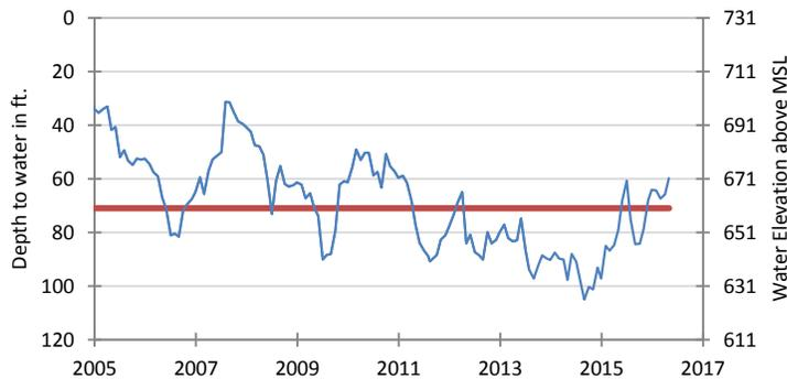
The late April water-level measurement in this Edwards (Balcones Fault Zone) Aquifer well, elevation 731 feet above mean sea level, was 59.81 feet below land surface, or 671.19 feet above mean sea level. This was 6.00 feet above last month's measurement, 19.29 feet above last year's measurement, and 13.17 feet below the initial measurement recorded in 1932.
