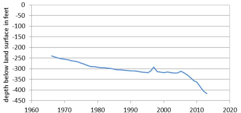
This Ogallala well, drilled to a depth of 474 feet in 1964, is an irrigation well in central Moore County, north of the Canadian River. The water quality is good with total dissolved solids at less than 350 milligrams per liter. The measured yield in 1966 was at 1150 gallons per minute with 38 feet of drawdown, presumably after 36 hours. Water levels have declined 176 feet since the initial measurement in 1966, and the rate of decline has increased since 2005.
