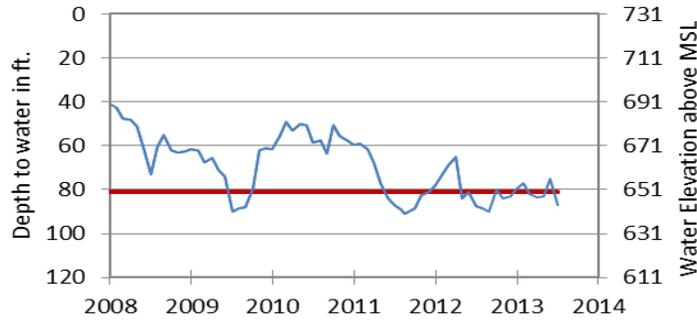
The late June water level measurement in this Edwards (BFZ) Aquifer well, elevation 731 feet above mean sea level, was 86.86 feet below land surface, or 644.14 feet above mean sea level. This was 12.06 feet below last month's measurement, 0.5 feet above last year's measurement, and 40.22 feet below the initial measurement recorded in 1932.
