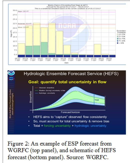
Figure 2: An example of ESP forecast from WGRFC (top panel), and schematic of HEFS forecast (bottom panel). Source: WGRFC.
