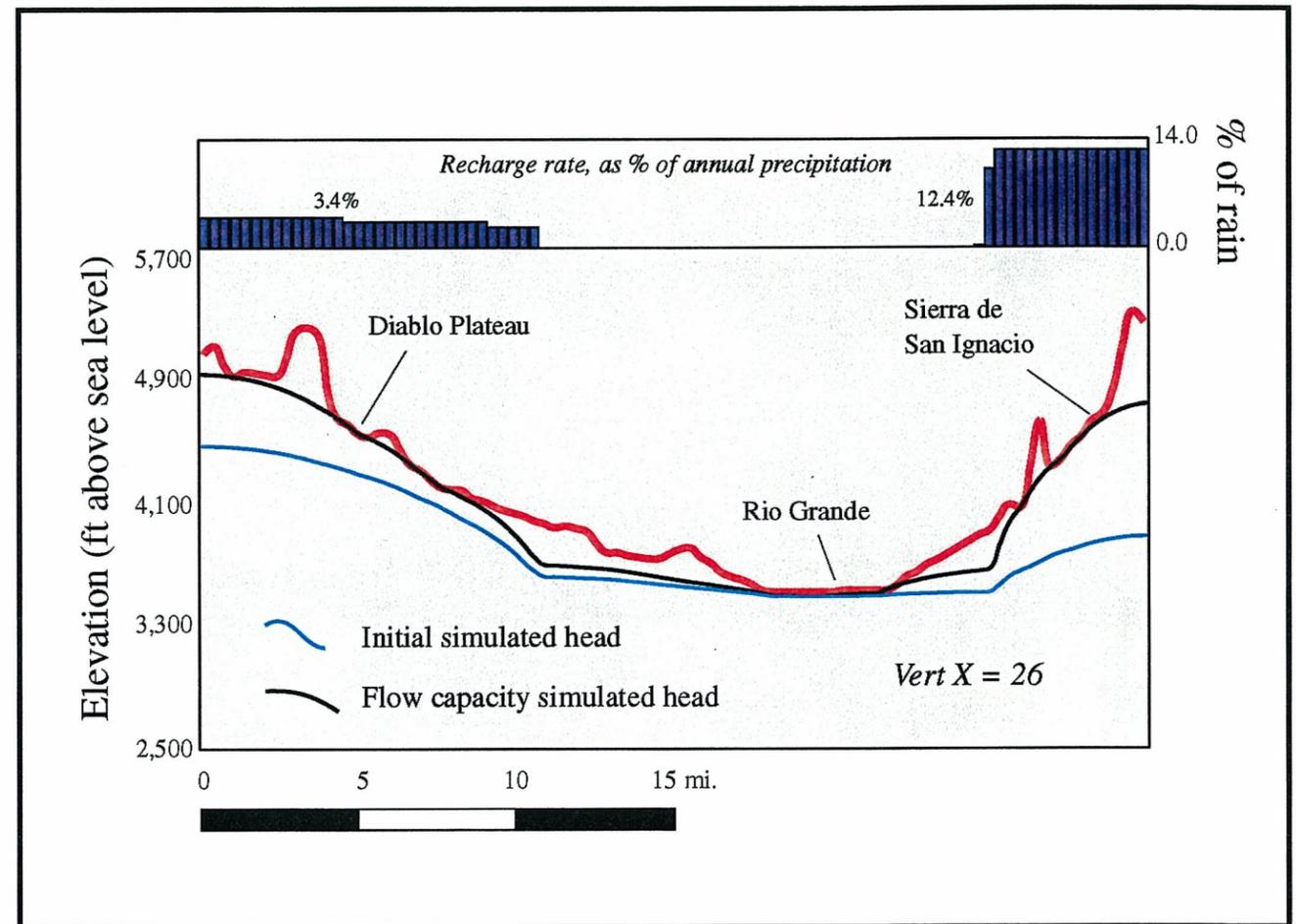
Figure 4.21. Comparison of initial simulated hydraulic head (see Figure 4.12) and simulated hydraulic head at flow capacity; and recharge rates at flow capacity, model scenario 3.
