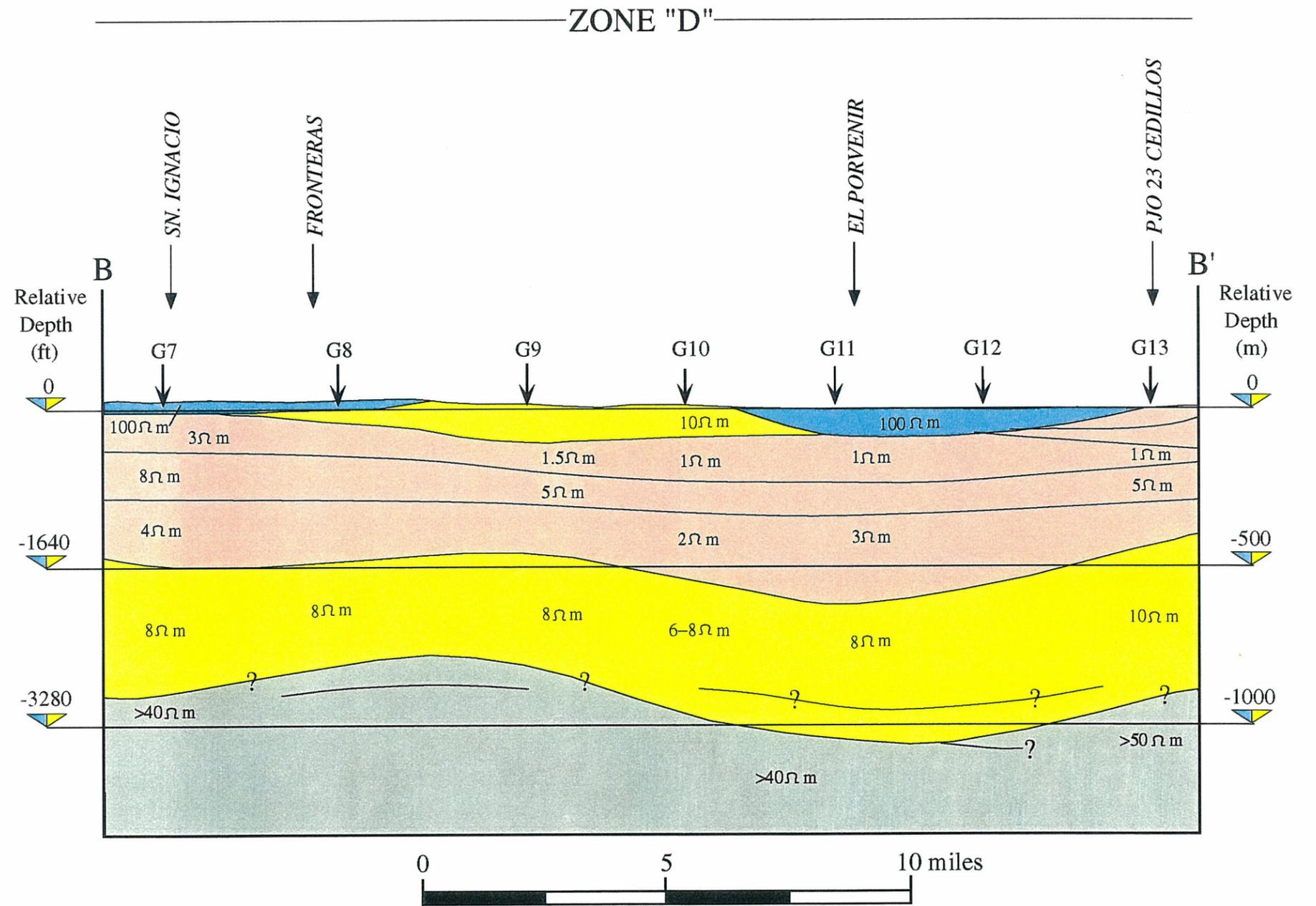
Figure 4.4. Geoelectric cross section B - B' across the southeastern Hueco aquifer, northern Chihuahua, Mexico. The map shows interpreted average real resistivities (modified from Geo Fimex, 1970; line of section shown on Figure 4.1).
