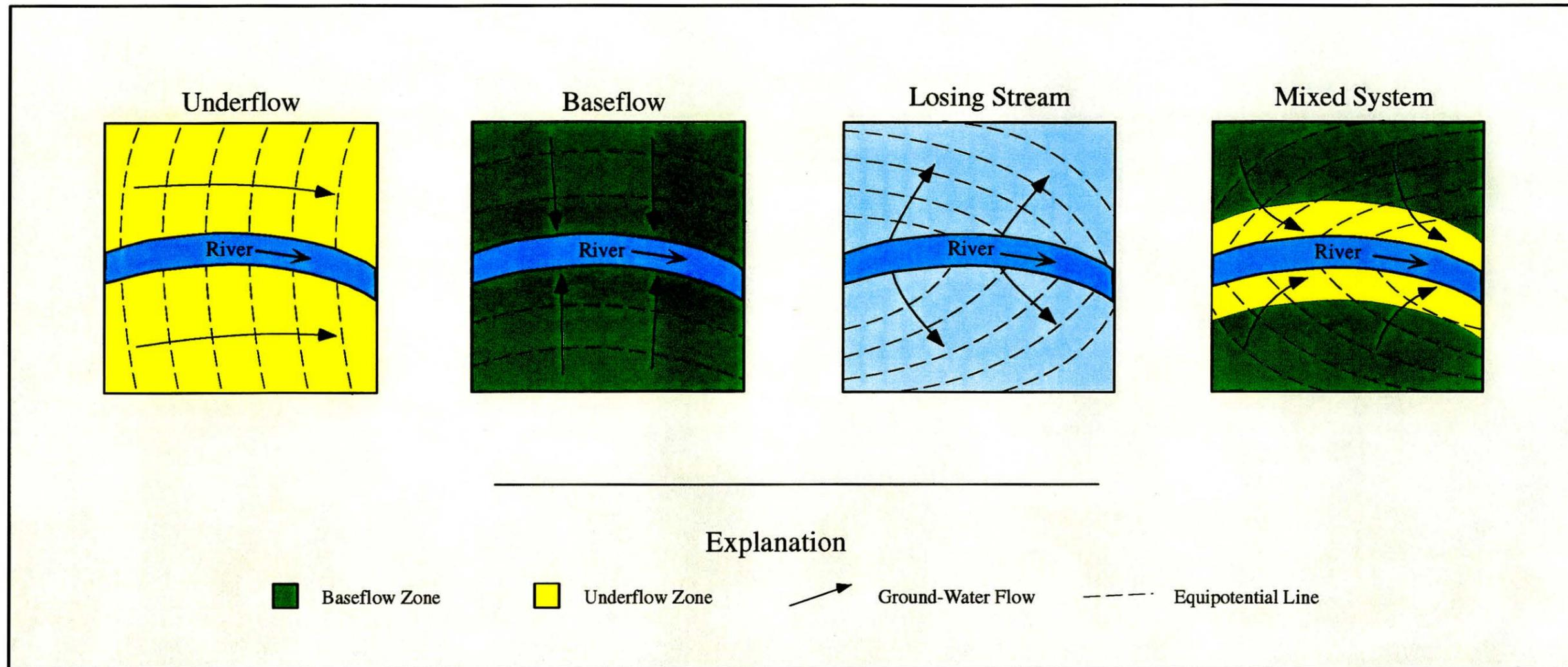
Figure 5.4. Diagram illustrating underflow, baseflow, losing stream, and a mixed system that includes underflow and baseflow components of flow in an alluvial aquifer hydraulically connected to a river (modified from Larkin, 1988).
