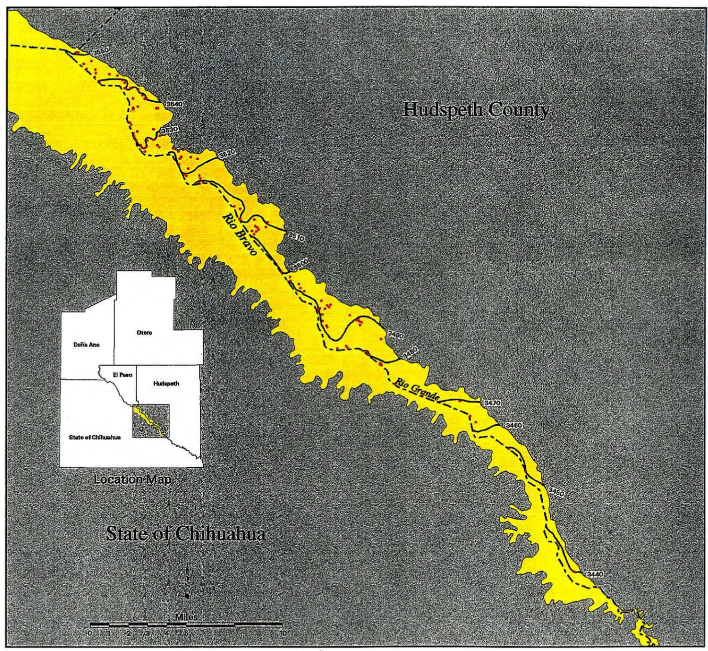
Figure 5.2. Water level contour map for the Rio Grande aquifer in El Paso and Hudspeth Counties, 1973 and 1974. Map illustrates losing stream, underflow, and baseflow conditions at different segments of the floodplain (source of data, Texas Water Development Board).
