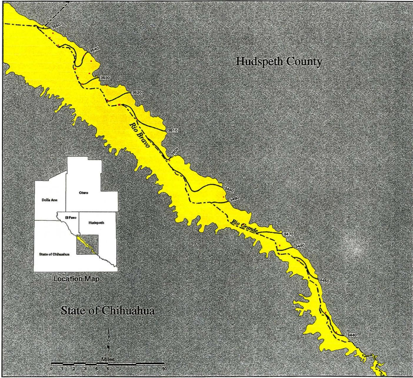
Figure 5.3. Water level contour map for the Rio Grande aquifer in El Paso and Hudspeth Counties, 1994 and 1995. A comparison of figures 5.2 and 5.3 indicates that drawdowns have intensified in the El Paso area since 1973 (see figure 5.1 for delineation of the El Paso area. Source of data, Texas Water Development Board).
