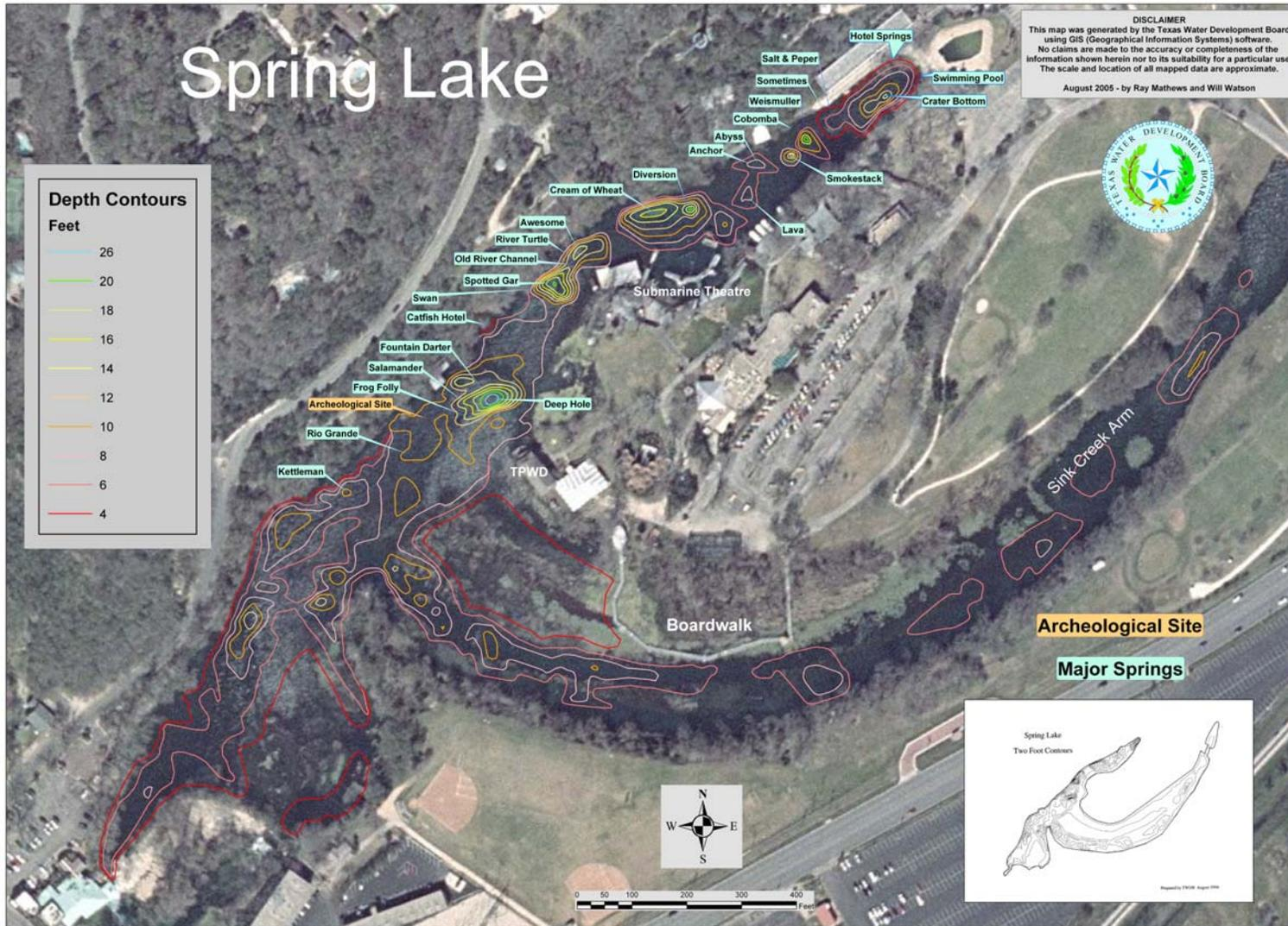
Figure 1. GPS-DOQ map of Spring Lake. Major springs and habitat features are shown with depth contours; based on hydrographic survey, depth and GPS measurements.
