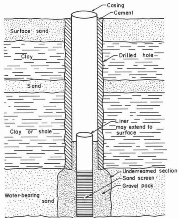
Figure 11.—Construction of a Typical Public-Supply Well
