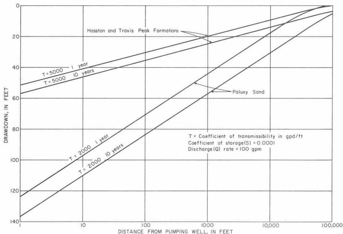
Figure 10.—Relation of Drawdown to Distance and Time in Pumped Aquifers
