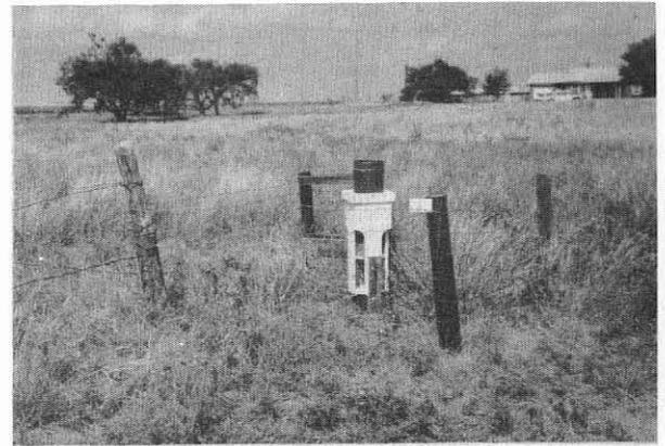
Typical non-recording rain gage installation. This is rain gage 19-S in study area. Photograph taken October 14, 1962.
