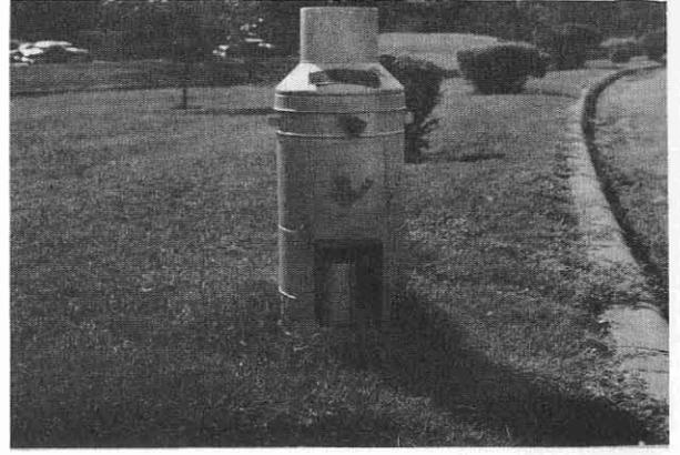
Typical recording rain gage. This photograph taken in Waller Creek watershed in Austin, Texas, October 16, 1962. Same type of recording rain gage is used in Mukewater Creek study area.
