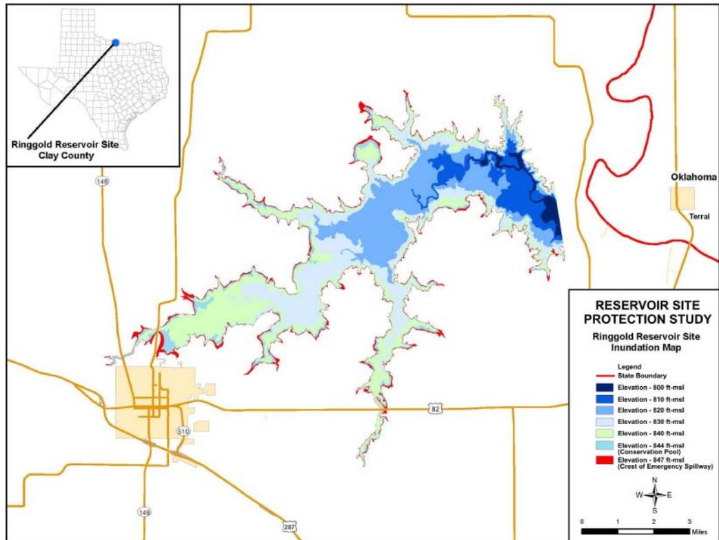
Figure 5-92. Inundation map for Ringgold Reservoir.
