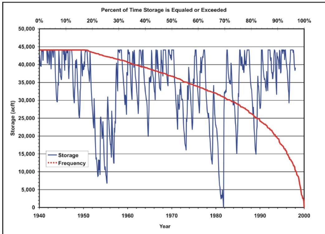
Figure 5-110. Simulated system storage for Lake Palo Pinto and Wilson Hollow reservoirs (system diversion=17,213 acre-feet per year).
