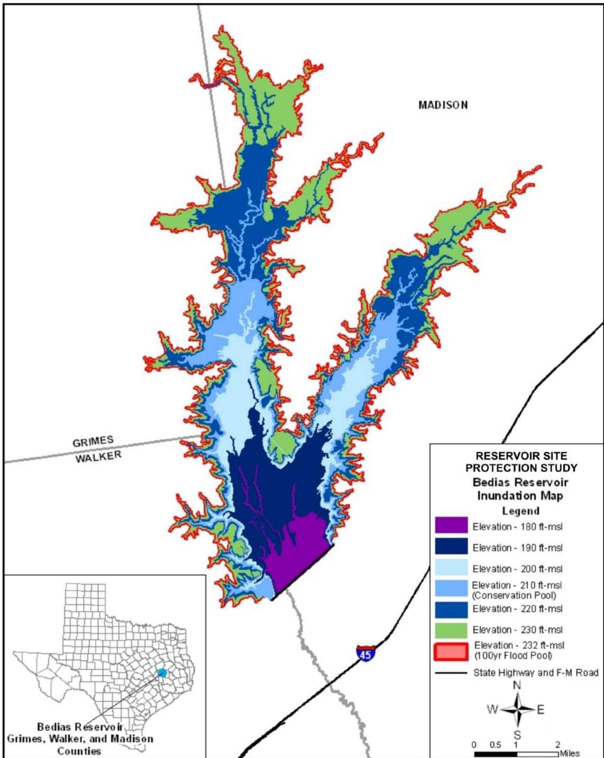
Figure 5-3. Inundation map for Bedia Reservoir.
