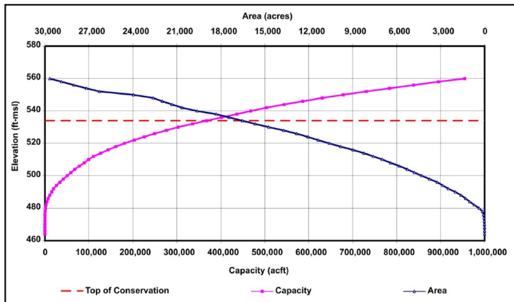
Figure 5-42. Elevation-area-capacity relationship for Lower Bois d'Arc Creek Reservoir. ft-msl=feet above mean sea level; acft=acre-feet
