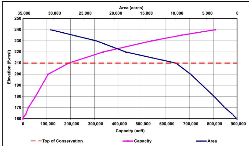
Figure 5-2. Elevation-area-capacity relationship for Bediais Reservoir. ft-msl=feet above mean sea level; acft=acre-feet
