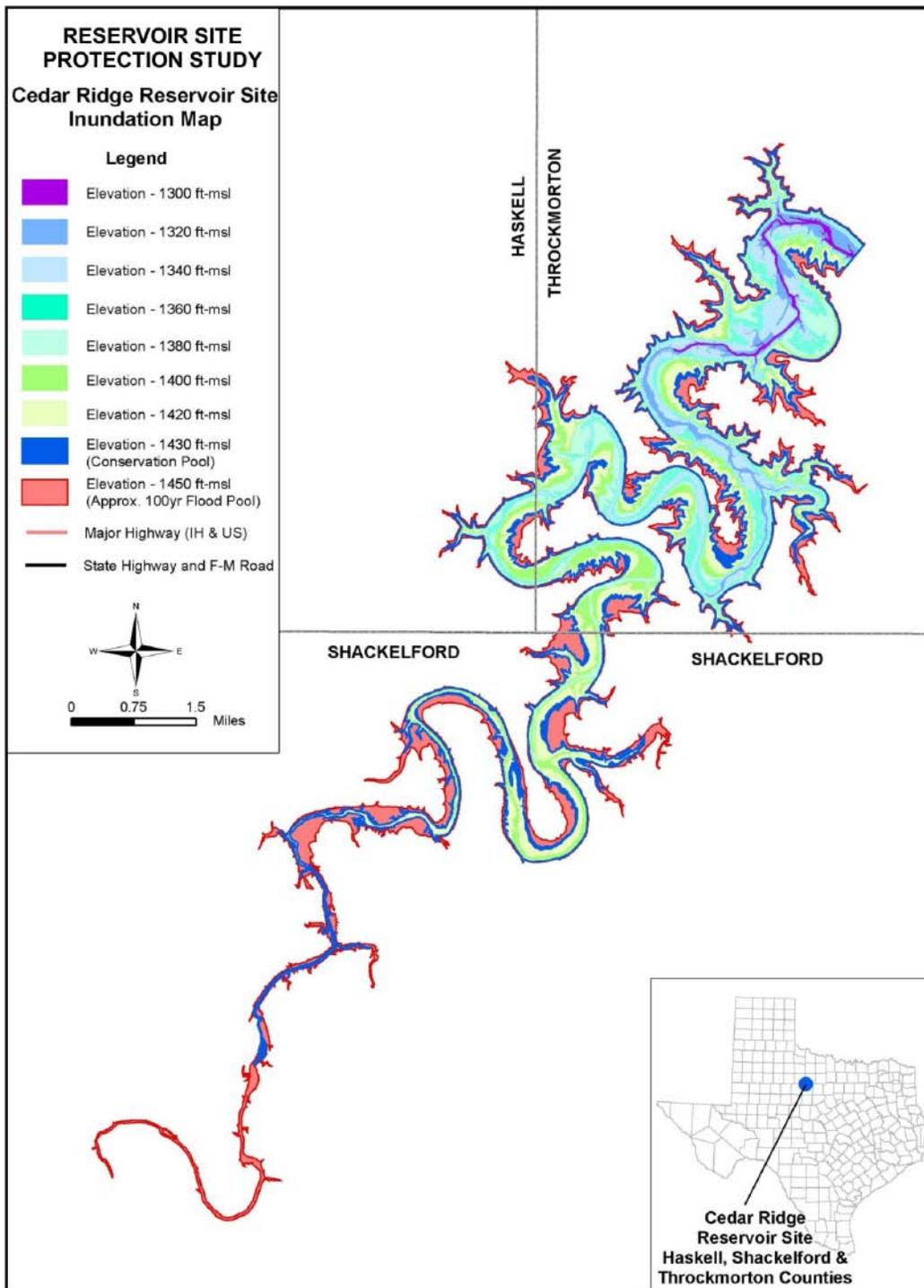
Figure 5-21. Inundation map for Cedar Ridge Reservoir.
