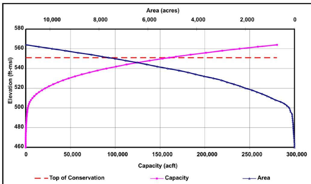
Figure 5-85. Elevation-area-capacity relationship for Lake Ralph Hall. ft-msl=feet above mean sea level; acft=acre-feet
