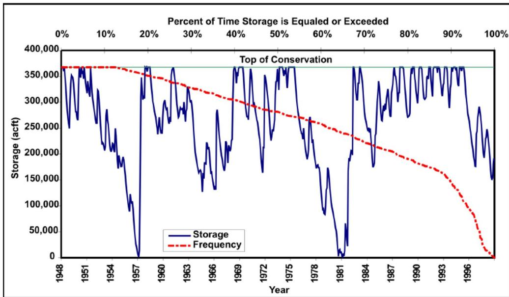
Figure 5-45. Simulated storage in Lower Bois d'Arc Creek Reservoir (conservation elevation=534 feet; diversion=126,280 acre-feet per year)
