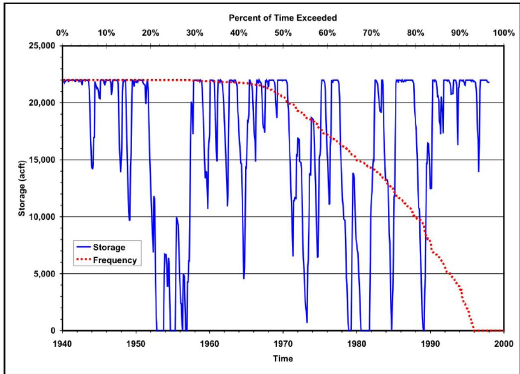
Figure 5-109. Simulated storage in Wilson Hollow Reservoir (conservation elevation=1,077 feet; incremental diversion=873 acre-feet per year).
