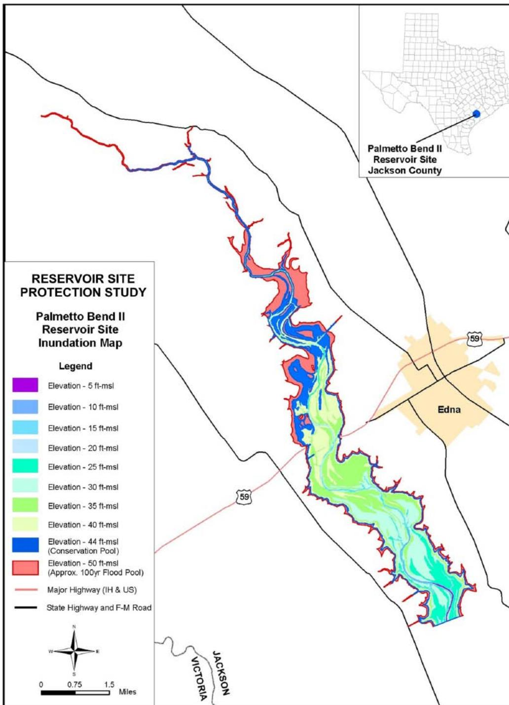
Figure 5-65. Inundation map for Palmetto Bend Reservoir—Stage II. ft-msl=feet above mean sea level
