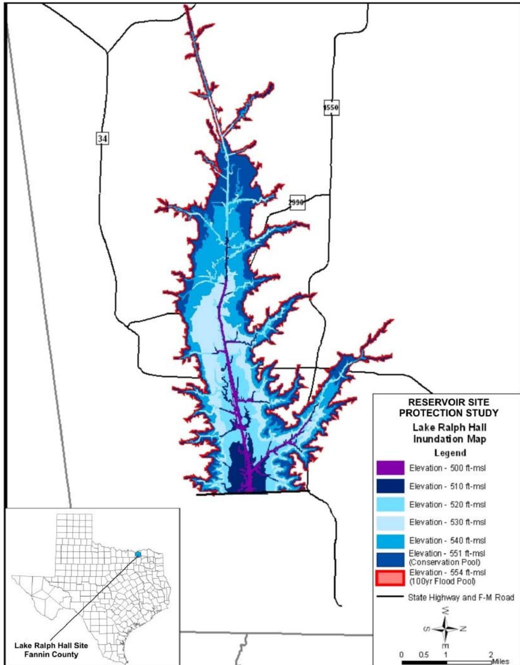
Figure 5-86. Inundation map for Lake Ralph Hall. ft-msl=feet above mean sea level
