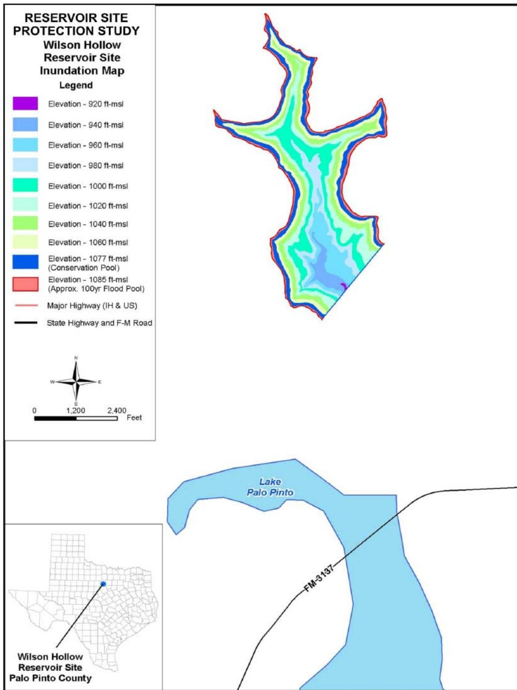
Figure 5-107. Inundation map for Wilson Hollow Reservoir.
