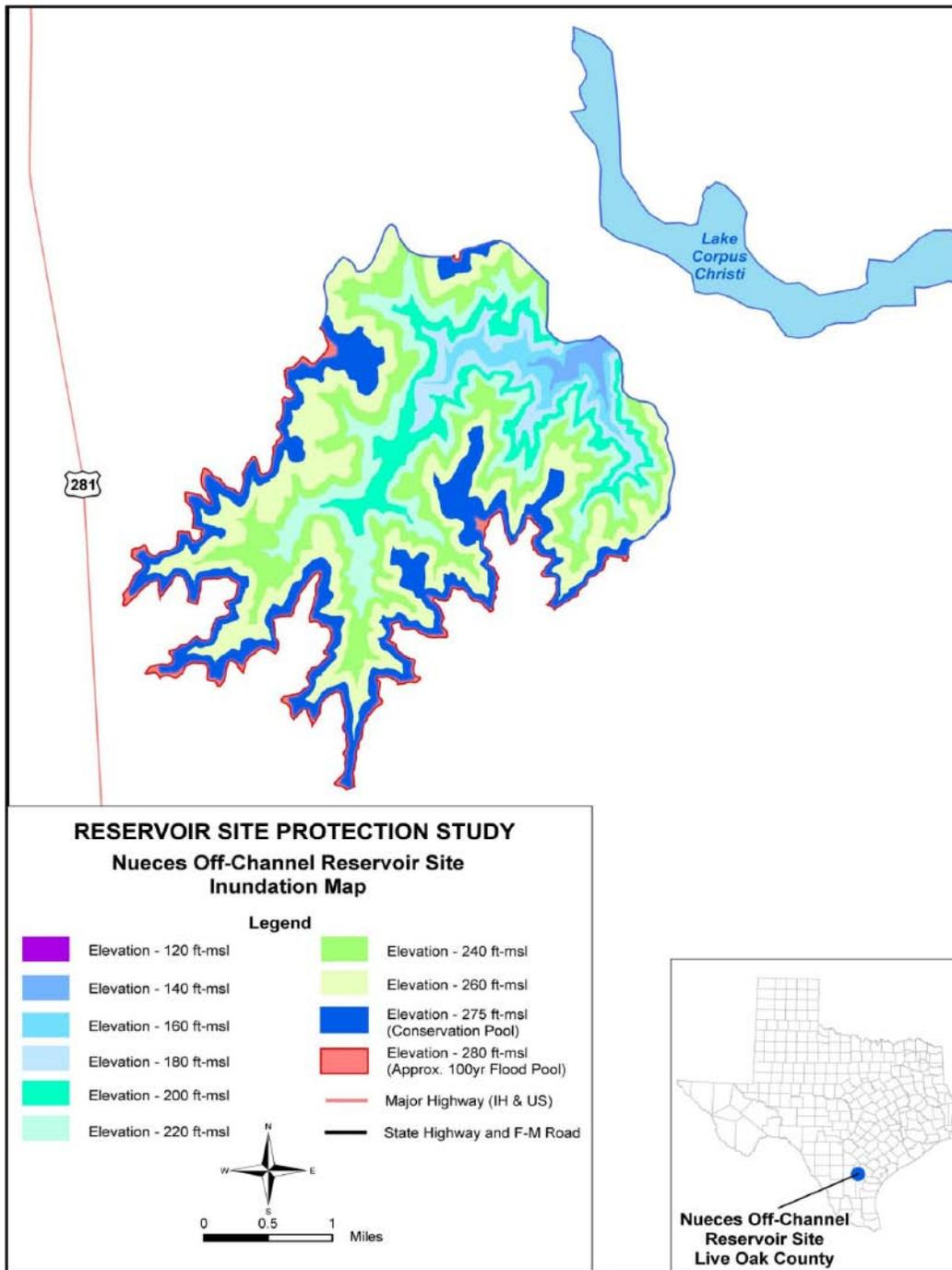
Figure 5-57. Inundation map for Nueces Off-Channel Reservoir. ft-msl=feet above mean sea level
