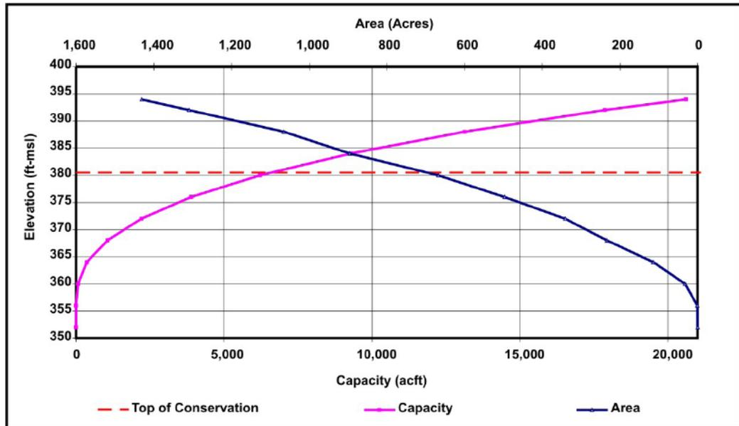
Figure 5-14. Elevation-area-capacity relationship for Brushy Creek Reservoir.
