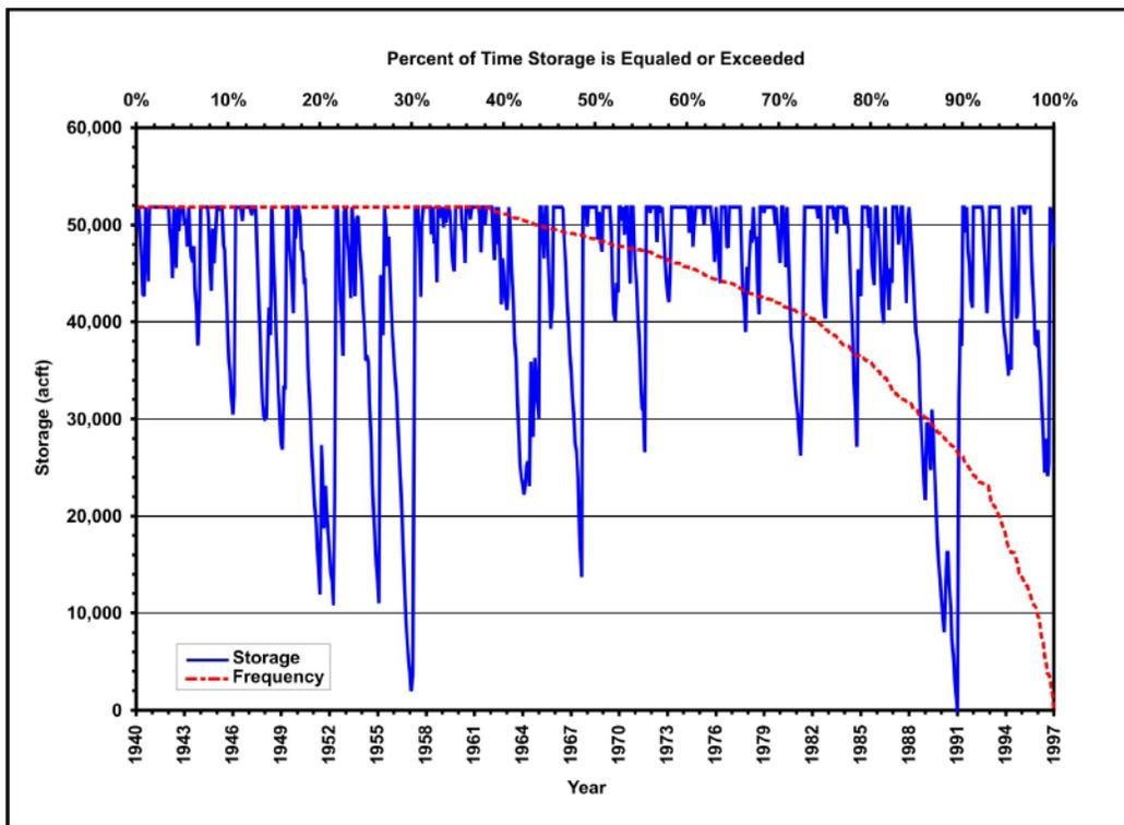
Figure 5-67. Simulated storage in Palmetto Bend Reservoir–Stage II (conservation elevation=44 feet; diversion=2,964 acre-feet per year). acft=acre-feet
