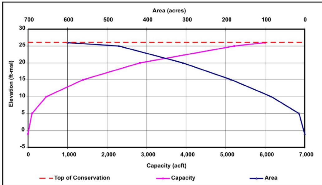
Figure 5-9. Elevation-area-capacity relationship for Brownsville Weir and Reservoir. ft-msl=feet above mean sea level; acft=acre-feet
