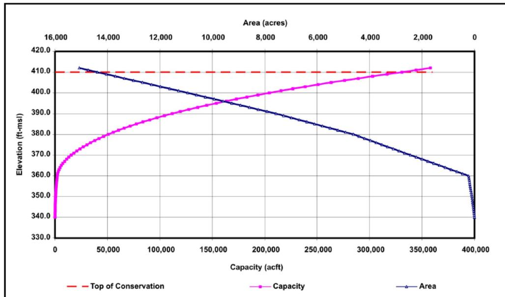
Figure 5-78. Elevation-area-capacity relationship for Parkhouse II Lake. ft-msl=feet above mean sea level; acft=acre-feet
