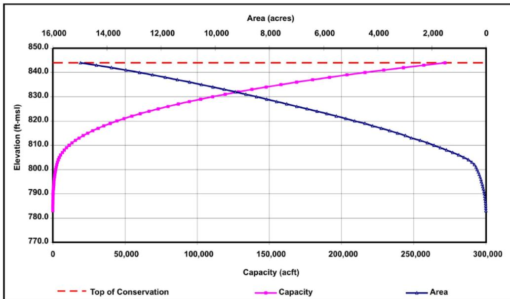
Figure 5-91. Elevation-area-capacity relationship for Ringgold Reservoir. ft-msl=feet above mean sea level; acft=acre feet
