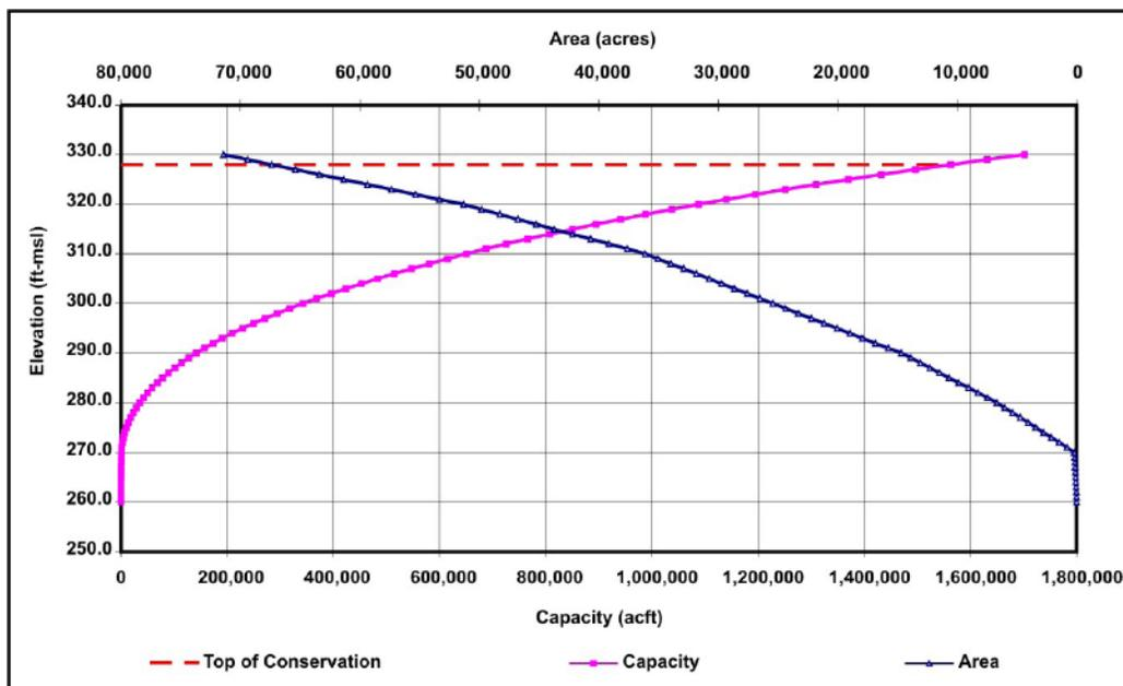
Figure 5-49. Elevation-area-capacity relationship for Marvin Nichols IA Reservoir. ft-msl=feet above mean sea level; acft=acre-feet
