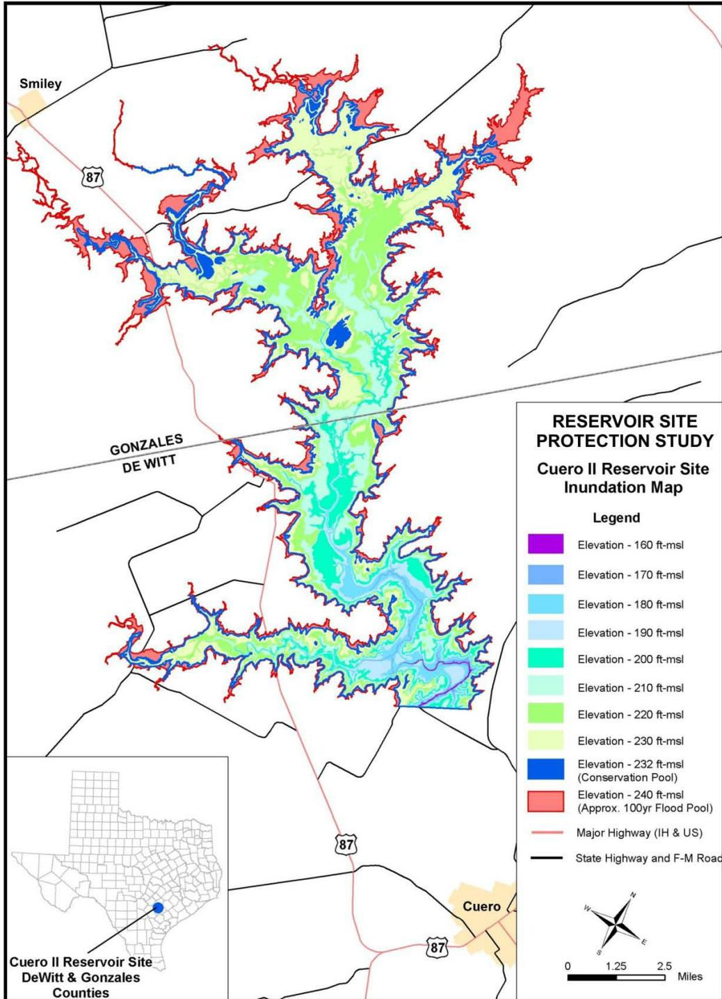
Figure 5-28. Inundation map for Cuero II Reservoir. ft-msl=feet above mean sea level
