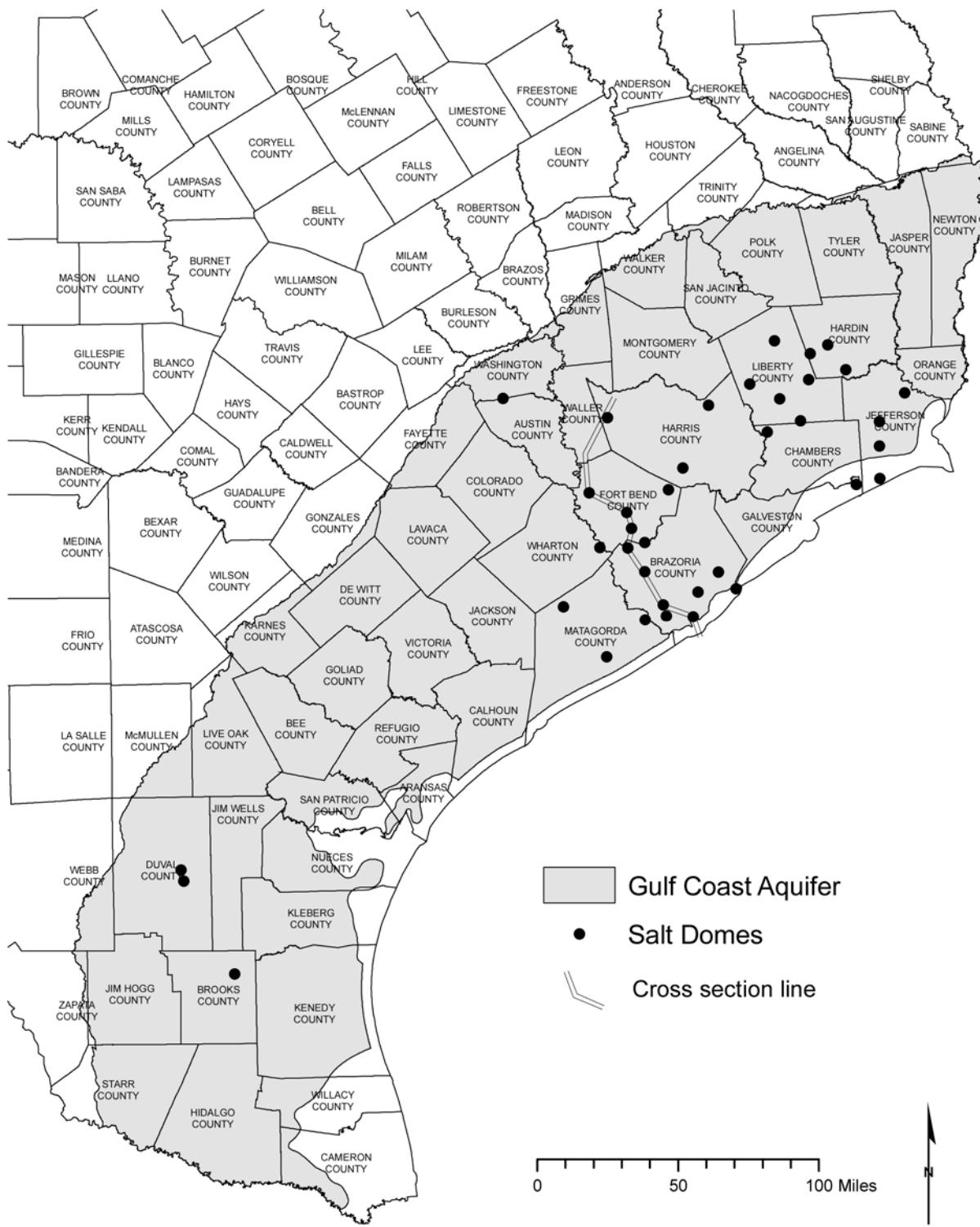
**Figure 12-3. Map of shallow salt domes in the Gulf Coast aquifer in Texas. Also showing line of cross section in Figure 12-2 (compiled from Seni and others, 1984b-d, 1985).**
