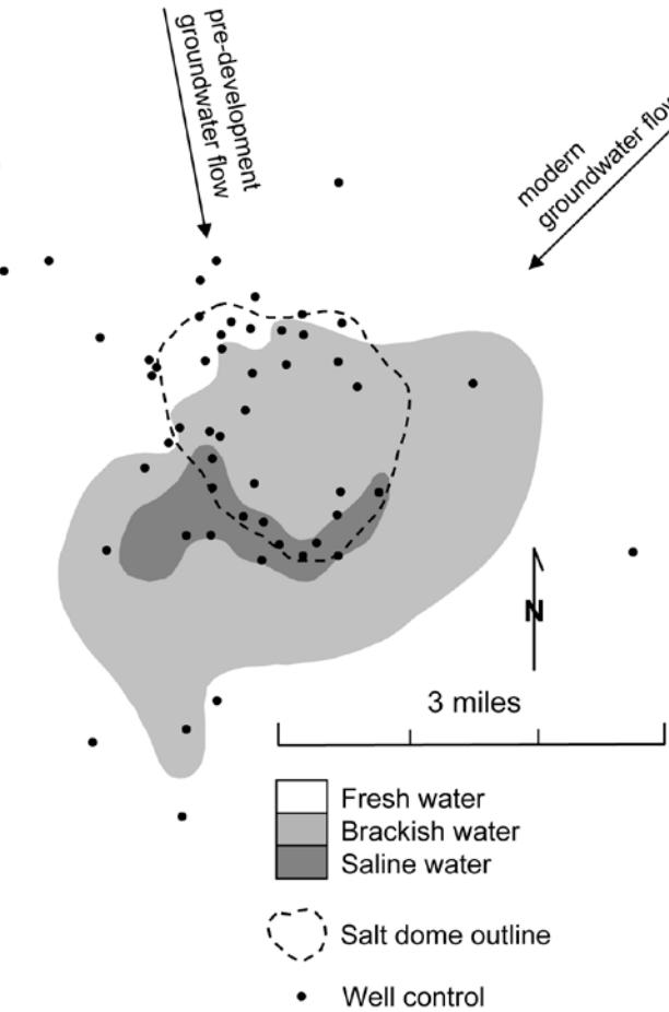
**Figure 12-8.** Map of groundwater salinity in a lower Chicot sand at Barbers Hill salt dome. Salinities were measured in water wells and calculated from geophysical logs. Anomalously high salinities on the southwest side of the dome outline a plume of saline water extending away from the salt dome in the down-flow direction (modified from Hamlin and others, 1988).
