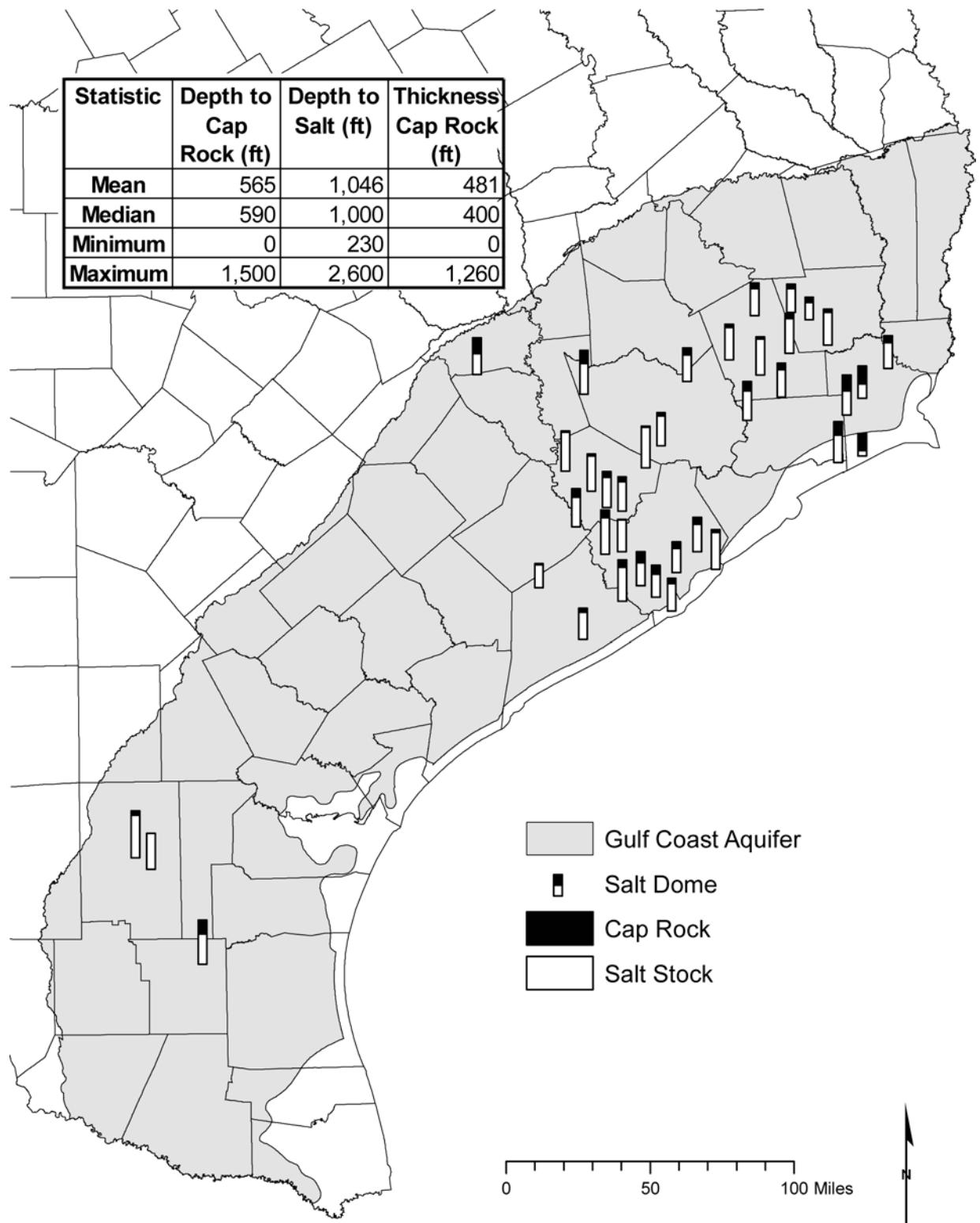
Figure 12-4. Map of shallow salt domes in the Gulf Coast aquifer showing relative depths and cap rock thicknesses. The salt domes are shown schematically extending above a datum at 3,000 feet below sea level. Depth and thickness statistics also shown (Compiled from Beckman and Williamson, 1990, and Seni and others, 1984b-d, 1985).
