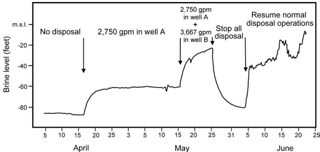
**Figure 12-6.** Hydrograph of a long-term cap rock injection test at Barbers Hill salt dome showing brine-level changes in a cap rock observation well during controlled brine disposal in two other cap rock wells. Water levels in nearby Chicot and Evangeline wells are around 100 feet below sea level or similar to cap rock brine levels when no disposal is occurring (modified from Hamlin and others, 1988).
