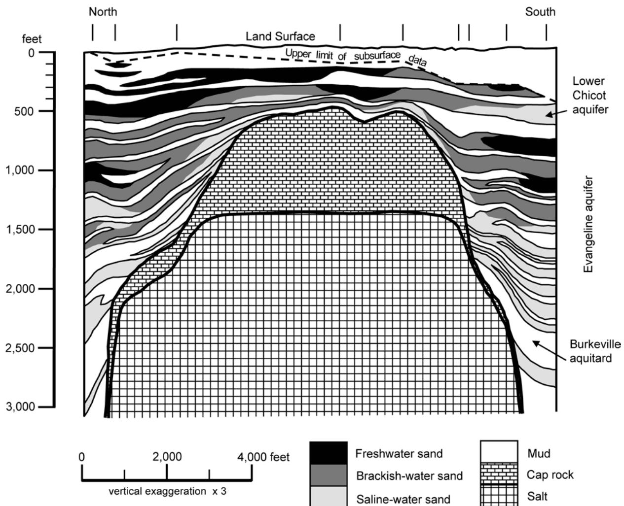
**Figure 12-7.** North-south cross section across Barbers Hill salt dome showing Chicot and Evangeline sands and groundwater salinities near and in contact with the cap rock. Groundwater salinities were interpreted from geophysical logs. Individual sand bodies were correlated and mapped using closely spaced geophysical and drillers logs. A map of salinity in the lower Chicot sand is shown in Figure 12-8 (modified from Hamlin and others, 1988).
