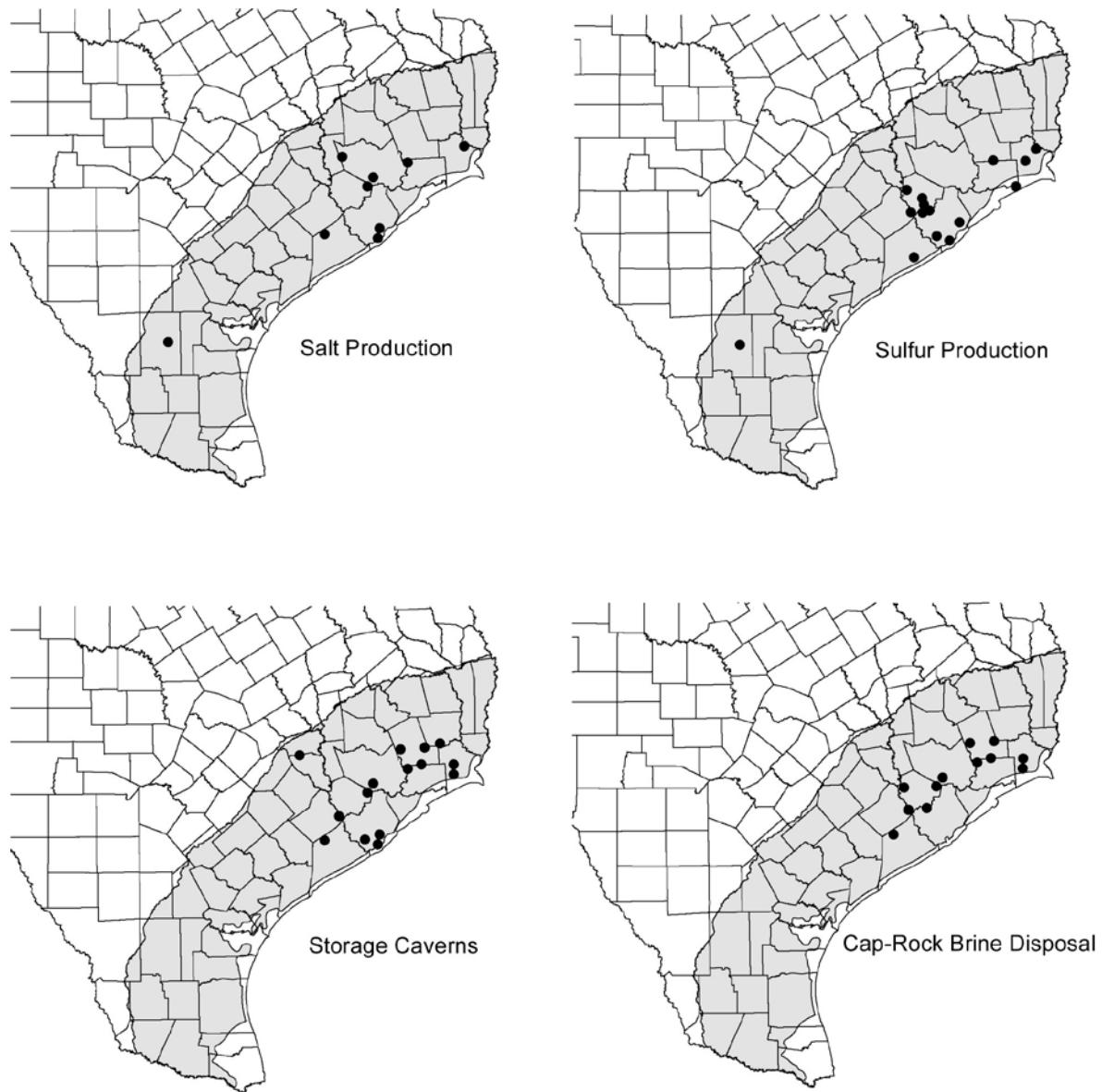
**Figure 12-5.** Maps of shallow salt domes in the Gulf Coast aquifer showing natural resources. Petroleum resources (not shown) have been developed at most Gulf Coast salt domes (compiled from Seni and others, 1984b-d, 1985).
