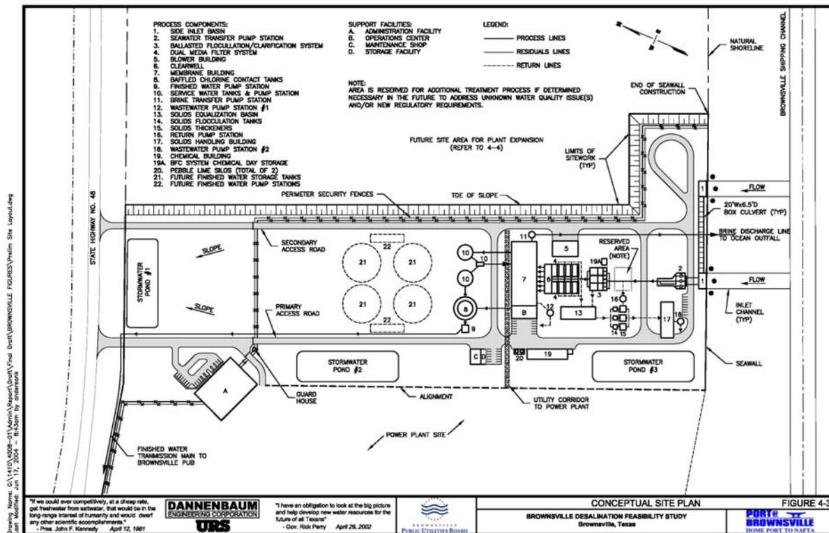
**Finished Water Transmission:** The finished water transmission main will leave the pump station located at the treatment plant site and cross State Highway 48 (SH 48) to the north. It will then parallel SH 48 and run westerly to the proposed offsite storage near FM 511. From this point, the finished water will be pumped into the Brownsville system and in future phases, to other municipalities.
