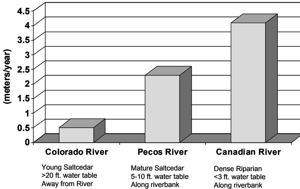
Figure 16-6: Evapotranspirational water loss from areas infested with saltcedar and associated plants on three major rivers in Texas, from 2000 well data (Hays, 2003).
