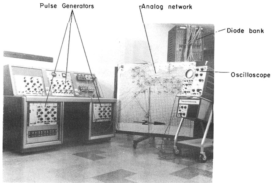
**A. Electronic equipment used to excite element**
