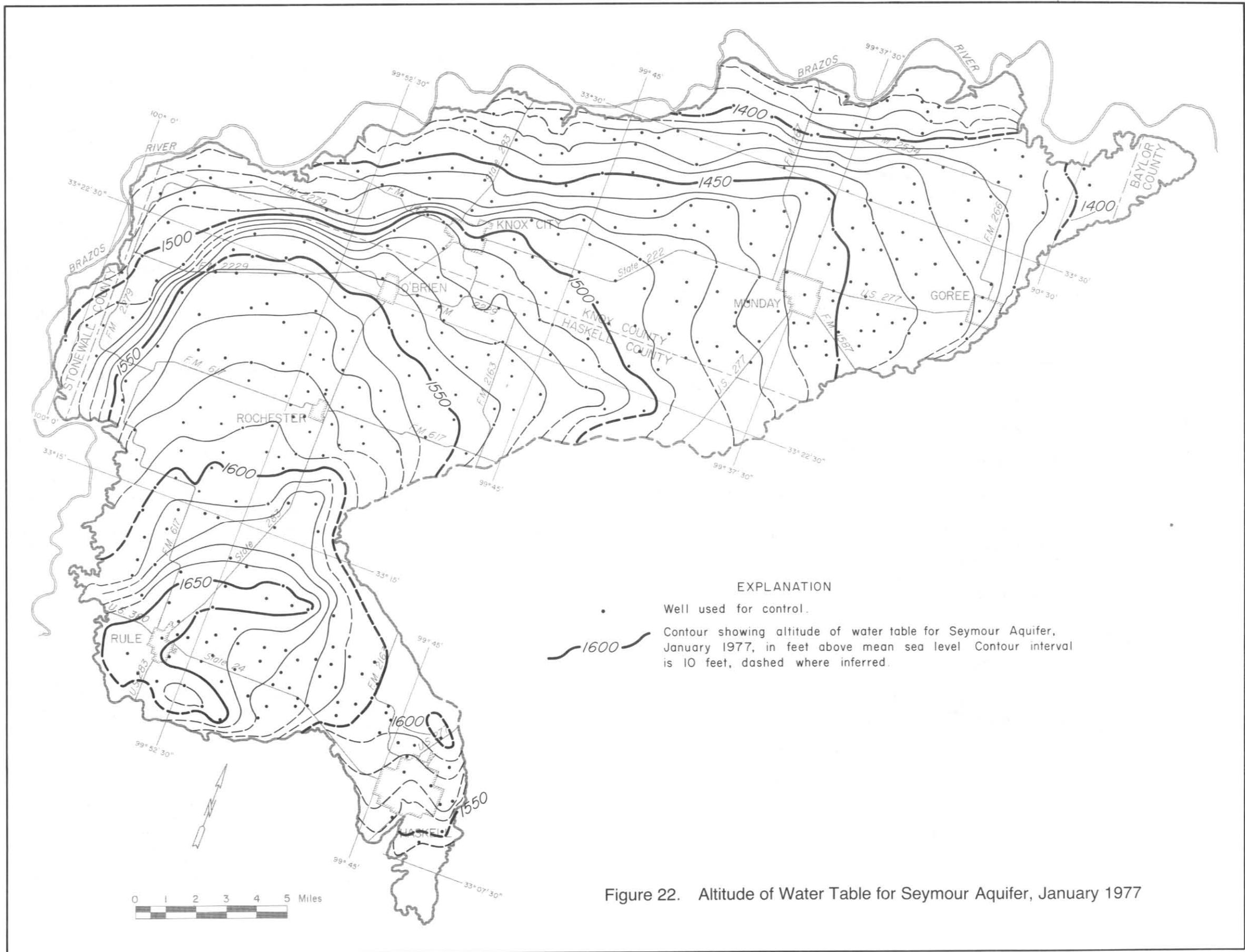
Figure 22. Altitude of Water Table for Seymour Aquifer, January 1977
