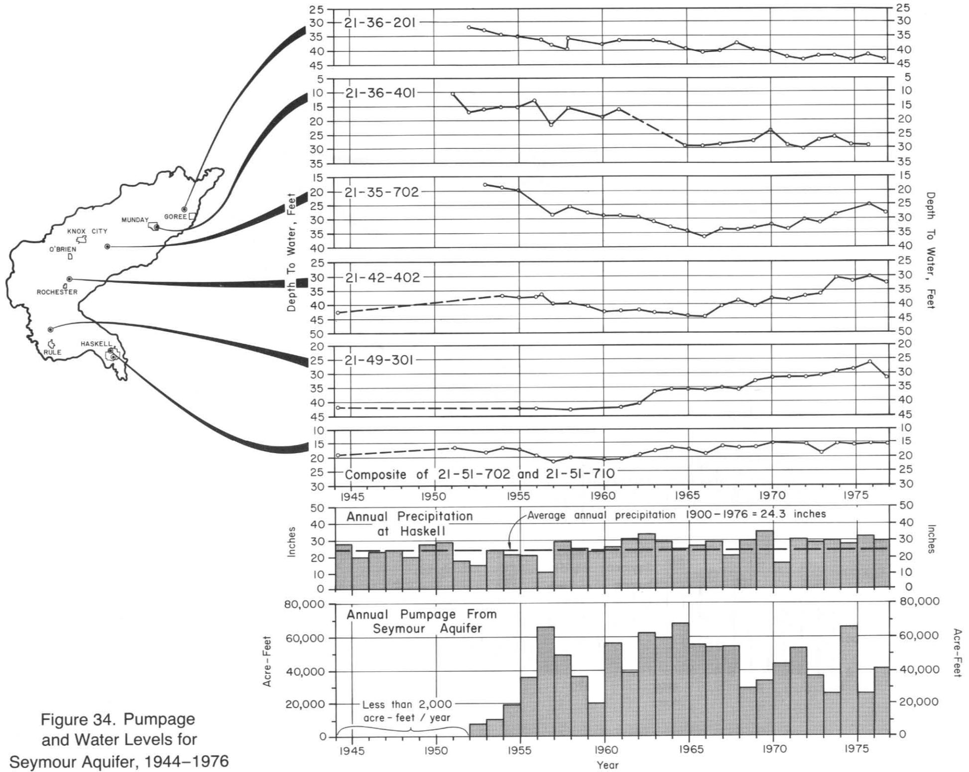
Figure 34. Pumpage and Water Levels for Seymour Aquifer, 1944-1976
