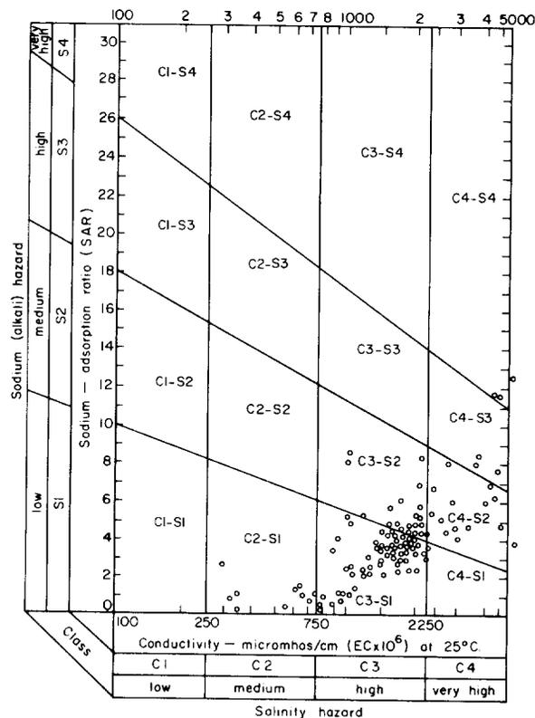
Figure 12.—Classification of Quaternary Alluvium Waters for Irrigation
