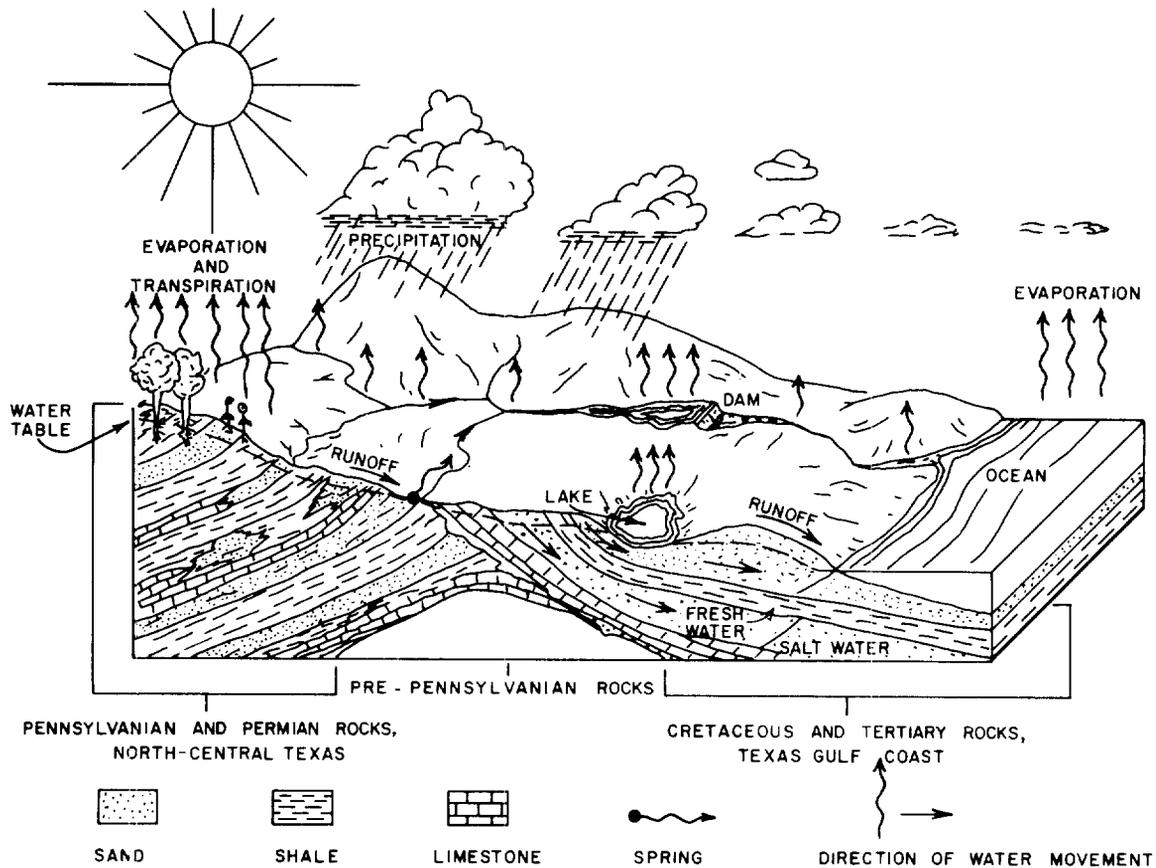
Figure 7.—Hydrologic Cycle
