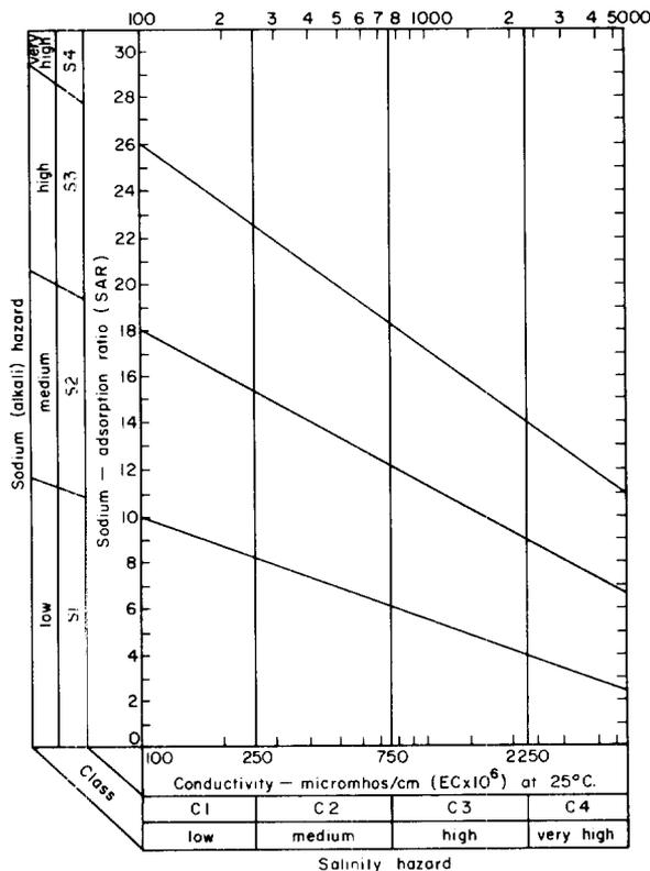
Figure 10.—Diagram for the Classification of Irrigation Waters (After U.S. Salinity Laboratory Staff, 1954, p. 80)
