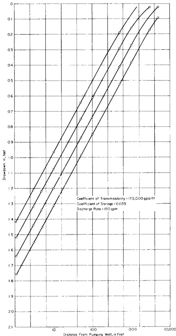
**Figure 13.—Diagram Showing Relation of Decline in Water Levels to Time and Distance as a Result of Pumping From the Alluvium Along Jim Ned Creek**
