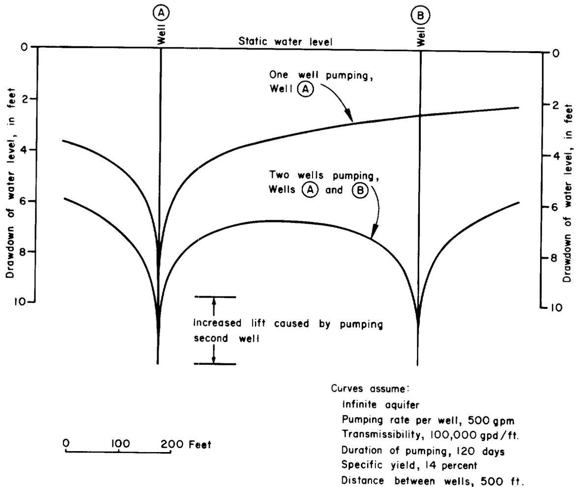
Figure 8.—Idealized Cross Section Showing Drawdown Interference Between Two Pumping Wells
