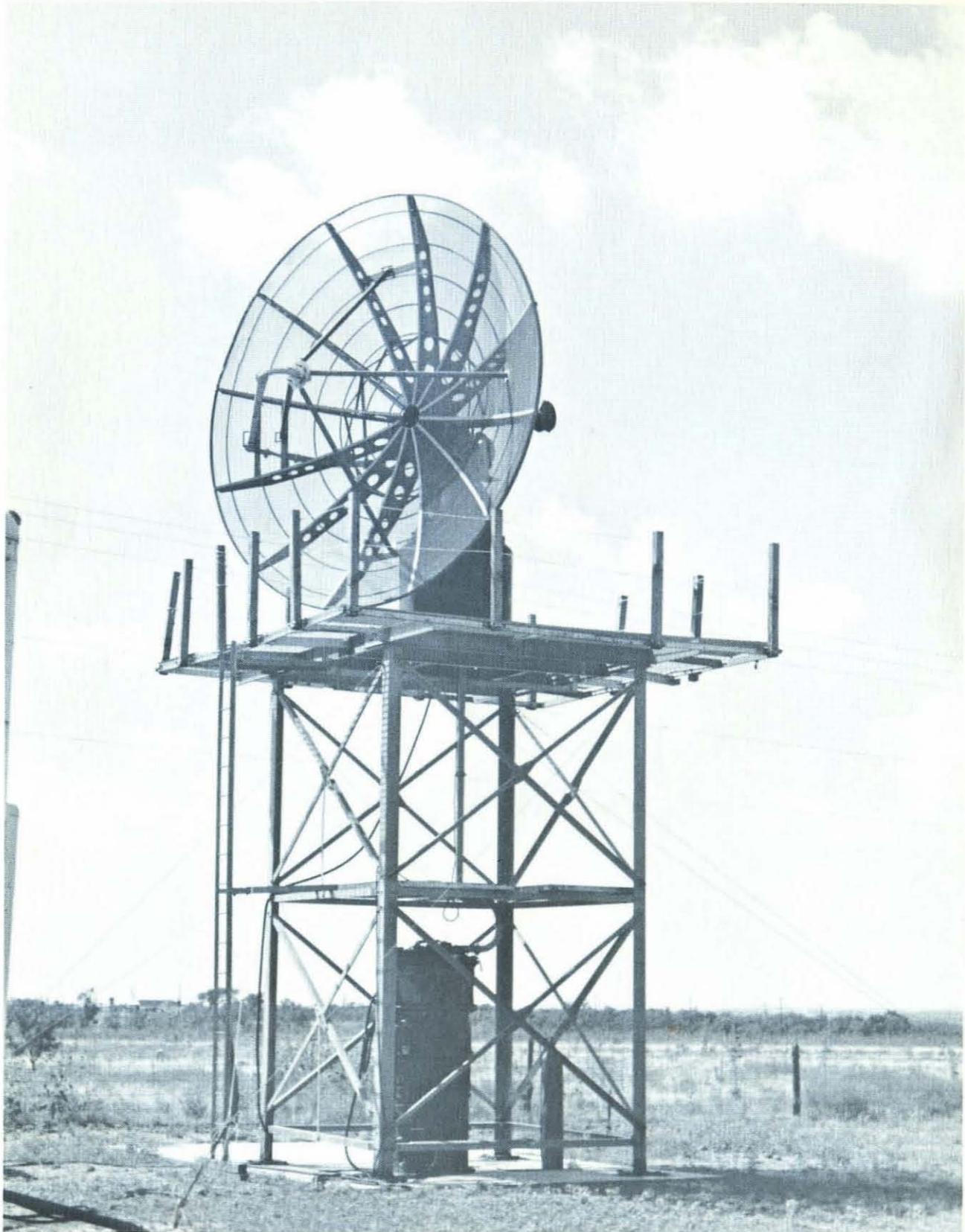
M-33 radar dish. This 15-foot parabolic dish antenna was used in the San Angelo Cumulus project to collect cloud physics data and obtain rainfall rate measurements. The radar system was later moved to Snyder to evaluate an operational cloud seeding project.
