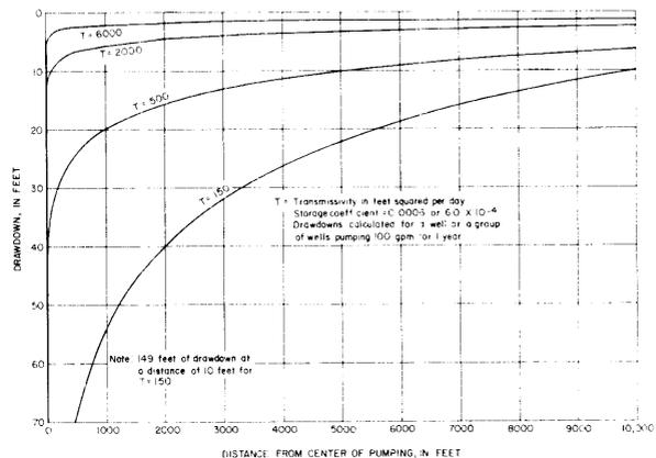
Figure 15.—Relation of Drawdown in an Artesian Aquifer to Transmissivity and Distance
