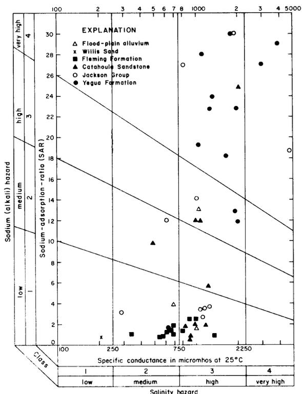
Figure 19.—Classification of Irrigation Waters
