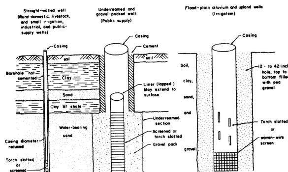
Figure 17.—Typical Construction of Rural-Domestic, Livestock, Public-Supply, Industrial, and Irrigation Wells
