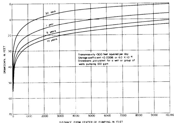
Figure 16.—Relation of Drawdown in an Artesian Aquifer to Time and Distance
