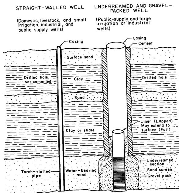
Figure 17.—Typical Construction of Domestic, Livestock, Public Supply, Industrial, and Irrigation Wells
