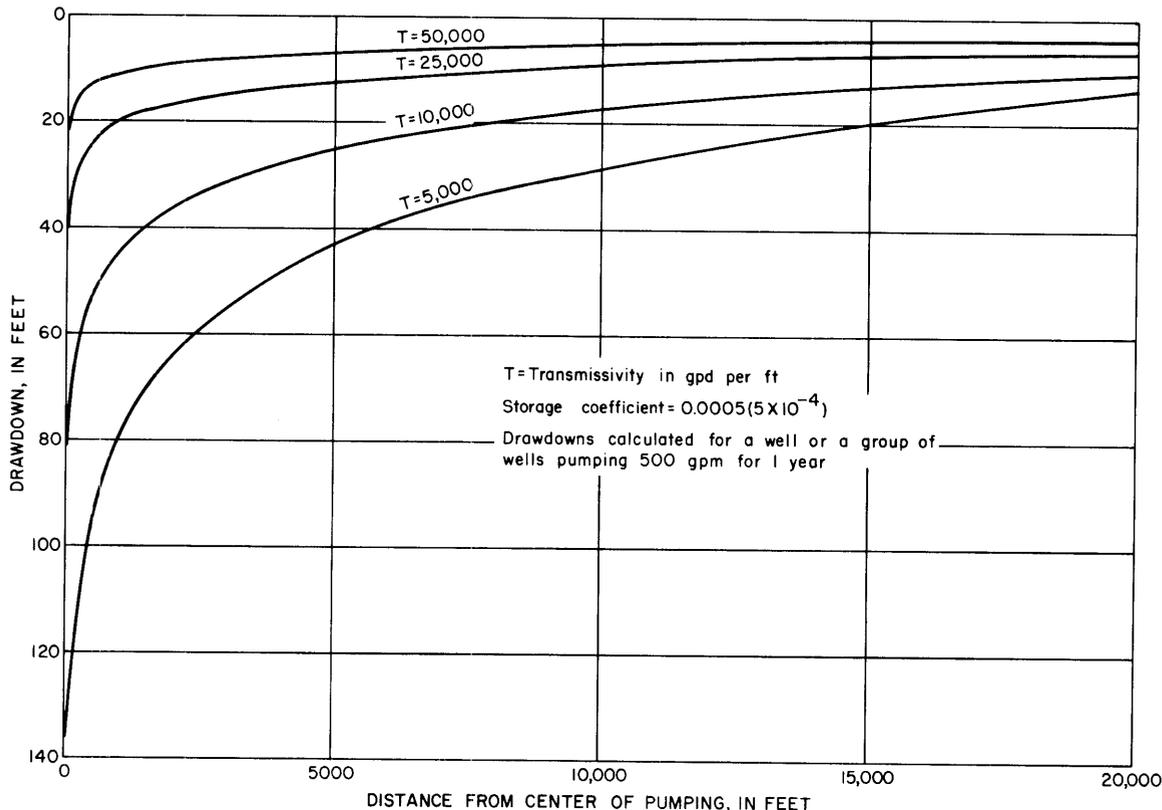
Figure 14.—Relation of Drawdown to Transmissivity and Distance
