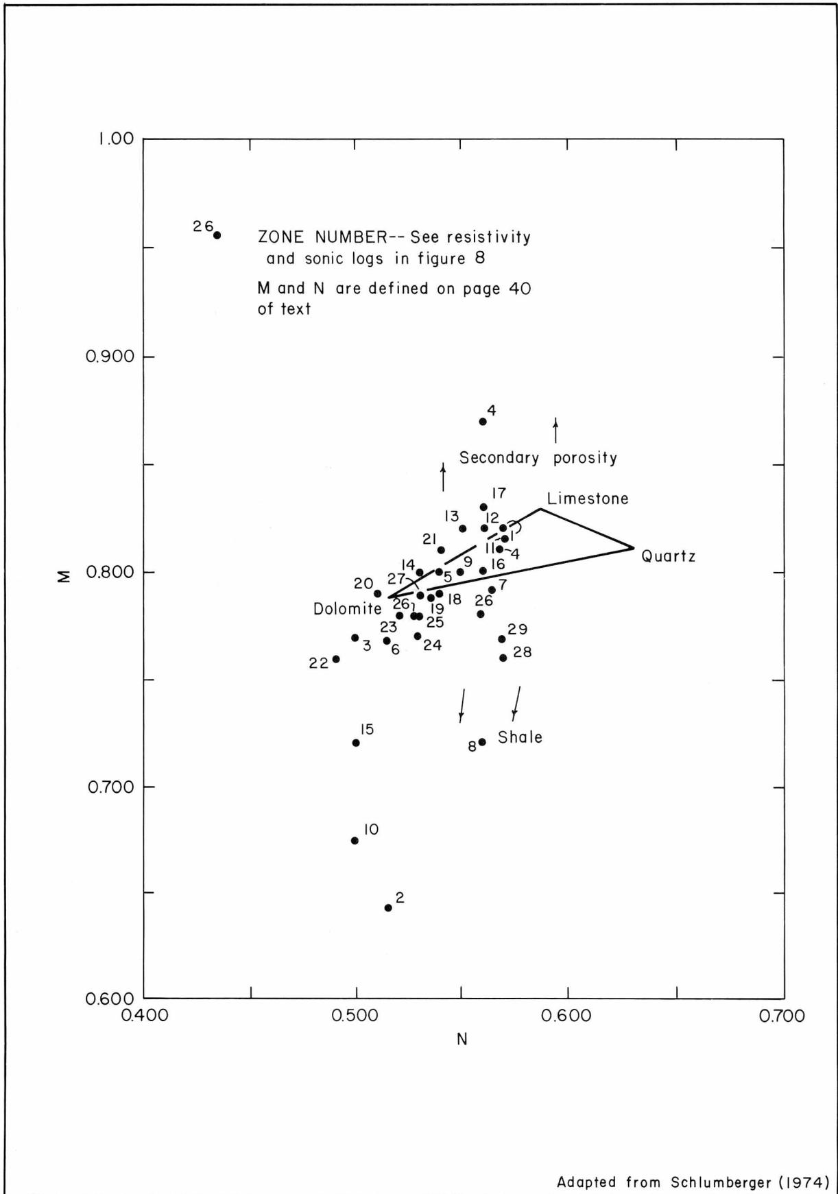
FIGURE 14.-M-N cross plot of distributed zones in the San Marcos test hole (LR-67-09-110)
