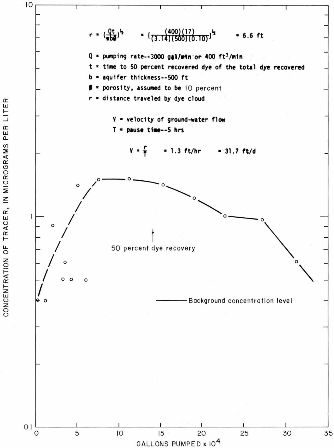
FIGURE 25.-Single-well pulse test in well AY-68-36-102
