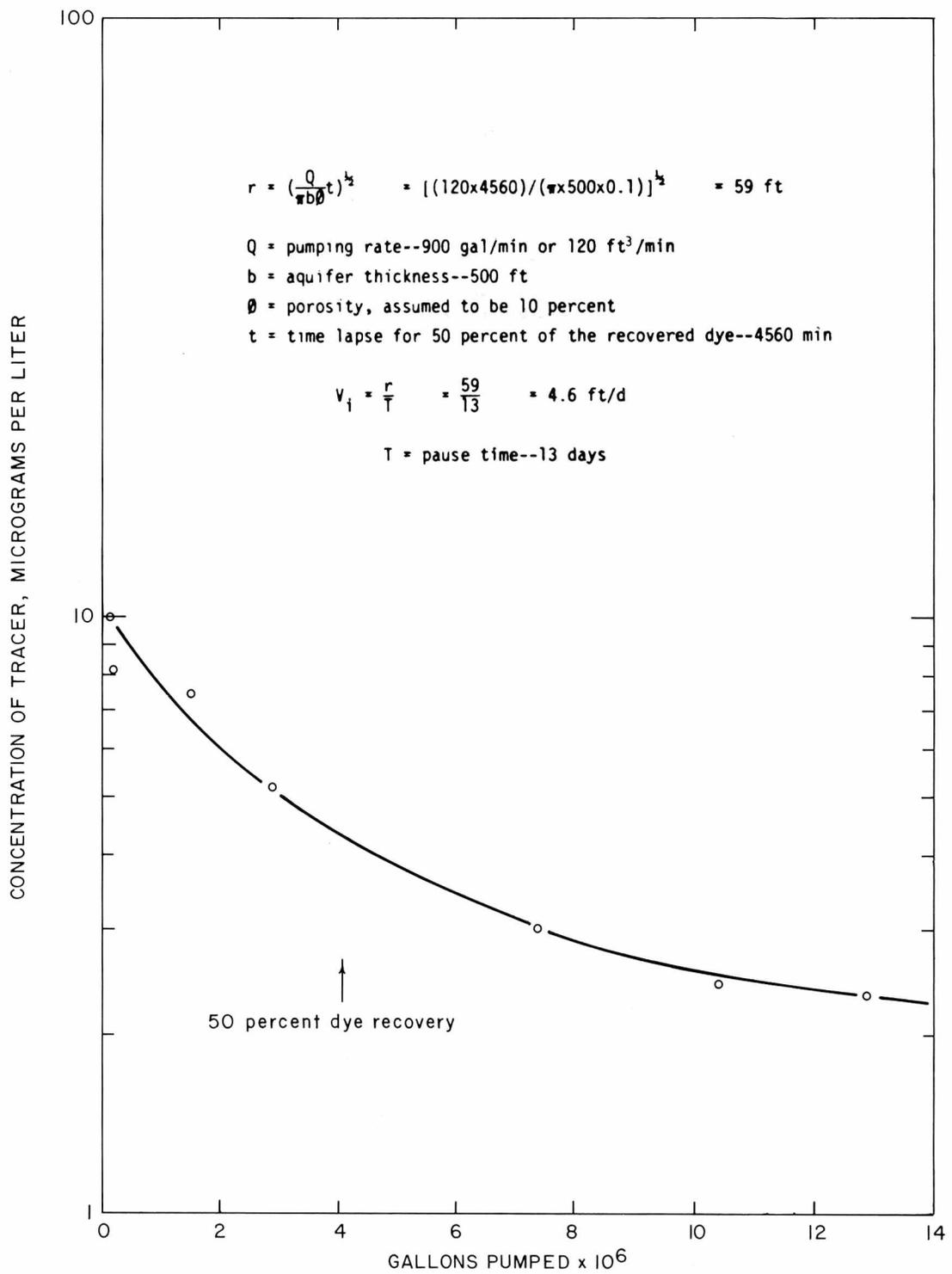
FIGURE 27.--Single-well pulse test in well AY-68-30-107
