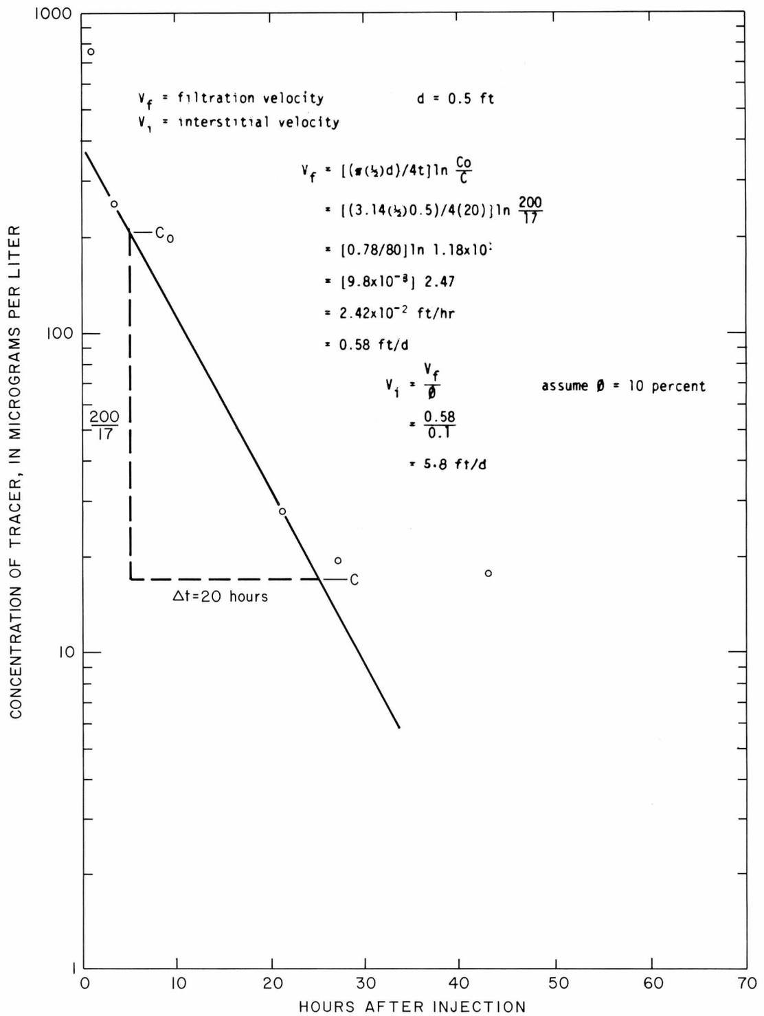
FIGURE 23.-Tracer-dilution test in well AY-68-27-5
