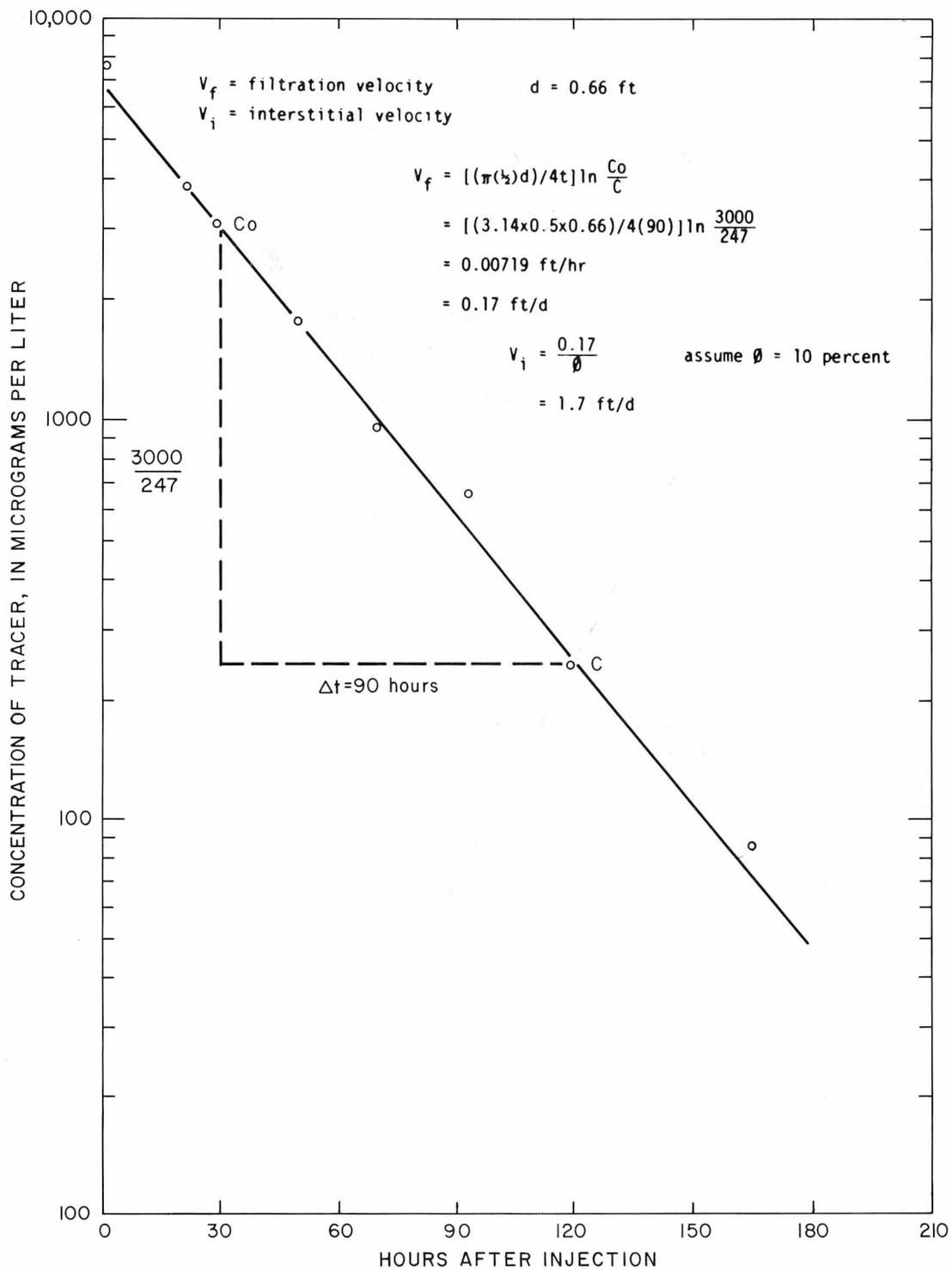
FIGURE 24.-Tracer-dilution test in well AY-68-29-103
