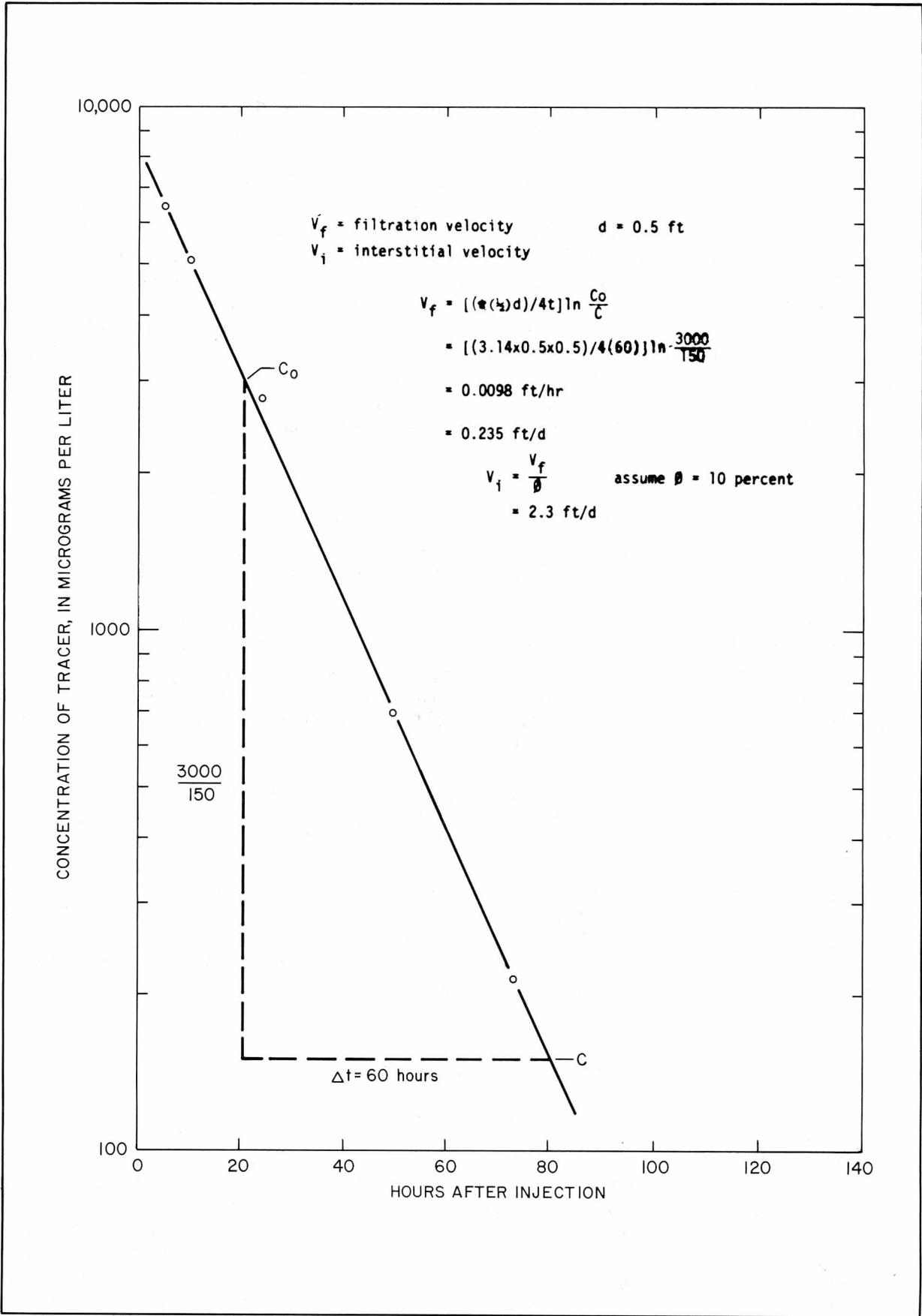
FIGURE 20.-Tracer-dilution test in well AY-68-27-505
