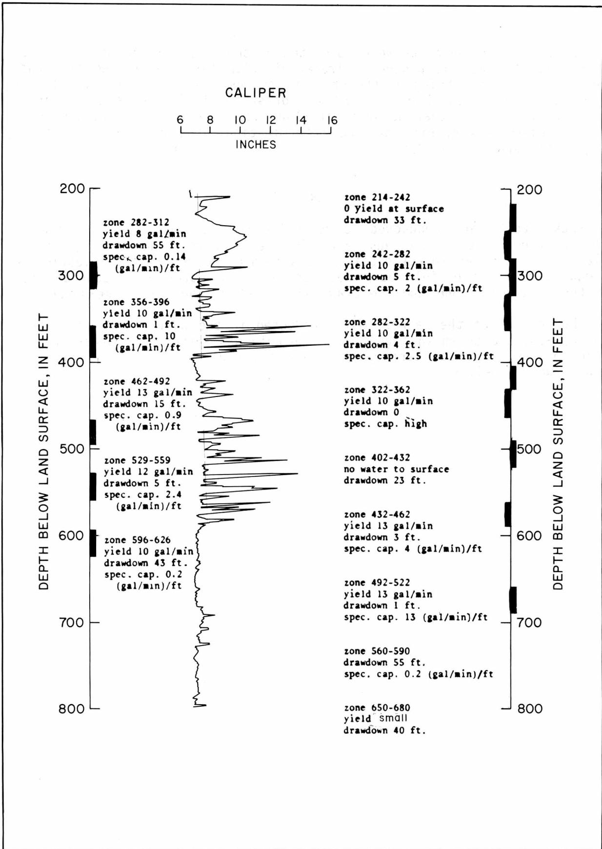
FIGURE 30.-Log showing packer test in the Castle Hills test hole (AY-68-28-910)
