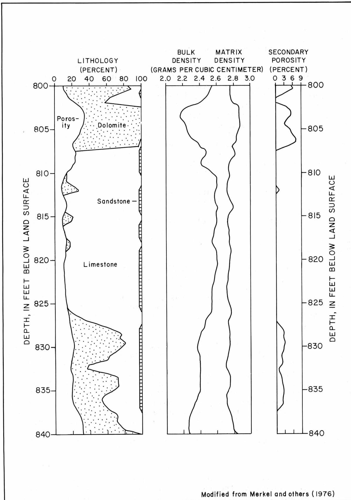
FIGURE 17.-Computer-processed interpretation of an interval in the Randolph test hole (AY-68-30-807)
