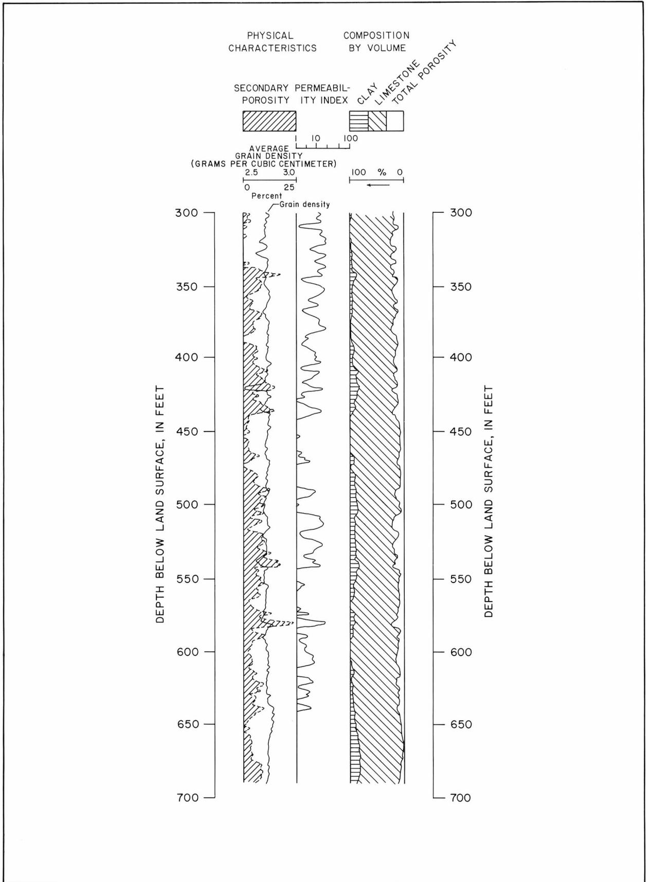
FIGURE 18.-Calculated total porosity, secondary porosity, grain density, and mineralogy for the Sabinal test hole (YP-69-37-402)
