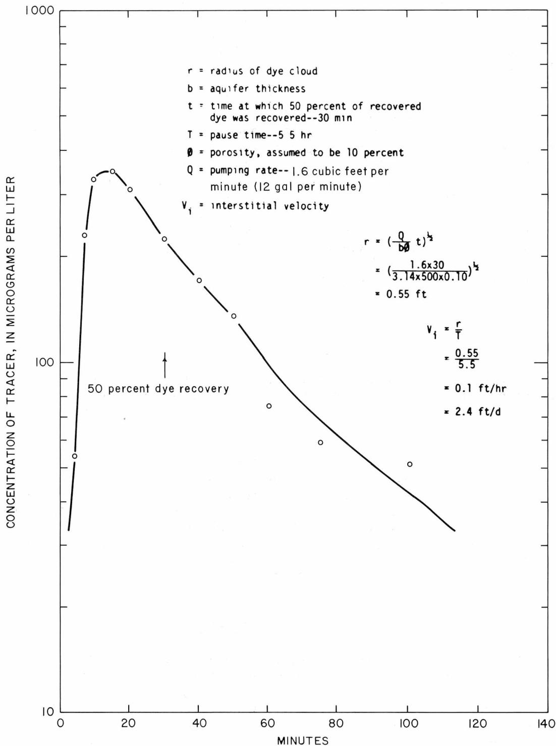
FIGURE 26.-Single-well pulse test in well AY-68-28-801
