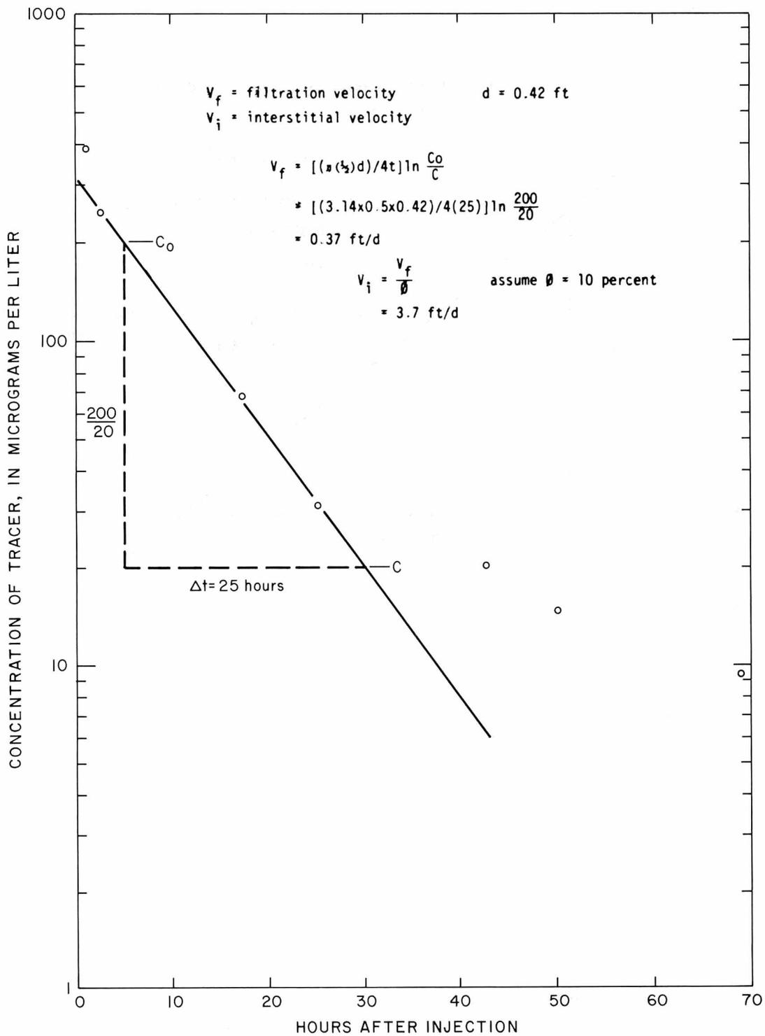
FIGURE 22.-Tracer-dilution test in well AY-68-28-801
