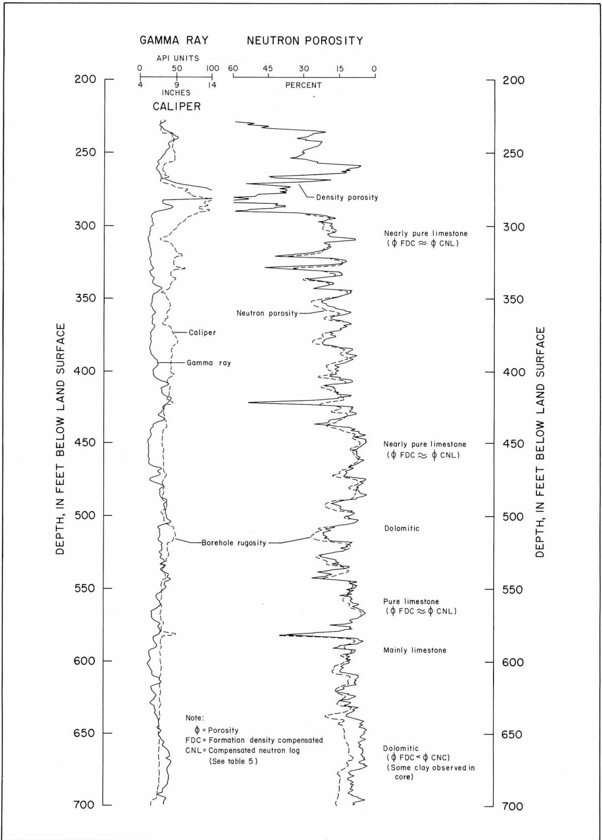
FIGURE 16.-Overlay of porosity logs calculated from density and neutron measurements in the Sabinal test hole (YP-69-37-402)
