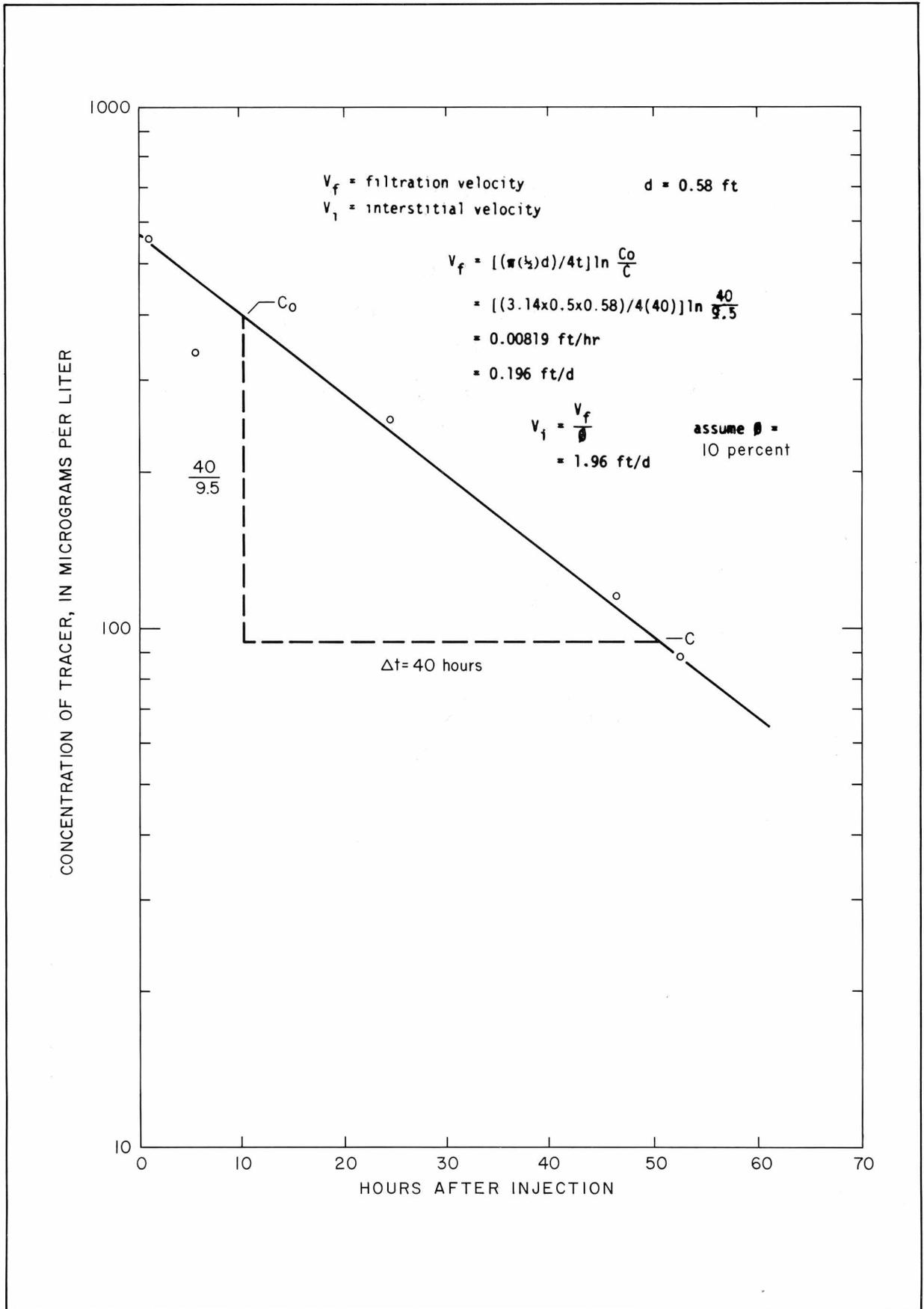
FIGURE 21.-Tracer-dilution test in well AY-68-28-102
