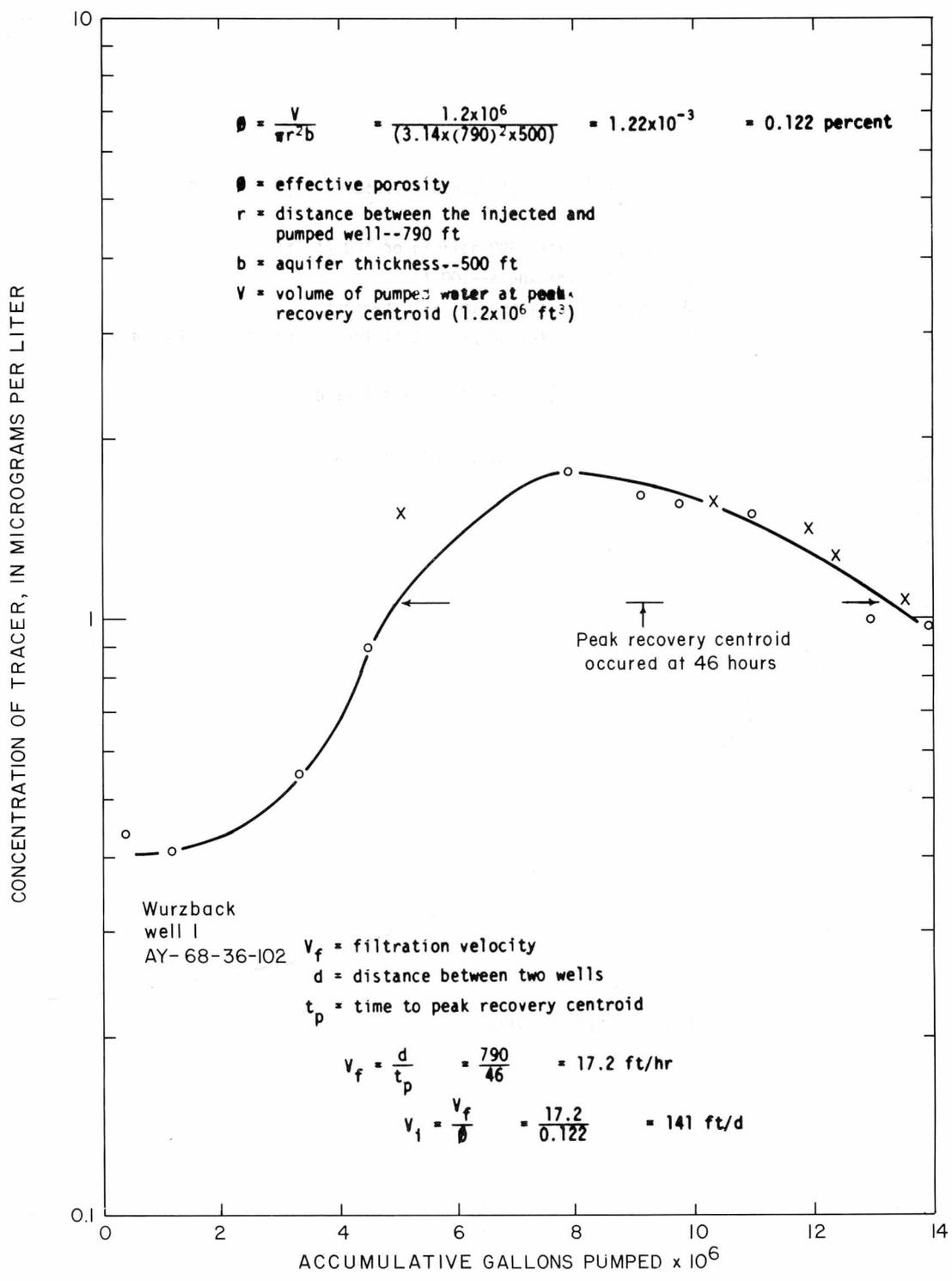
FIGURE 28.-Transit-time test of tracer between two wells at Wurzback station
