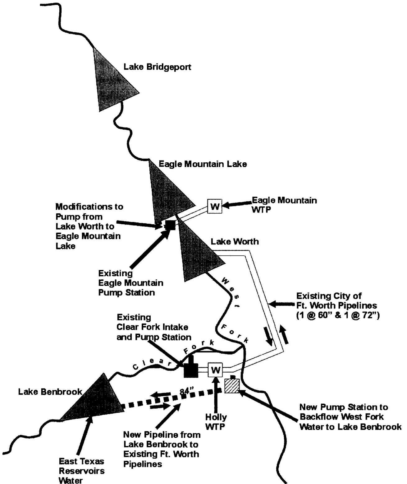
Figure 3-2. Enhancement of West Fork Water Supply (Option 1)
