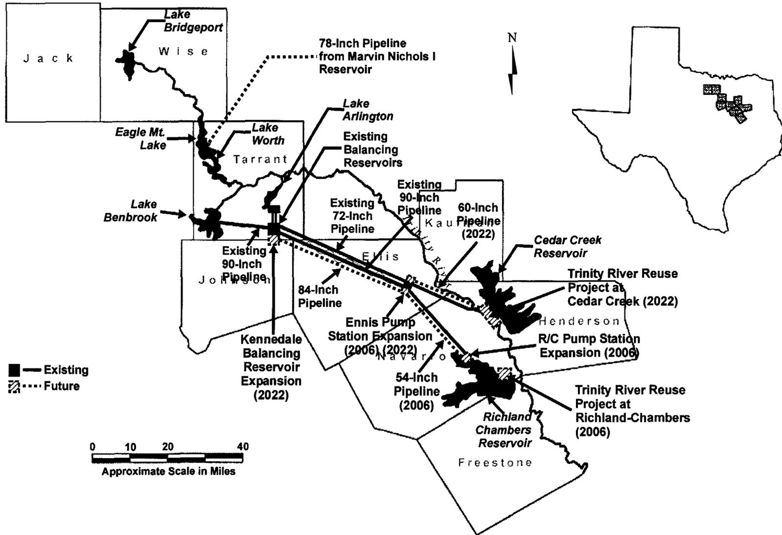
Figure 5-5. Integrated Water Supply Plan 2 — Delivery System Improvements
