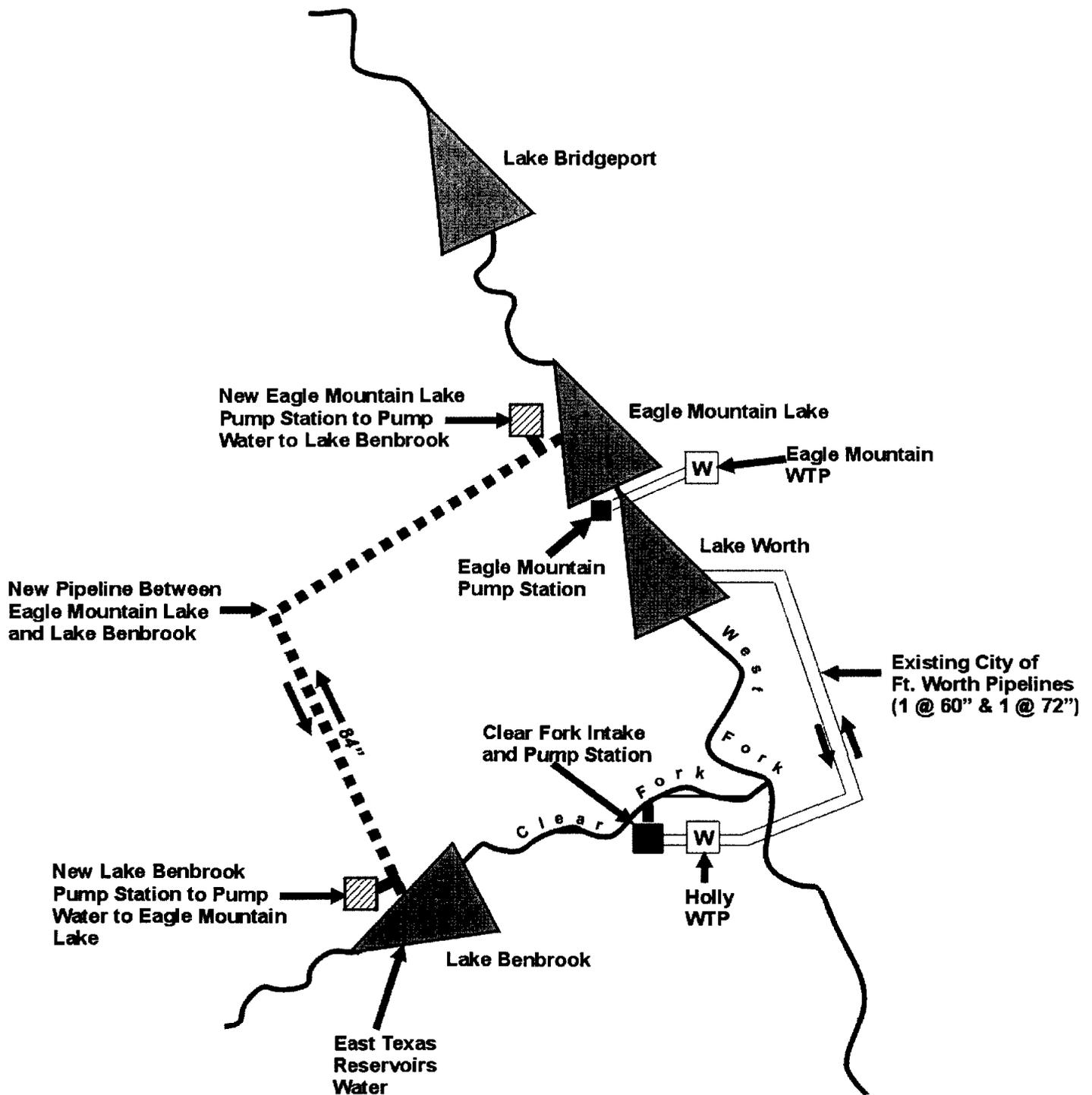
Figure 3-3. Enhancement of West Fork Water Supply (Option 2)
