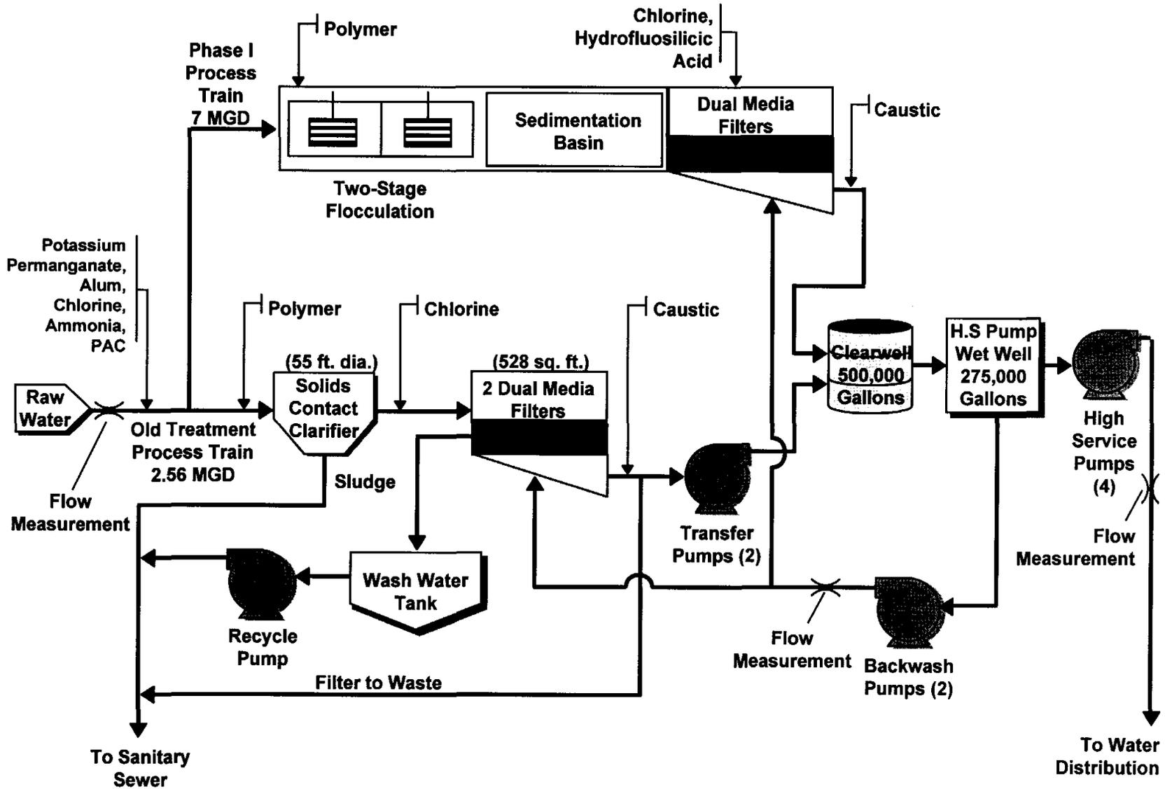
Figure 4-1. Treatment Schematic — City of Mansfield WTP
