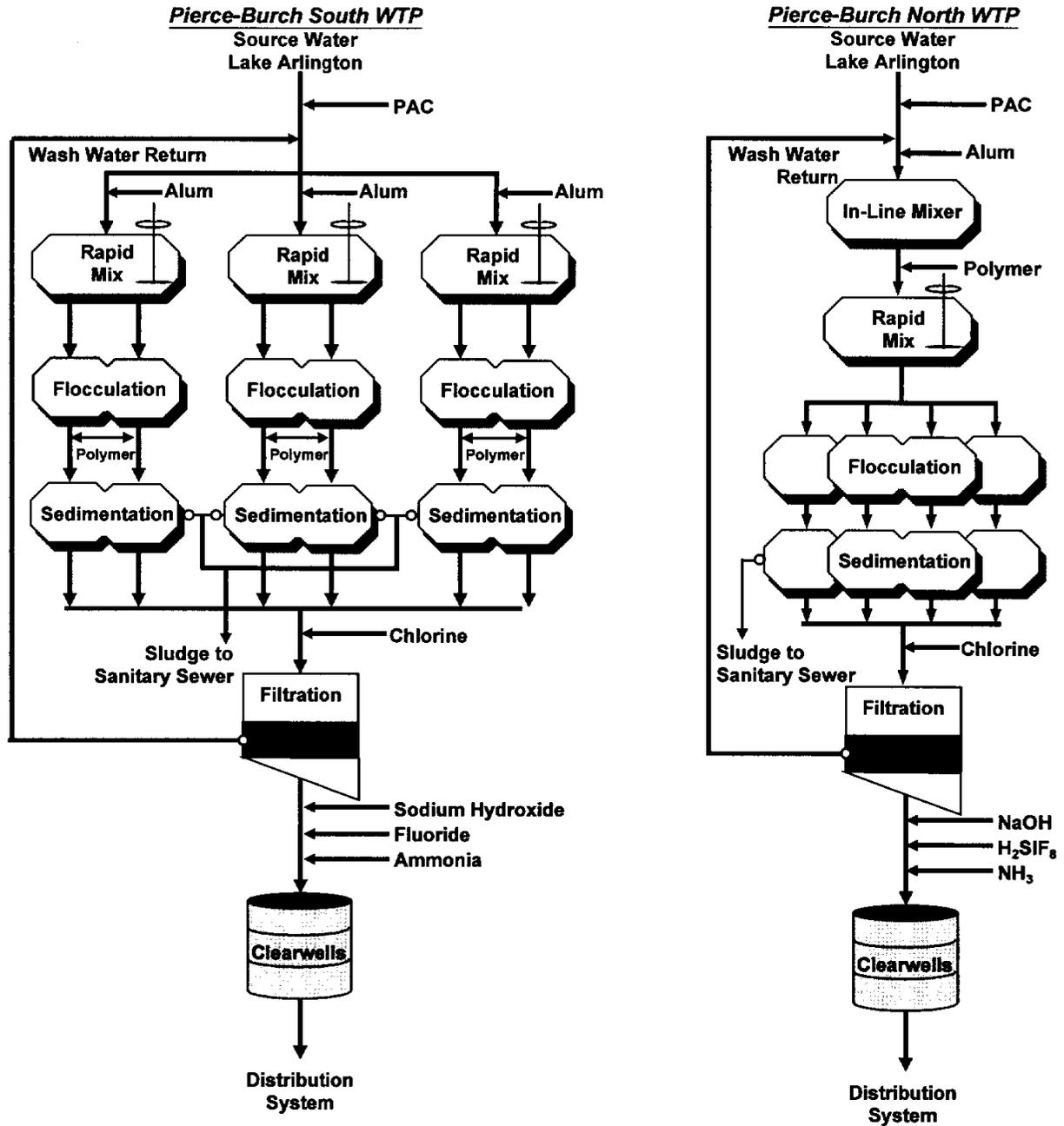
Figure 4-5. Treatment Schematics — Arlington Water Utilities
