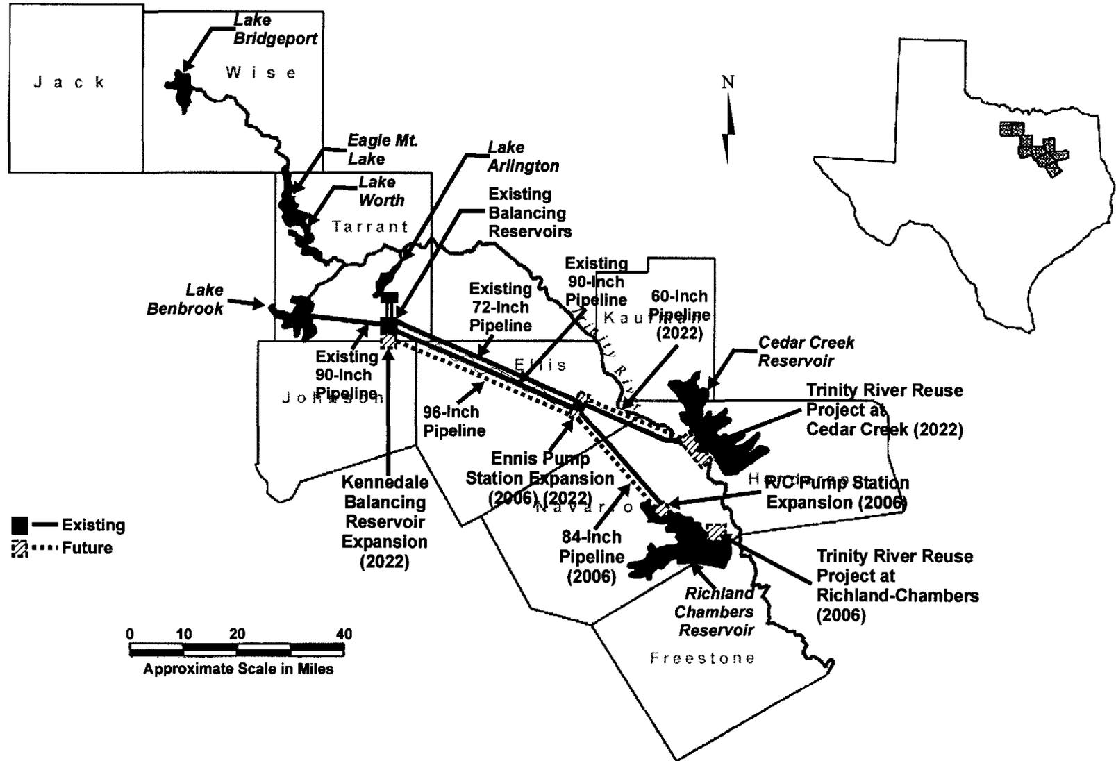
Figure 5-4. Integrated Water Supply Plan 1 — Delivery System Improvements
