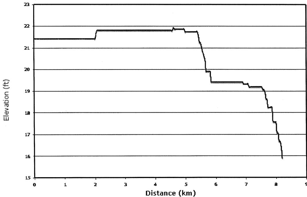
Figure 12. DEM-derived longitudinal profile of Mussel Shoals Creek.
