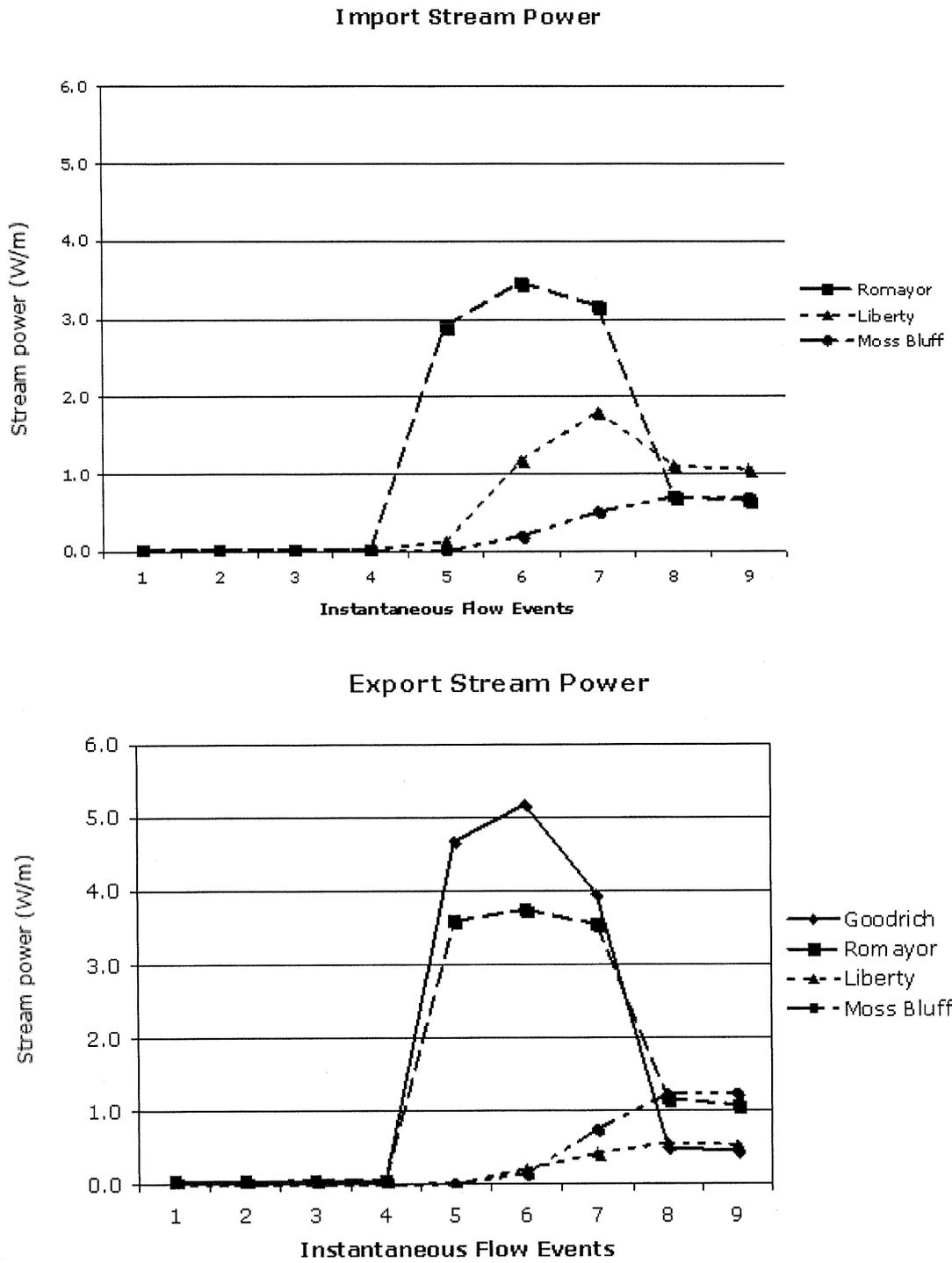
Figure 9. Stream power at Trinity River gaging stations for nine Hurricane Rita instantaneous flows, based on discharge and upstream (import) or downstream (export) slope.
