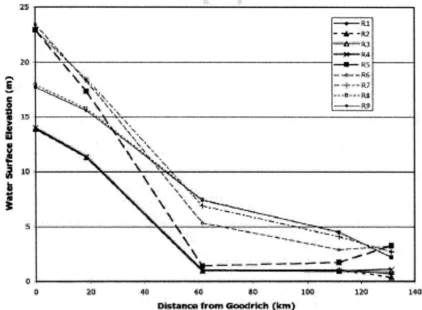
Figure 8. Water surface profiles from Goodrich to Wallisville for nine sample times during the Hurricane Rita flow event.
