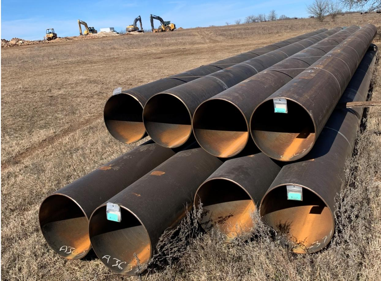
**Figure 3-14. 20-inch surface casing.**
