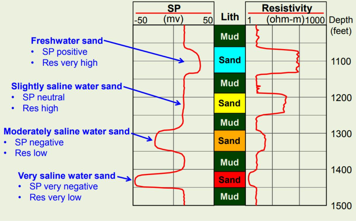
Figure 7-26. Schematic showing idealized SP and resistivity characteristics in unconsolidated formation materials under various salinity conditions (source: Introduction of TWDB Groundwater Availability Modeling Program, Queen City, Sparta, and Carrizo-Wilcox Aquifers).
