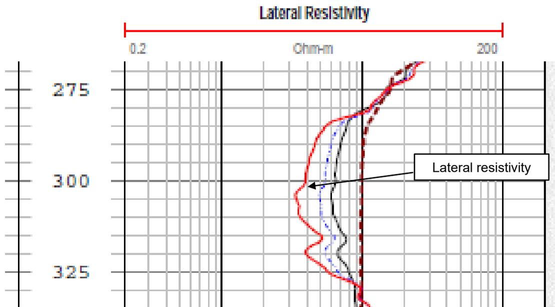
Figure 7-9. Example log for lateral resistivity tool.
