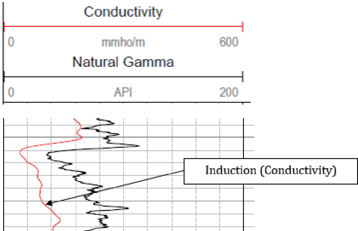
Figure 7-10. Conductivity (red line) log.
