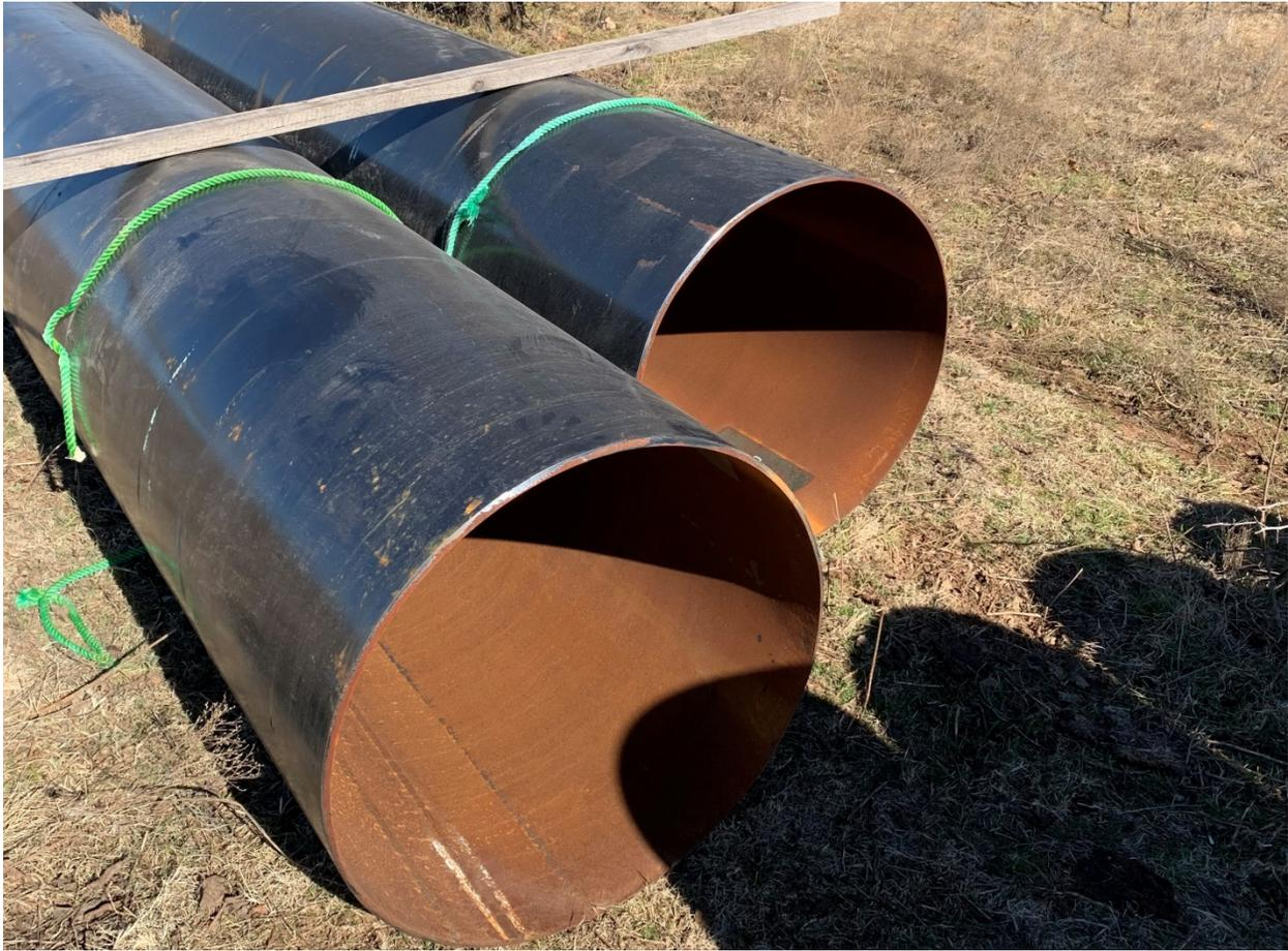
**Figure 3-12. 30-inch conductor casing.**
