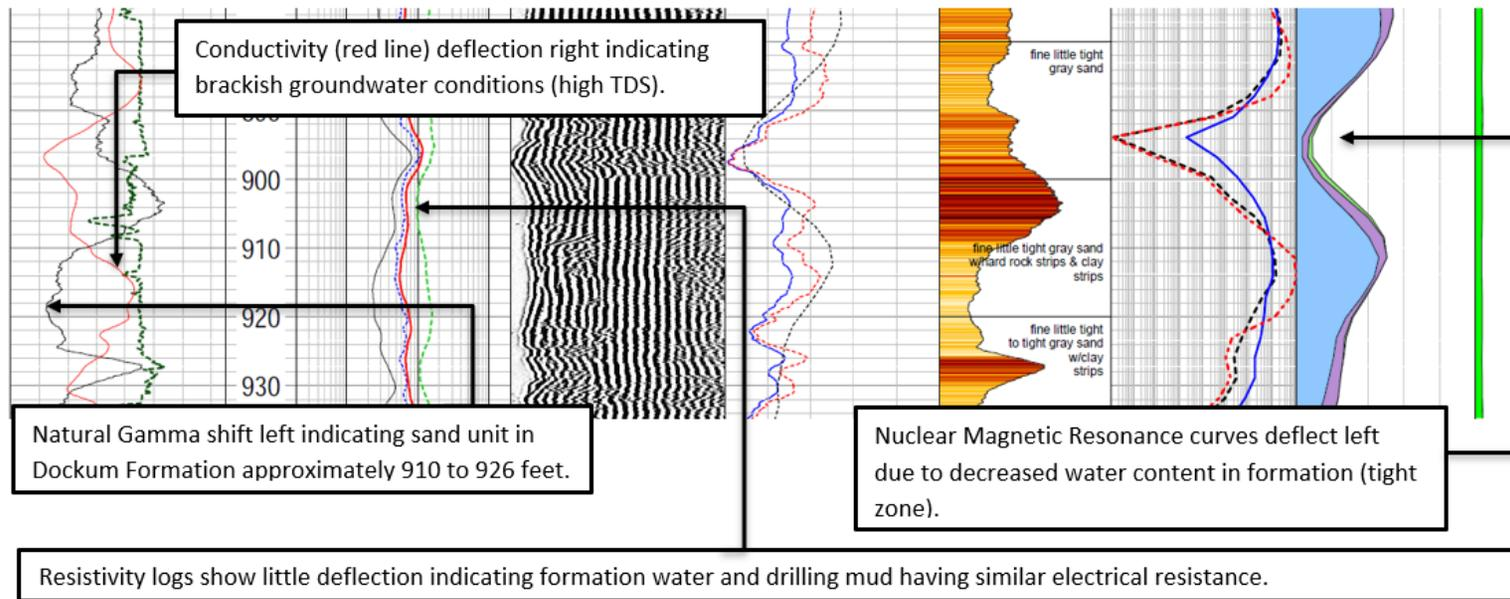
**Figure 7-24. Log of borehole drilled in unconsolidated formation materials within a brackish groundwater zone showing natural gamma ray, conductivity, resistivity, and nuclear magnetic resonance characteristics (source: High Plains Underground Water Conservation District).**
