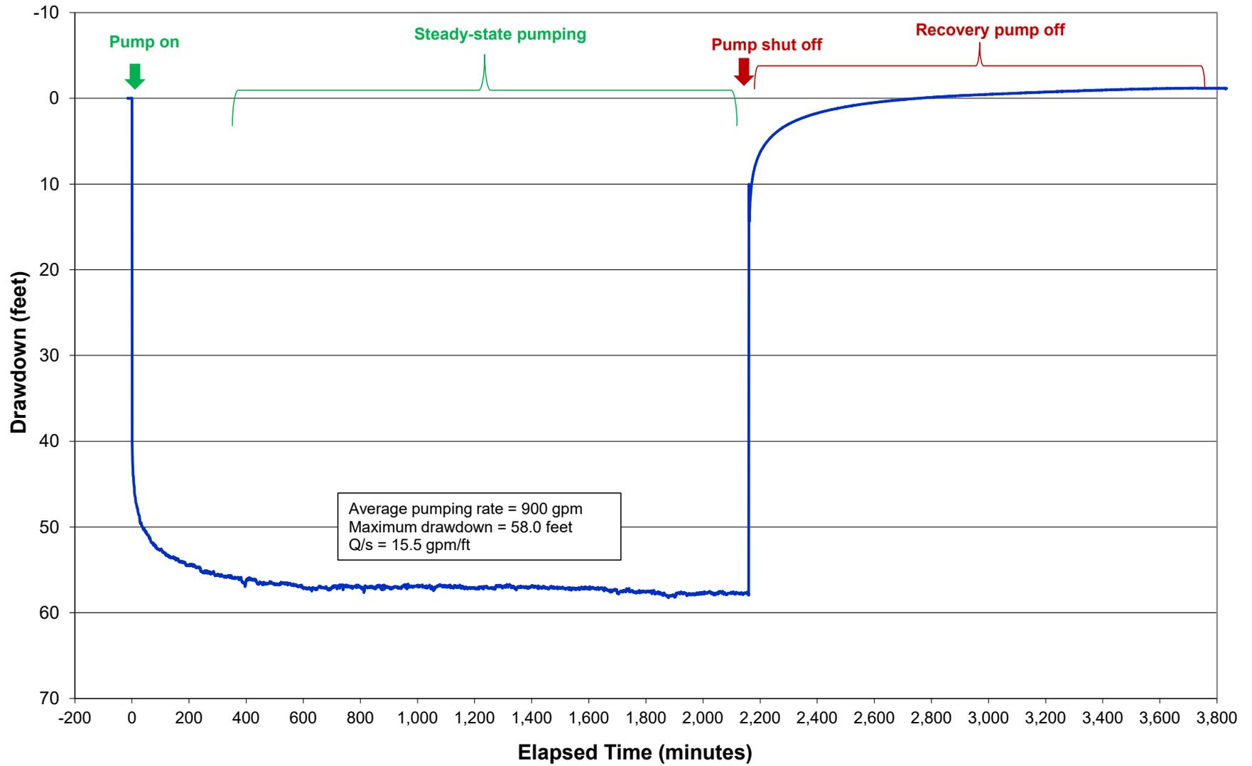
Figure 8-8. Example of a constant rate pumping test drawdown plot (source: DBS&A).
