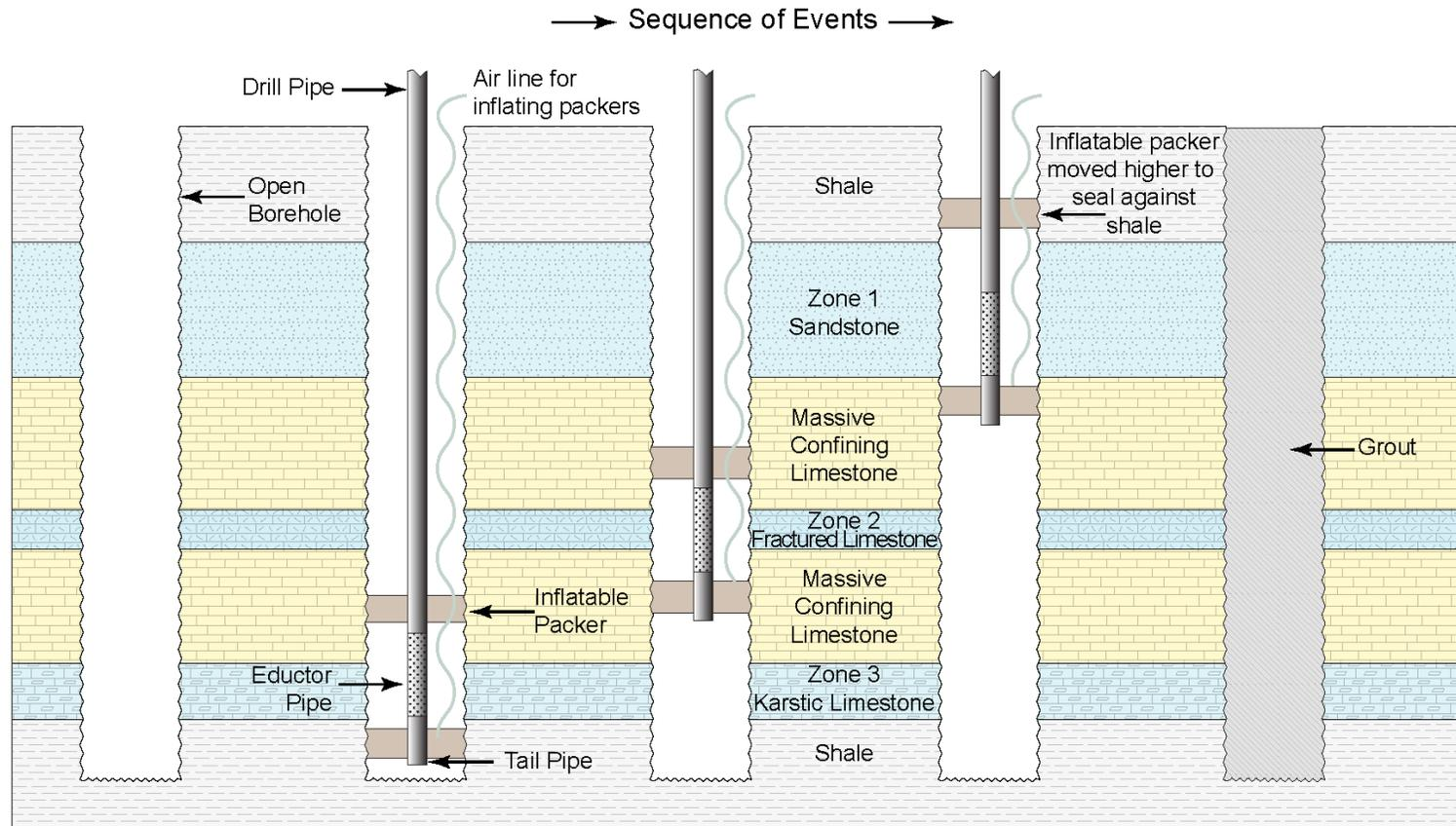
Step 1: Drill exploration borehole and perform geophysical survey.
