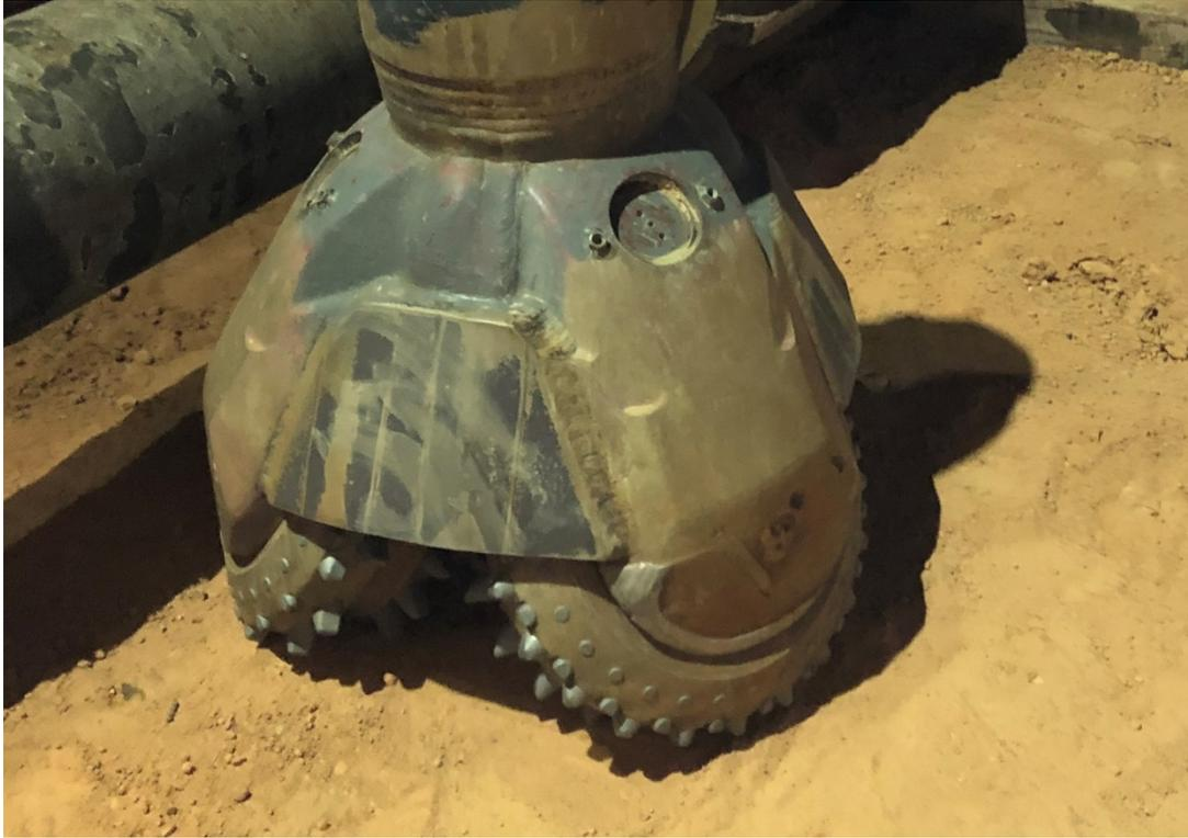
**Figure 3-4. Tri-cone bit.**
