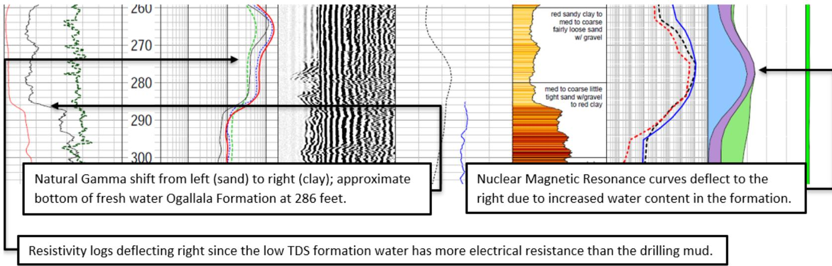
Figure 7-23. Log of borehole drilled in unconsolidated formation materials within a fresh groundwater zone showing natural gamma ray, resistivity, induction log, and nuclear magnetic resonance characteristics (source: High Plains Underground Water Conservation District).
