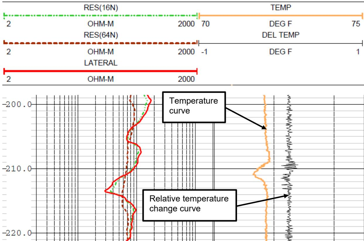
**Figure 7-20. Example of a temperature log. Temperature curve shown in orange and relative temperature change curve shown in black. Note temperature reduction (cooling) below approximately 210 feet associated with permeable zone indicated by normal resistivity curves (source: USGS GeoLog Locator; USGS NWIS Site Number: 301504097501401, USGS NWIS Station Name: YD-58-42-711, Travis County, Texas).**
