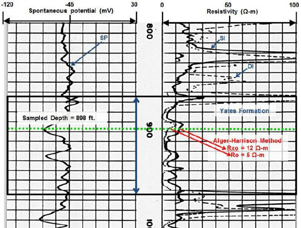
Figure 7-29. SP deflection to the left indicates a sand with a thickness greater than 10 feet. The corresponding shallow resistivity curve  $R_{x0}$  shows a resistivity reading of 12 ohm-m and the deep resistivity curve  $R_0$  shows a resistivity reading of 5 ohm-m (source: Robinson and others, 2018).
