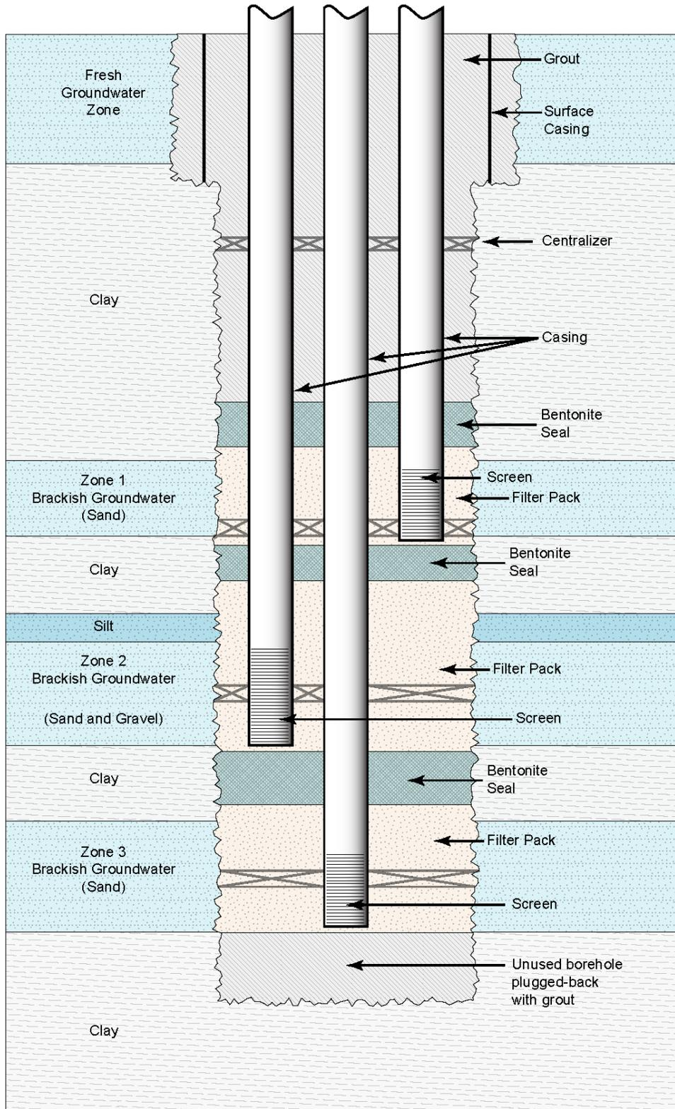
Figure 2-4. Schematic of a nested well.
