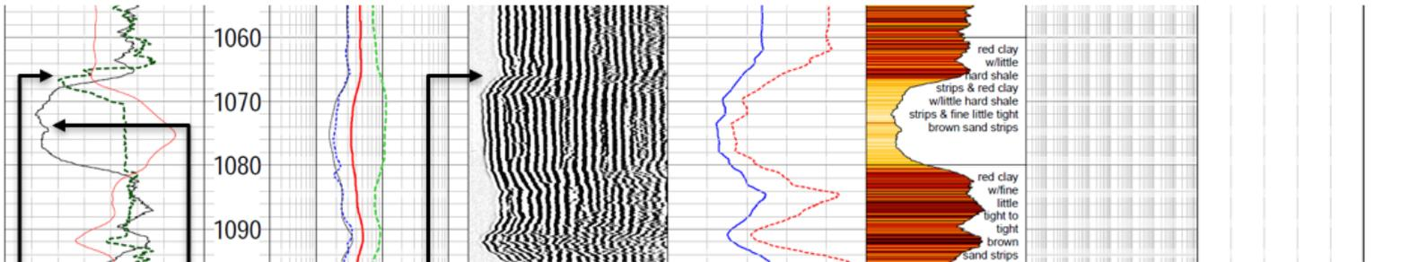
Sonic log showing transition from softer (energy-absorbing) clay to harder (energy reflecting) sand approximately 1,066 to 1,082 feet. Hard streak also shown at approximately 1,093 feet.
