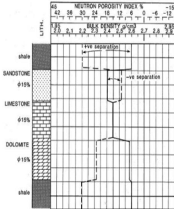
Figure 7-13. Bulk density of various formation materials (source: Rider, 1996).
