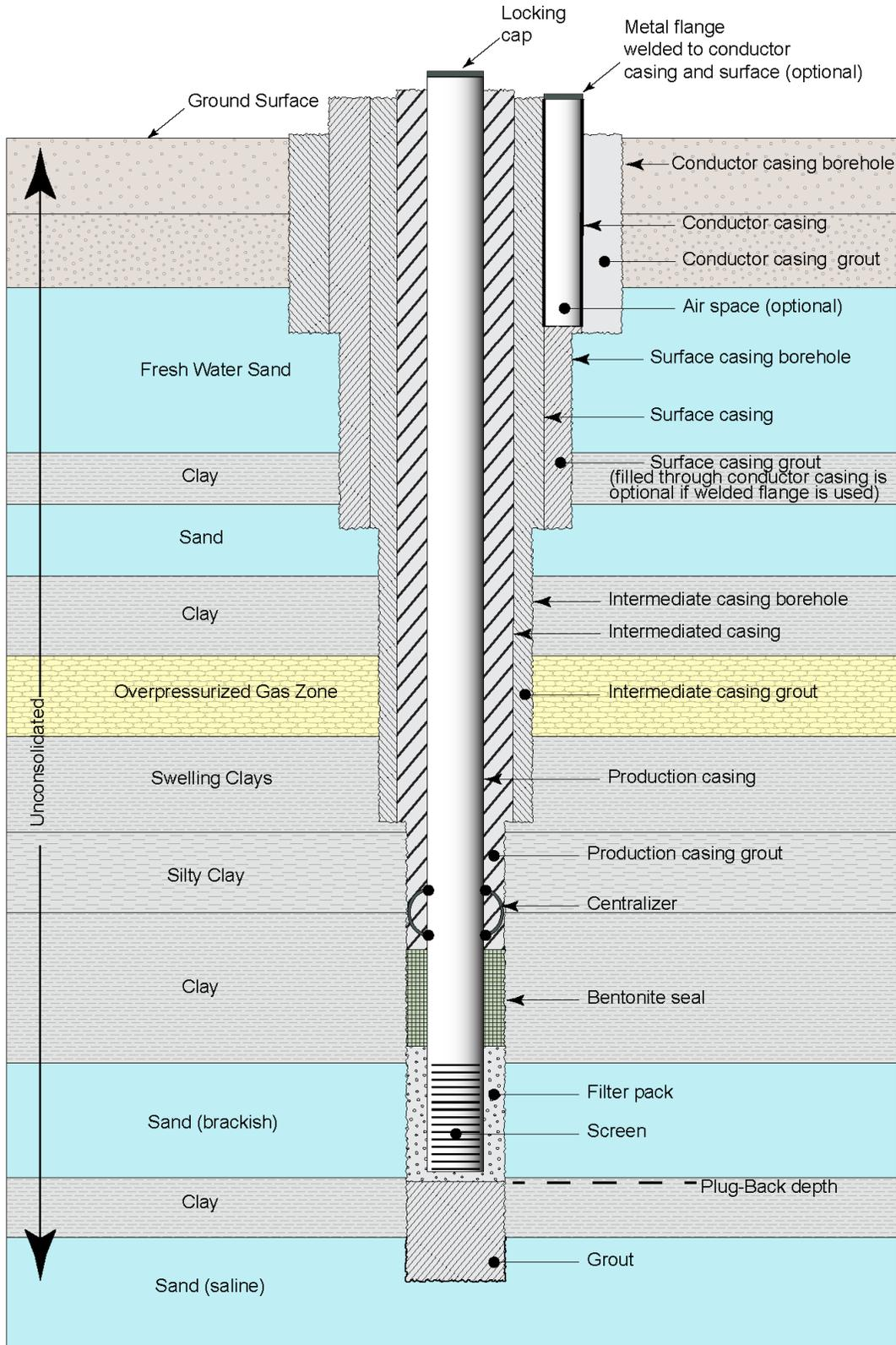
Figure 3-11. Standard well completion in unconsolidated formation materials.
