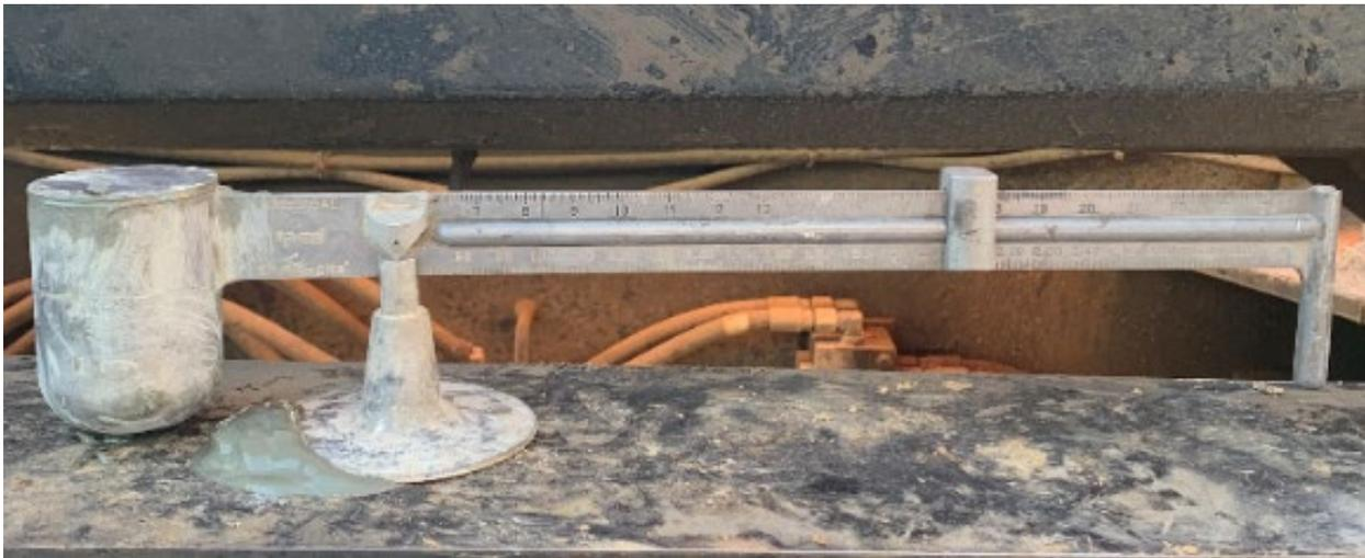
Figure 7-28. Mud scale (source: DBS&A).
