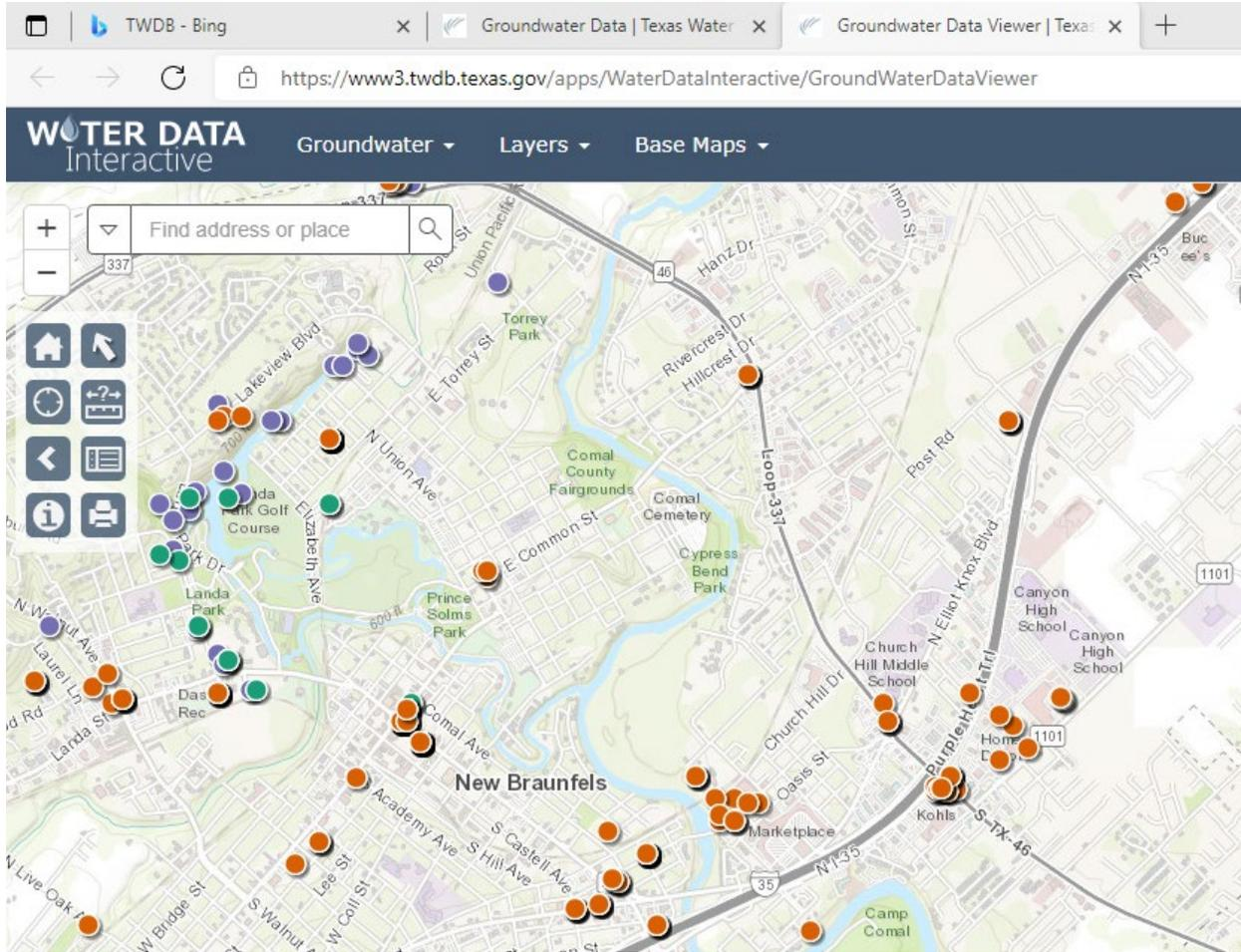
**Figure 5-1.** Screenshot from the TWDB Water Data interactive website. This map shows the availability of TWDB database wells (purple dots), TDLR well reports (orange dots), and BRACS database wells (green dots).
