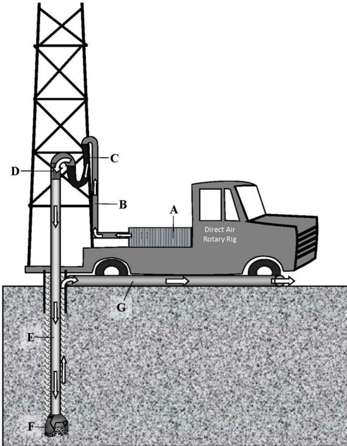
Figure 3-3. Direct air-rotary drilling system (source: Glotfelty, 2019). The drilling fluid circulation path is shown by arrows. A: Air compressor, B: Stand pipe, C: Kelly hose, D: Swivel, E: Drill pipe and collars, F: Drill bit, G: Blooey line.
