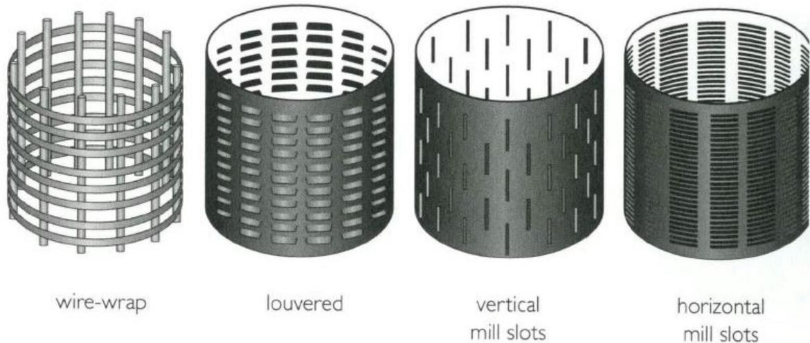
Figure 3-15. Common well screen types (source: Glotfelty, 2019).
