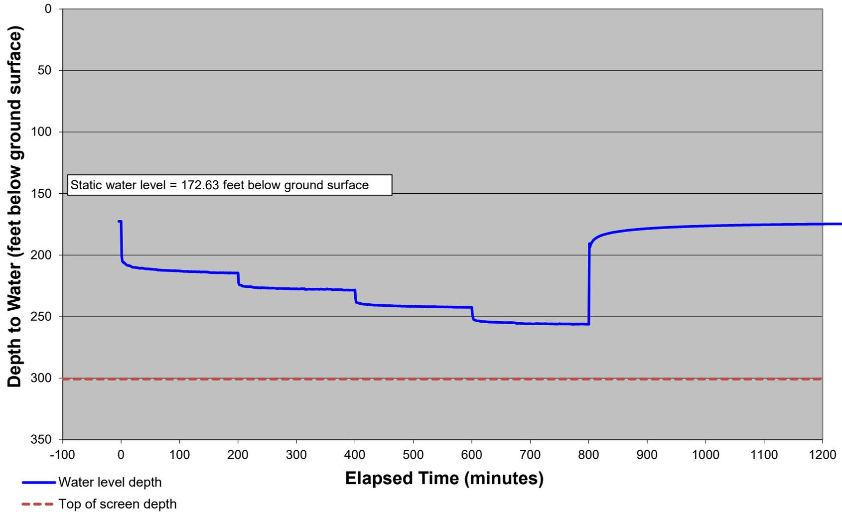
Figure 8-7. Example step drawdown data showing the water level depth versus time relative to a near-surface measuring point and the top of the screen interval (source: DBS&A).
