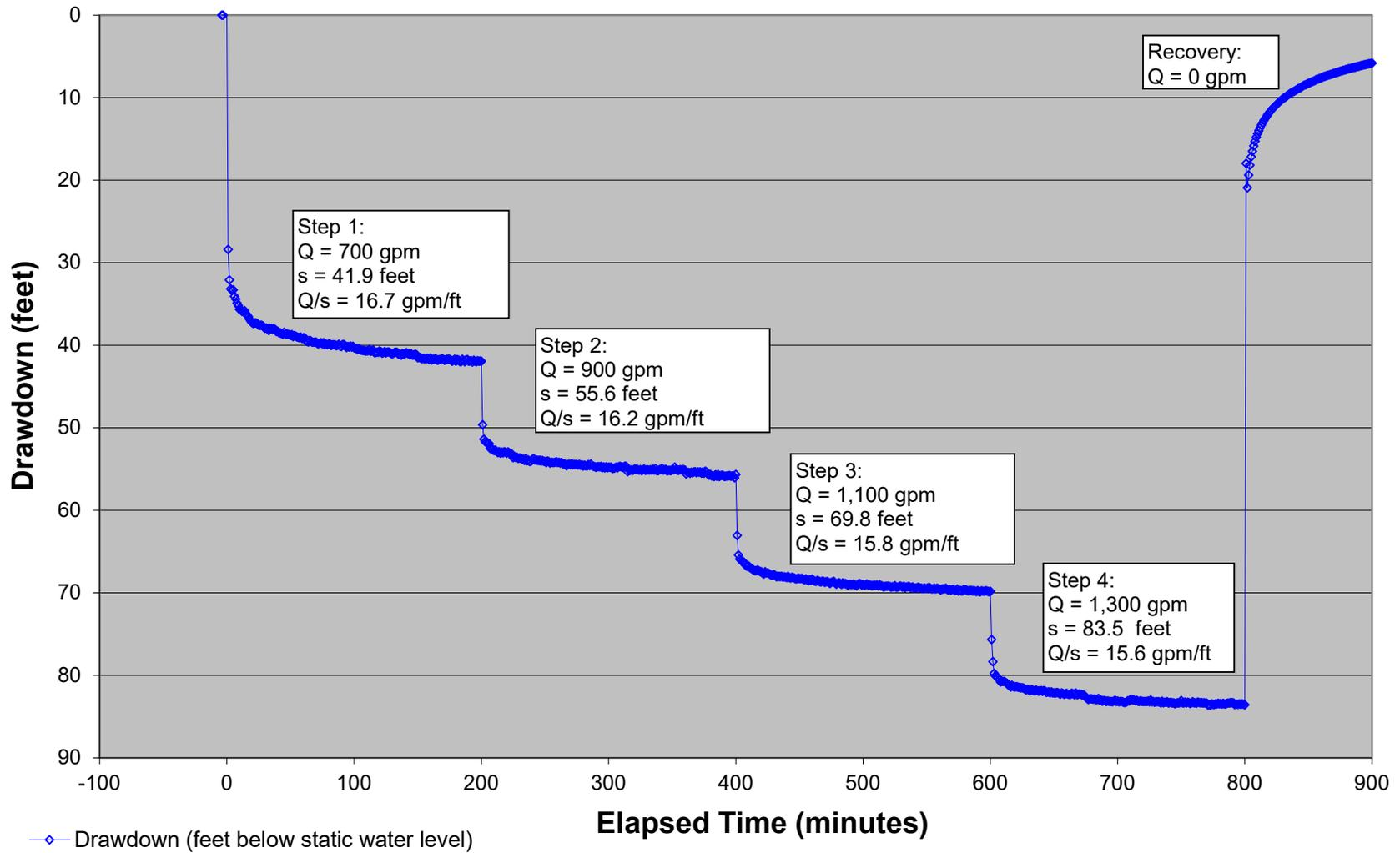
Figure 8-6. Example of a step drawdown test plot of drawdown versus time (source: DBS&A).
