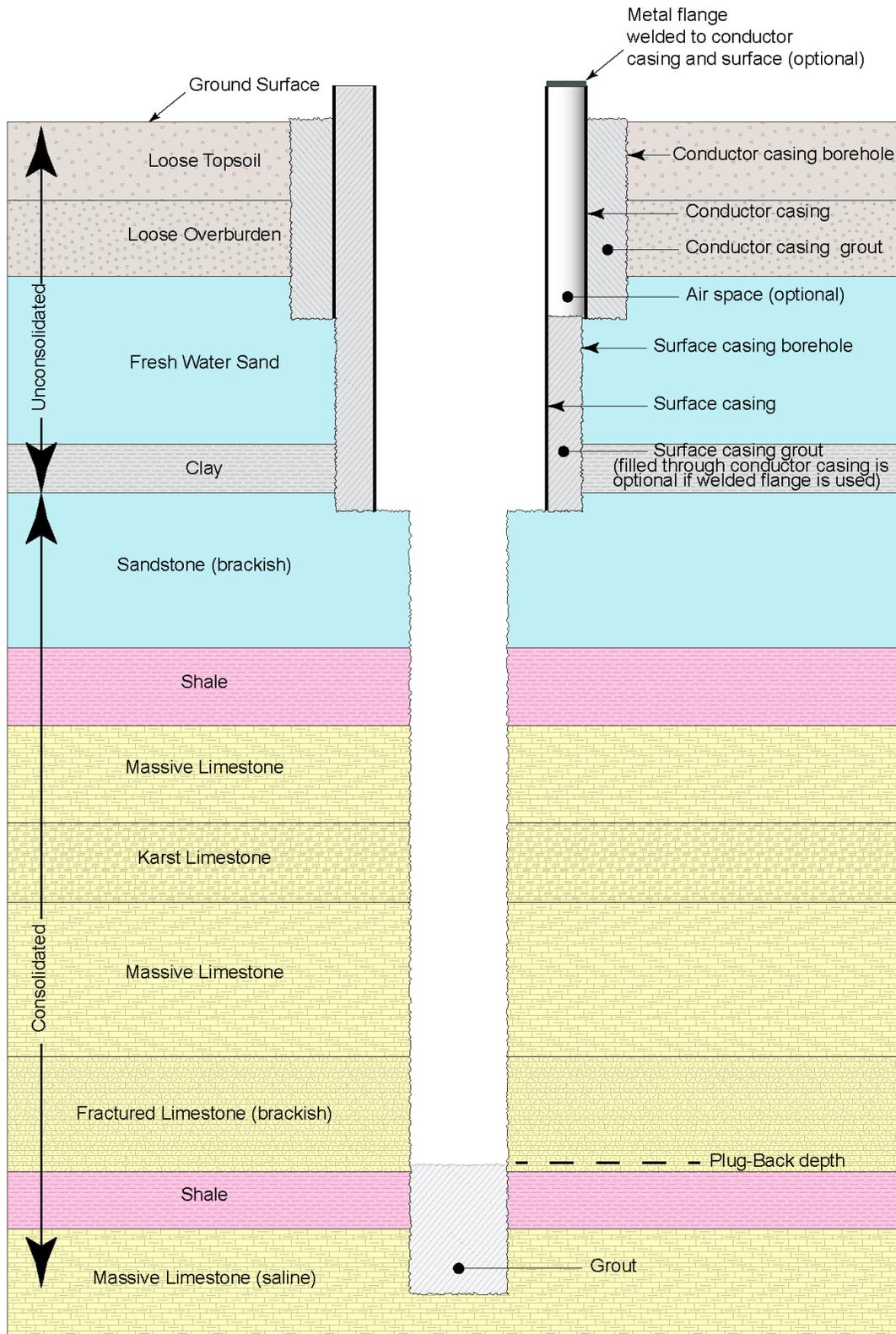
Figure 3-16. An open hole completion in consolidated formation materials.
