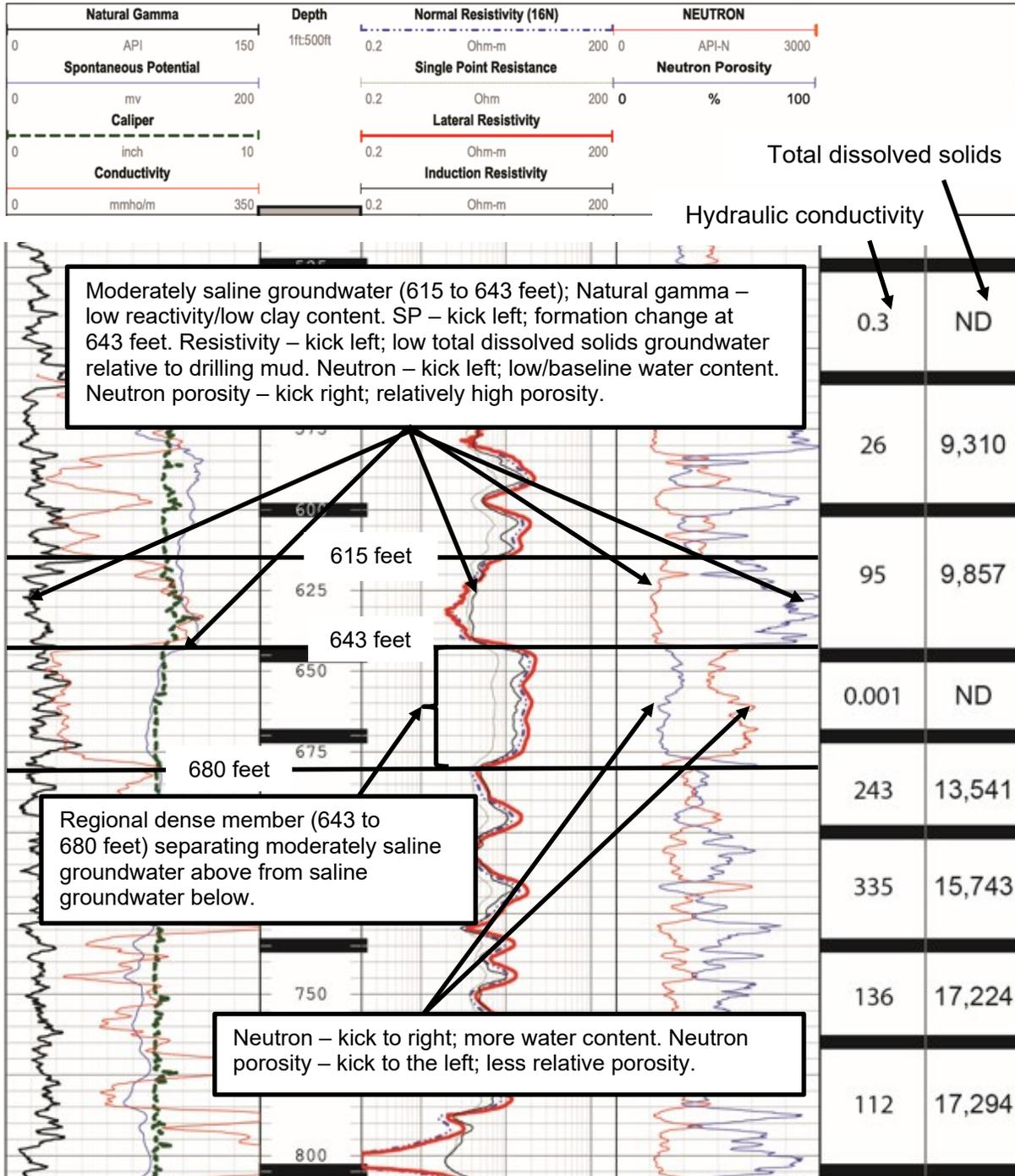
Figure 7-22. Log showing various log responses within a transition zone of a limestone interval (source: Barton Springs Edwards Aquifer District).
