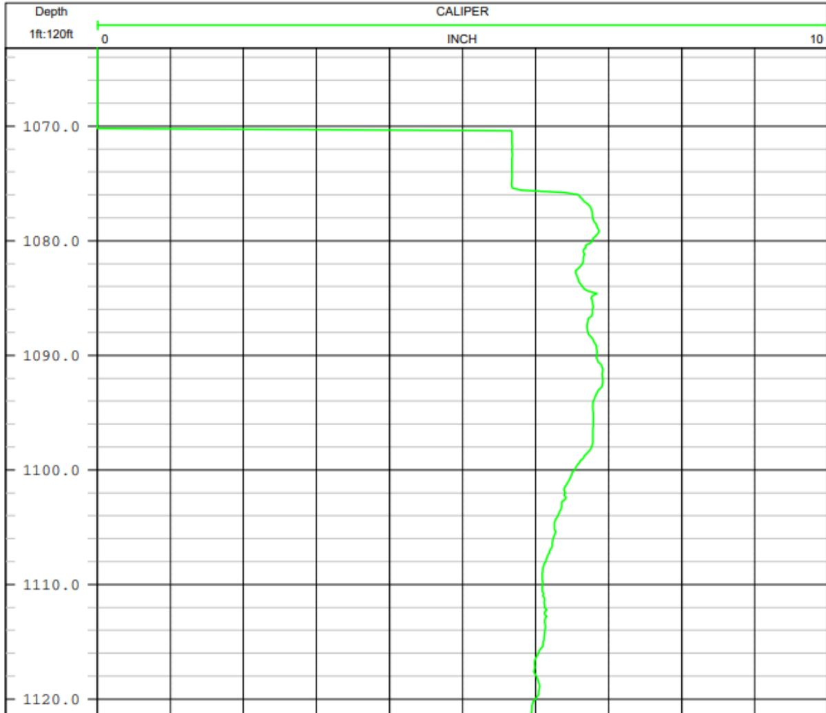
**Figure 7-17. Example of a caliper log. Bottom of intermediate casing set at approximately 1,075 feet below ground surface as indicated by straight vertical line, and formation washout immediately below the casing (source: USGS GeoLog Locator; USGS NWIS Site Number: 291612099302001, USGS NWIS Station Name: YP-69-44-902 East Uvalde 2, Uvalde County, Texas).**
