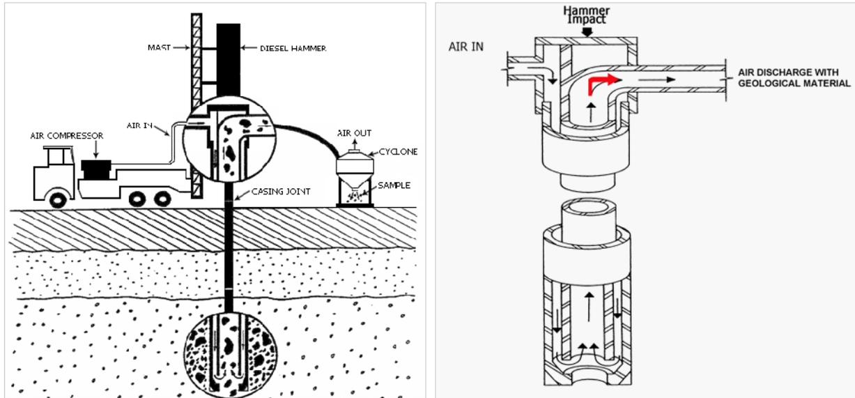
**Figure 3-9. Becker hammer drilling method (source: Great West Drilling, 2021). Compressed air travels through the annulus (interstitial void) of the dual-wall drive pipe as the drive pipe is driven. No rotation of the drive pipe occurs. Drill cuttings are entrained in the compressed air and are discharged through a cyclone at the ground surface.**
