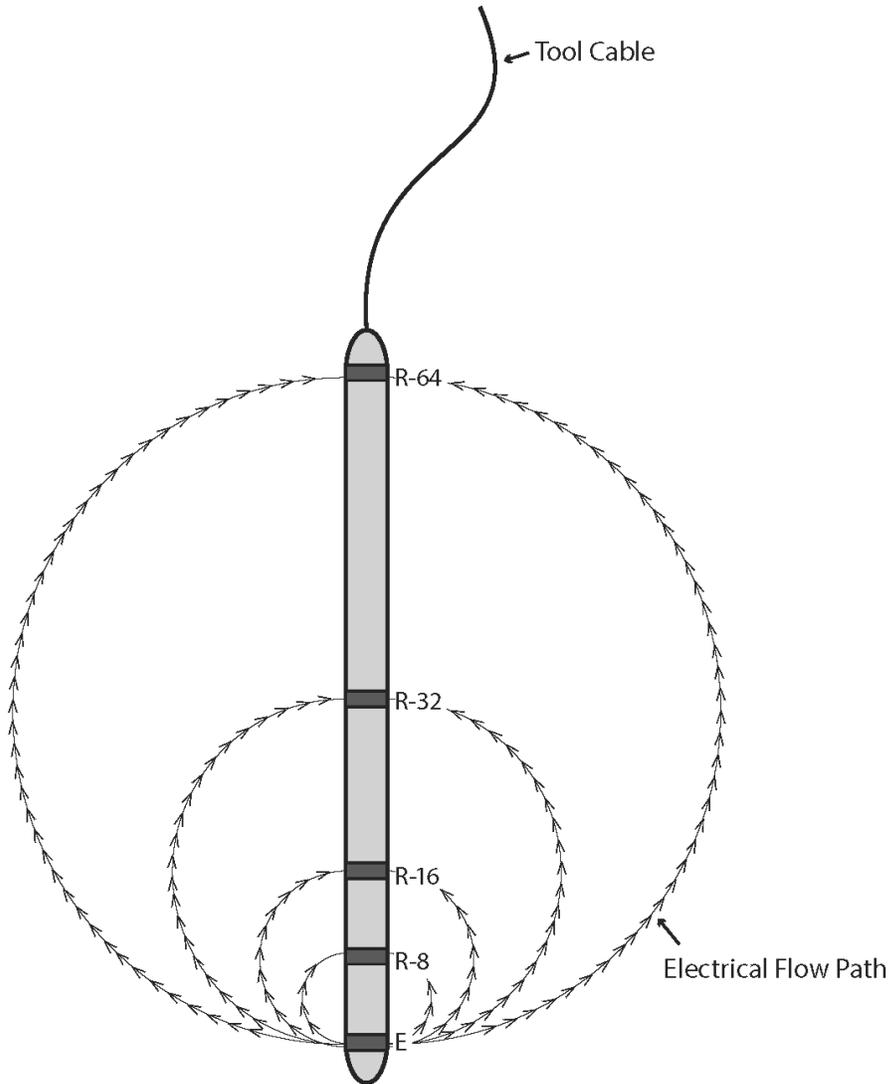
**Figure 7-7. Normal resistivity tool schematic.**
