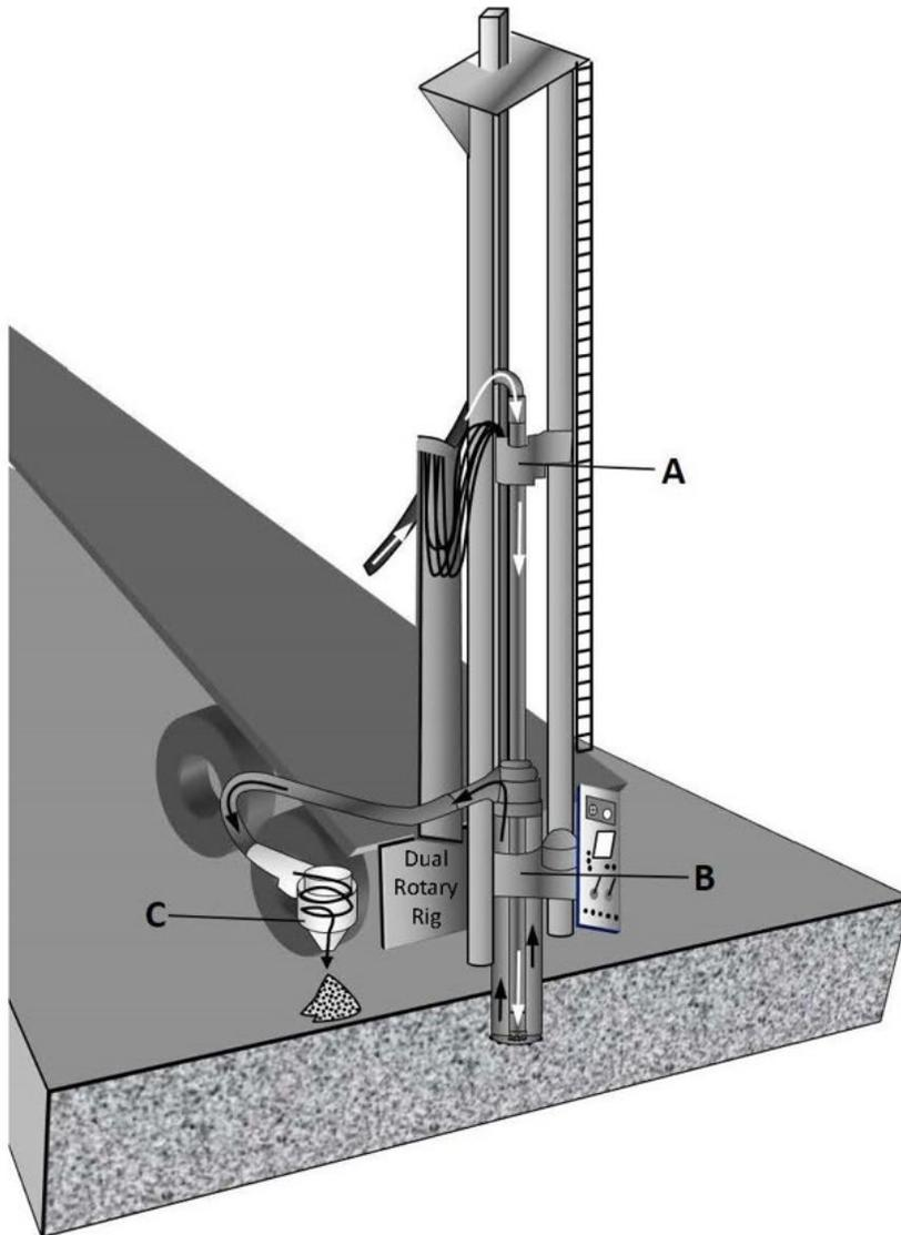
Figure 3-7. Dual-rotary circulation drilling system (source: Glotfelty, 2019). The compressed air or drilling fluid flow path is shown by arrows. The upper drive head (A) rotates the inner drill pipe, and the lower drive head (B) rotates the DR casing. Cuttings are discharged to a cyclone (C) or a mud pit.
