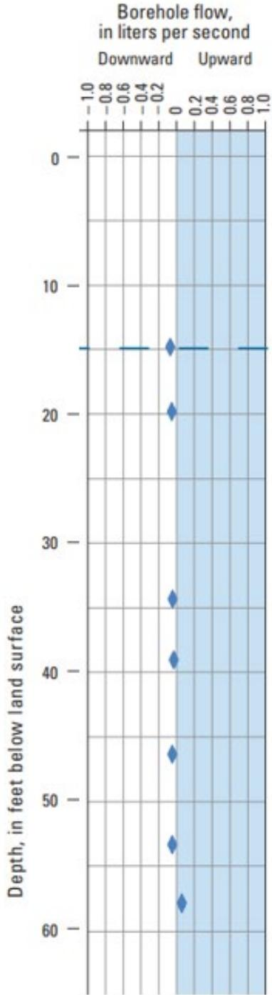
Figure 7-19. Example of flow meter log. Blue diamonds represent the flow in liters per second, with downward flow from the static water level (blue dashed horizontal line) to approximately 55 feet below ground surface and upward flow at approximately 58 feet below ground surface (source: Clarke and others, 2011).
