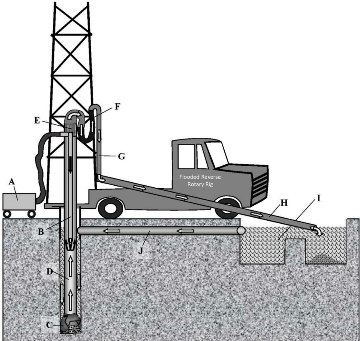
Figure 3-6. Flooded reverse-rotary drilling circulation system (source: Glotfelty, 2019). The compressed air flow path is shown by solid arrows, while the drilling fluid circulation path is shown by open arrows. A: Air compressor, B: Air line, C: Drill bit, D: Drill pipe and collars, E: Swivel, F: Kelly hose, G: Stand pipe, H: Flow line, I: Mud pit, J: Return flow line.
