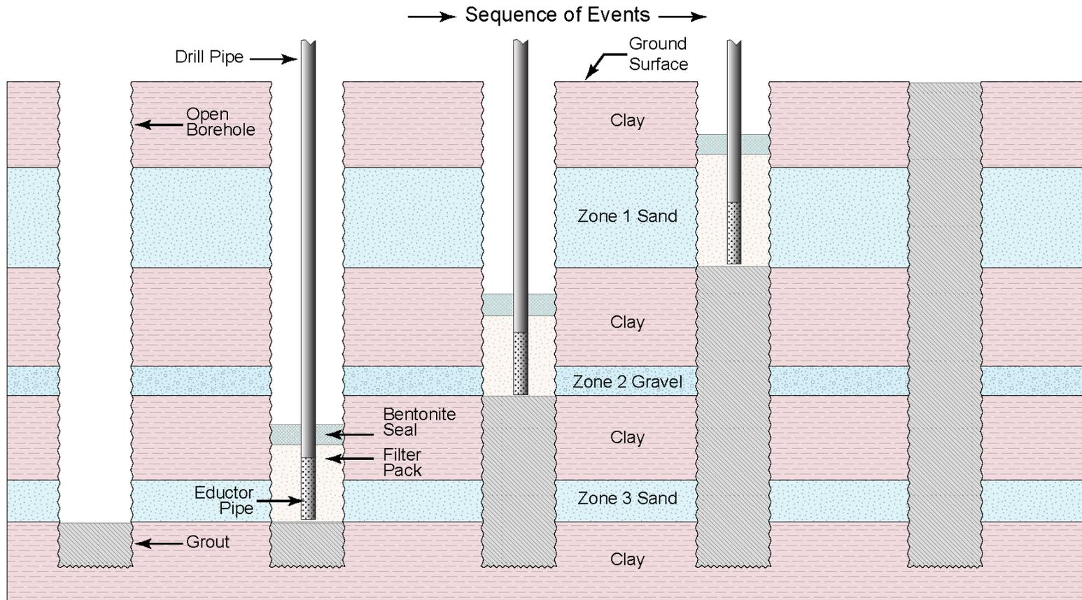
Step 1: Drill exploration borehole, perform geophysical survey, and plug back.
