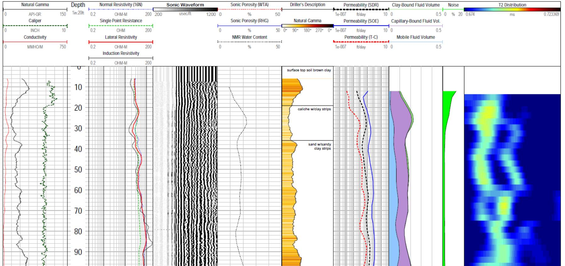
Figure A-1. Geophysical log from the exploratory test boring.
