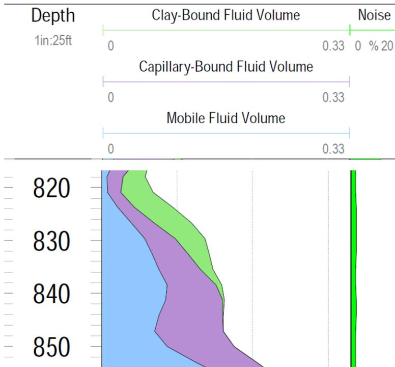
Figure 7-15. Example of nuclear magnetic resonance log. Green color shows fluid bound by clay, purple color shows fluid bound within the capillary portion of the formation, and blue color shows mobile fluids (source: High Plains Underground Water Conservation District, Dockum Test Well; USGS NWIS Site Number 341816101570901, Station Name KY-11-41-5xx).
