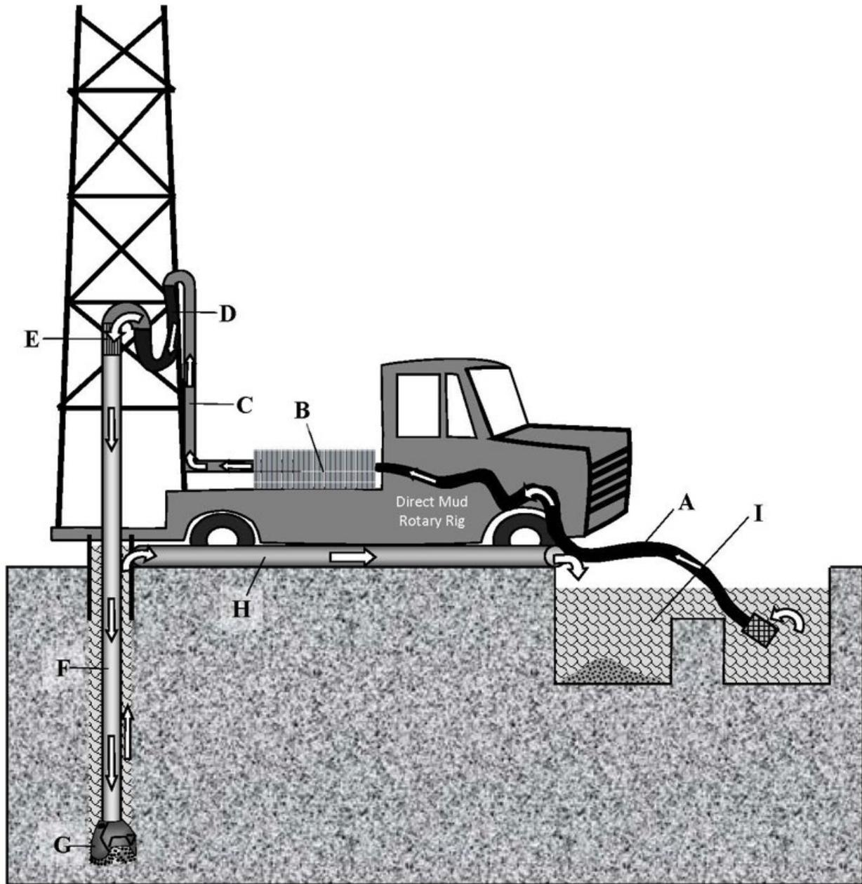
Figure 3-1. Direct mud-rotary drilling system (source: Glotfelty, 2019). The drilling fluid circulation path is shown by arrows. A: Intake line, B: Mud pump, C: Stand pipe, D: Kelly hose, E: Swivel, F: Drill pipe and collars, G: Drill bit, H: Return flow line, I: Mud pit (may be above-ground open-top steel tank).
