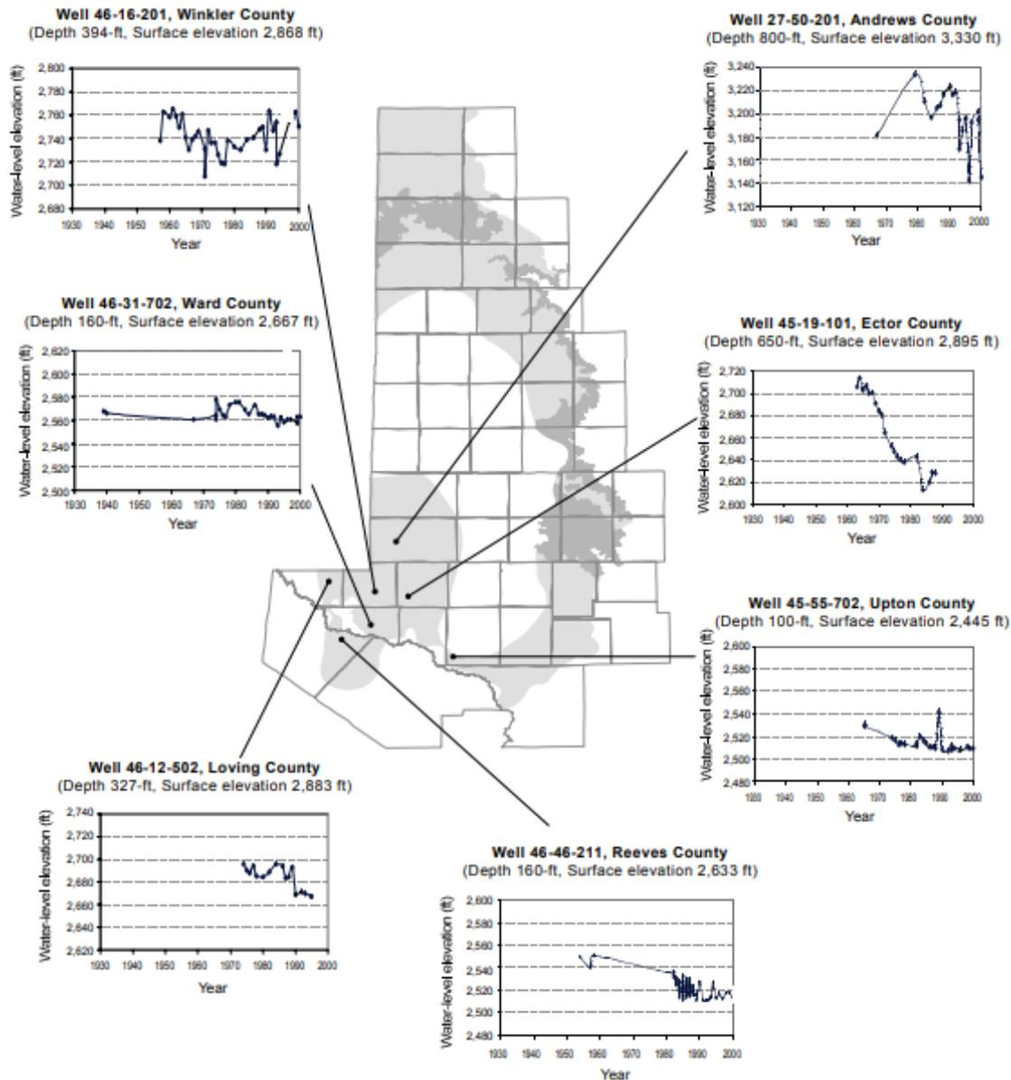
Figure 8-5. Example of hydrographs (source: Bradley and Kalaswad, 2003). These plots were used as a visual aid to evaluate water level trends in the Dockum Aquifer wells over long time periods.
