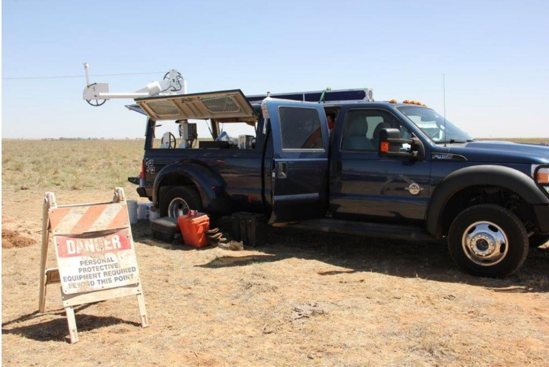
Figure A-4. Geophysical logging truck at the drilling site.
