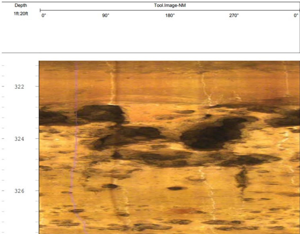
**Figure 7-18. Example optical log showing sidewall image of a karstic limestone with solution cavities (source: USGS GeoLog Locator, USGS NWIS Site Number 294529098360401, USGS NWIS Station Name: CampStandley-CSI-LGR, Comal County, Texas).**
