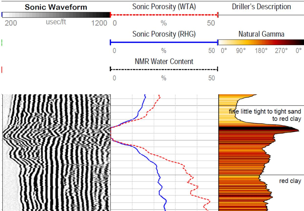
Figure 7-16. Example of an acoustic log. Sonic (acoustic) waveform plot shows deflection to the left where acoustic travel speed is reduced entering a clay zone (source: High Plains Underground Water Conservation District, Dockum Test Well).
