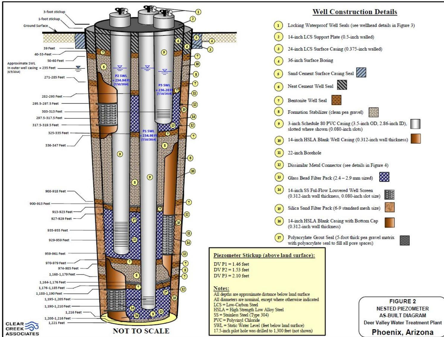
Figure D-3. As-built diagram of Deer Valley nested well.
