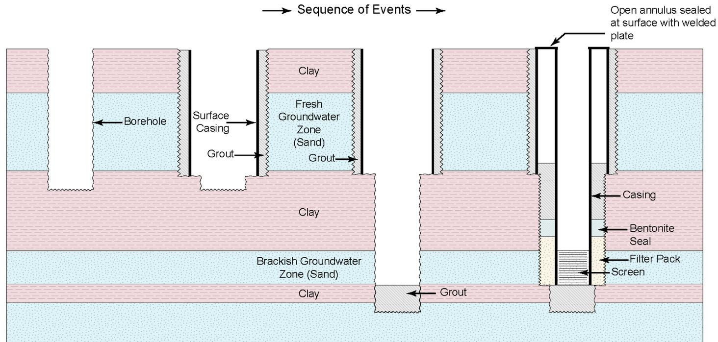
Step 1: Drill pilot borehole and perform geophysical survey to identify fresh groundwater zone.
