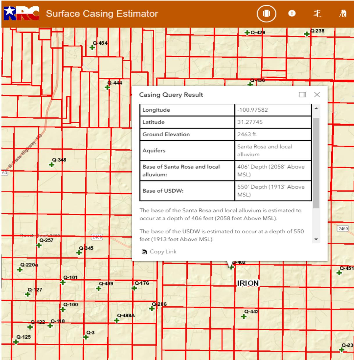
Figure 5-5. RRC surface casing estimator website.
