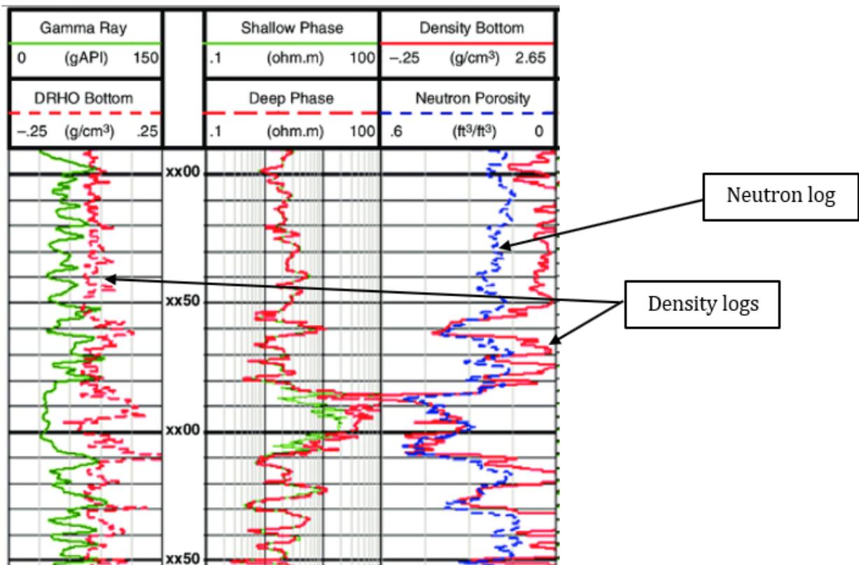
Figure 7-14. Example of density (gamma-gamma) and neutron logs.
