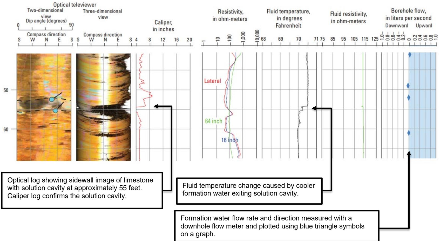
Figure 7-27. Optical, caliper, and fluid temperature logs used with a borehole flow graph to study flow characteristics within a well (source: Clarke and others, 2011).
