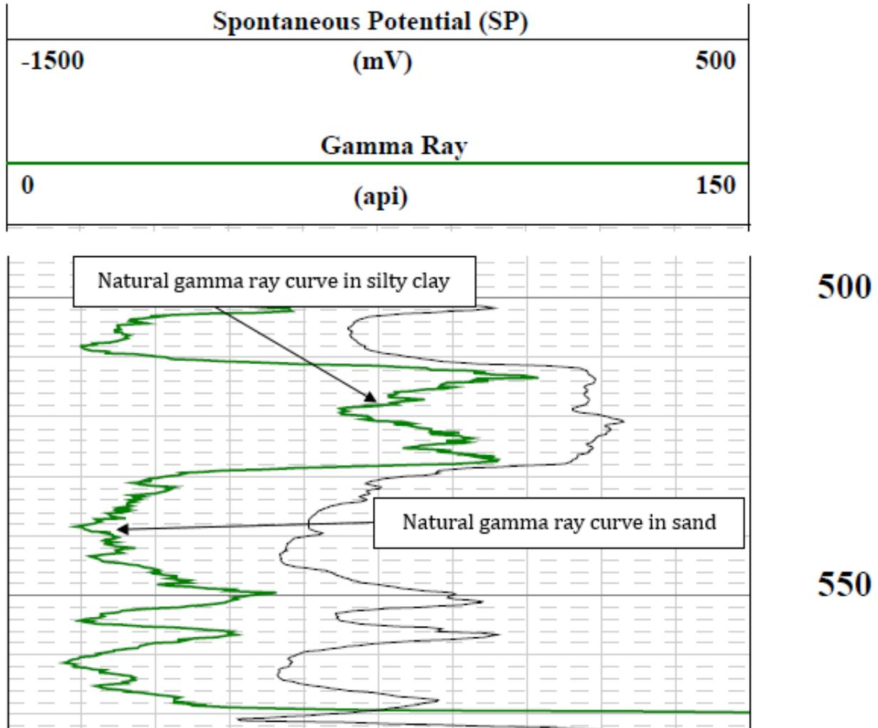
Figure 7-12. Example natural gamma log curves.
