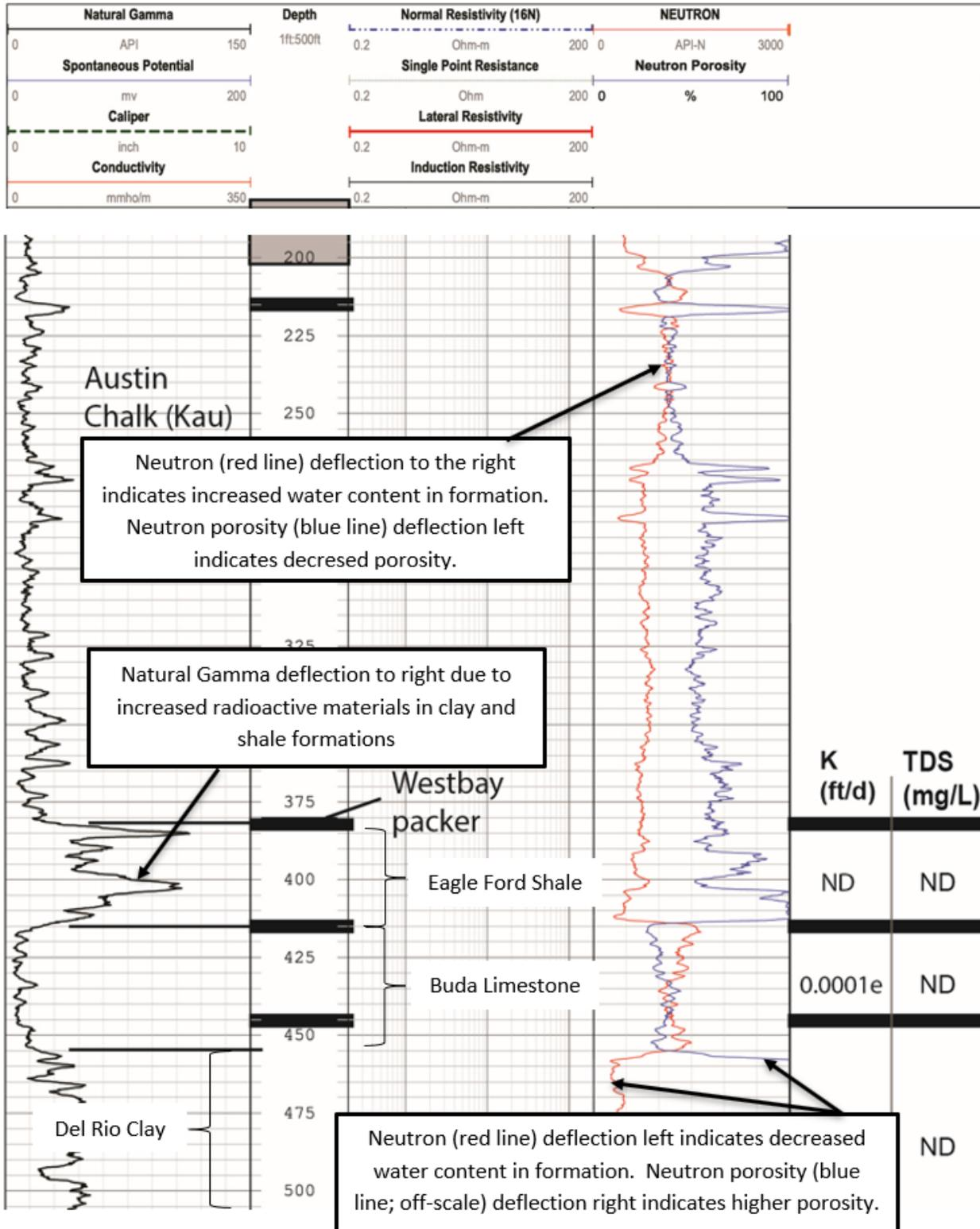
Figure 7-21. Log of borehole drilled in consolidated and unconsolidated materials within a fresh groundwater zone, showing natural gamma ray and neutron characteristics (source: Barton Springs Edwards Aquifer District).
