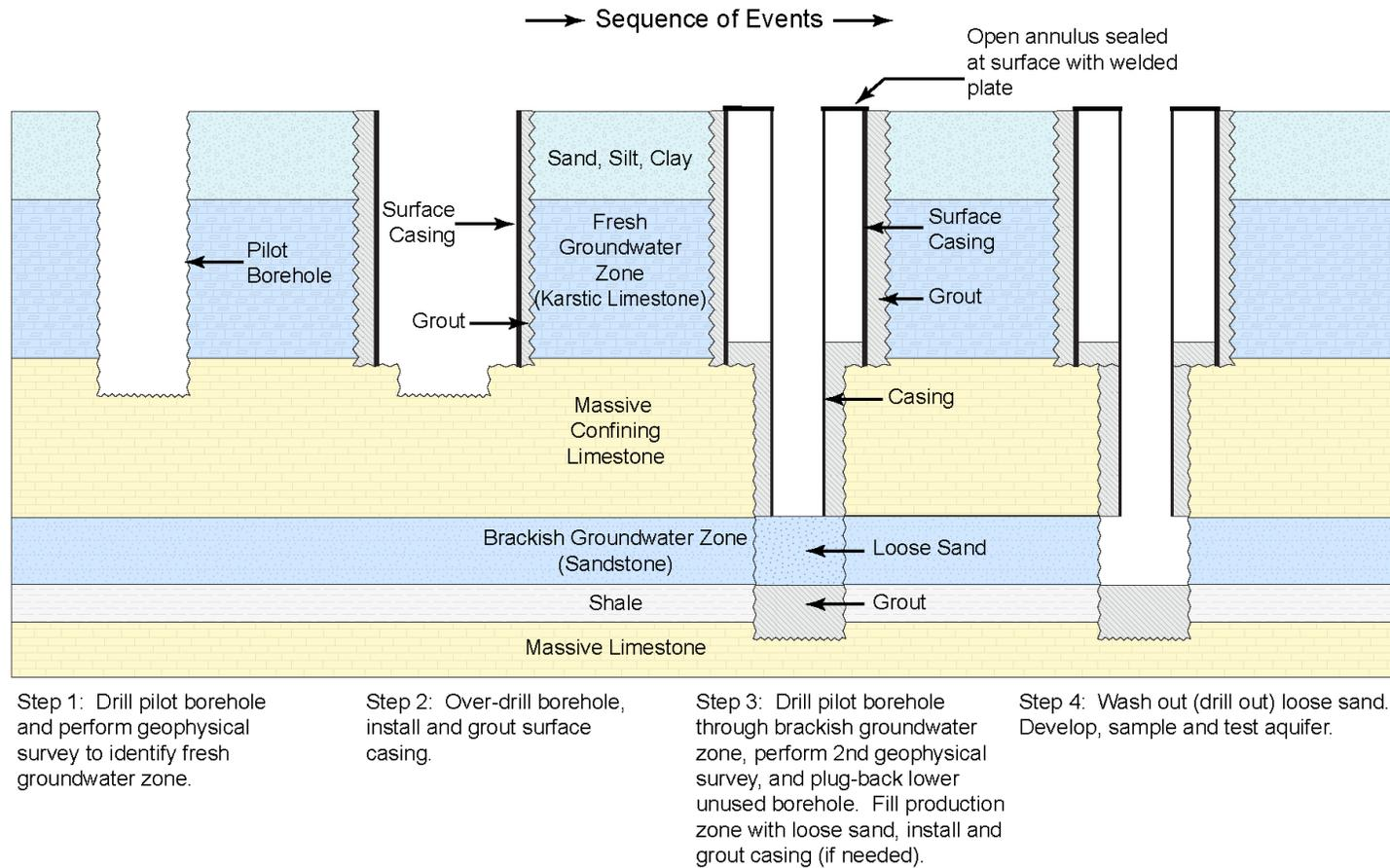
**Figure 2-2. Construction sequence for single-zone test well in consolidated formations.**
