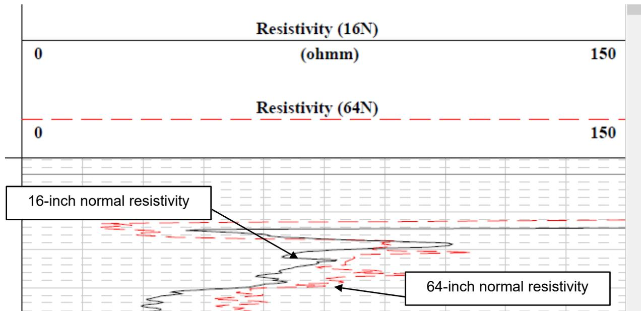
Figure 7-8. Log scale and curves for 16-inch and 64-inch electrode spacing normal resistivity tools.
