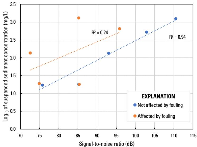
Figure 11. Relation between signal-to-noise ratio (in decibels) and suspended-sediment concentrations (in milligrams per liter) in a subset of data collected at USGS station 08162501 Colorado River near Wadsworth, TX affected by biofouling.
