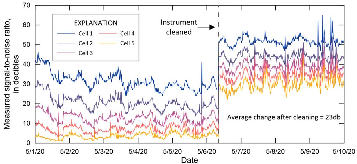
Figure 10. Signal-to-noise ratio before and after acoustic Doppler velocity meter at USGS station 08162501 Colorado River near Wadsworth, TX was cleaned to remove barnacles.
