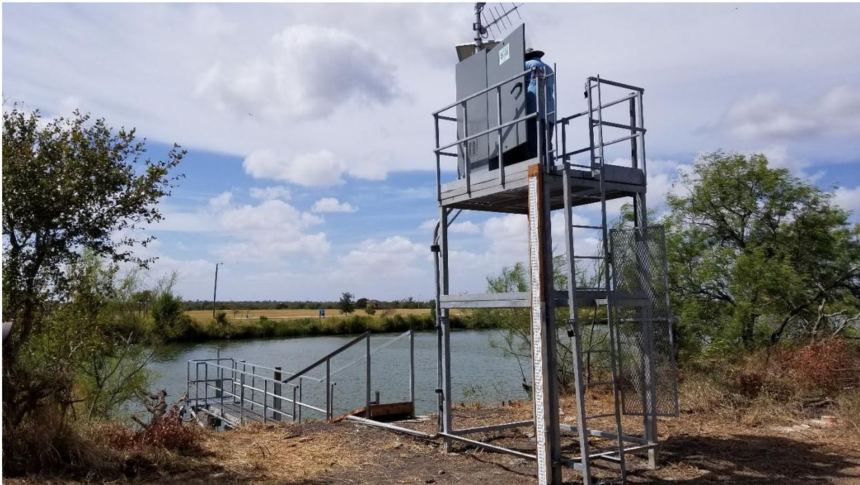
Figure 18. Streamgauge installed at USGS station 08211502 Nueces River near Odem, TX, August 2019.
