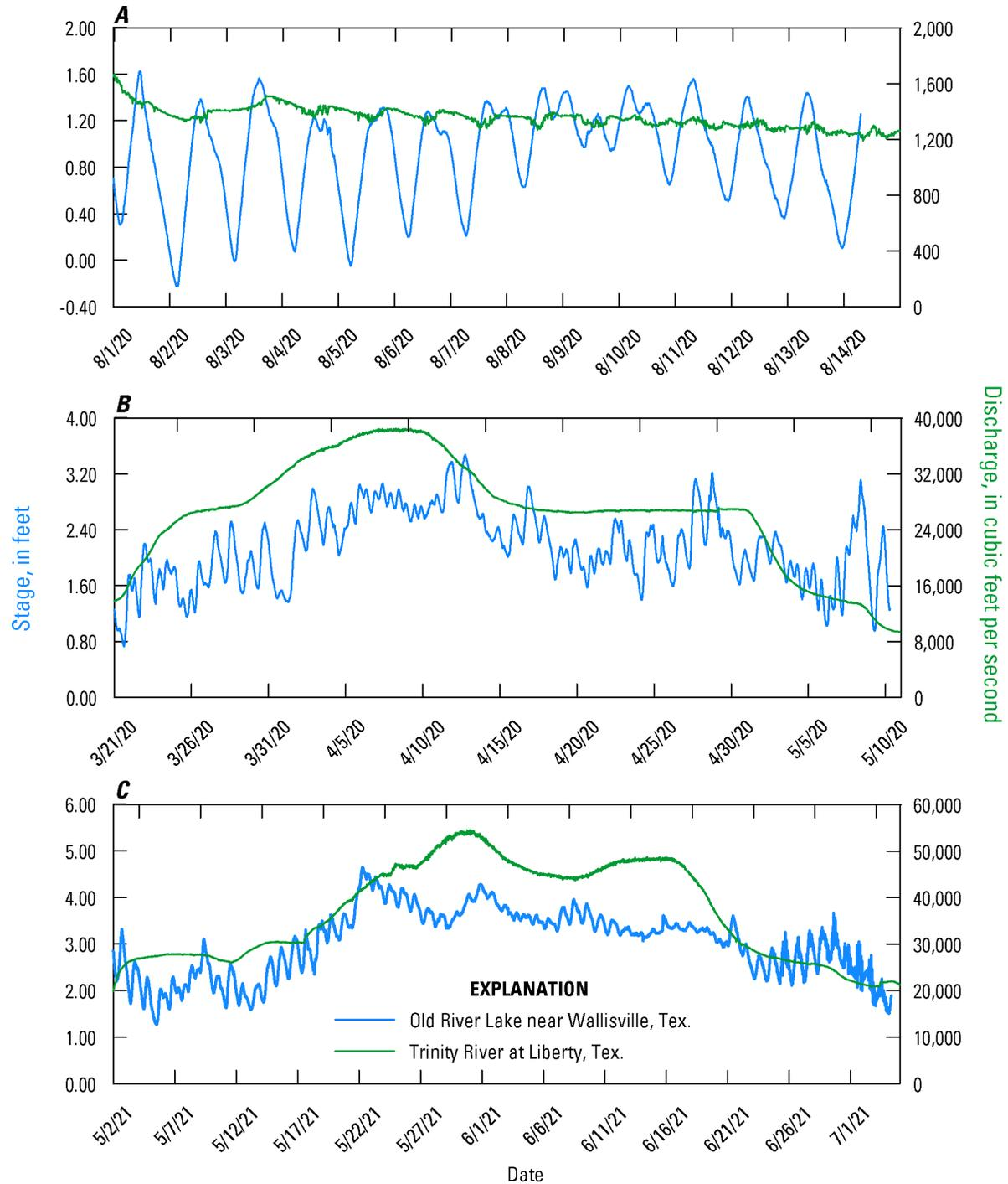
Figure 4. Stage at USGS station 08067230 Old River Lake near Wallisville, TX and discharge at 08067000 Trinity River at Liberty, TX on *A*, August 1–August 15, 2020 (baseflow conditions), *B*, March 21–May 10, 2020 (high-flow event), and *C*, May 2–July 4, 2021 (high-flow event).
