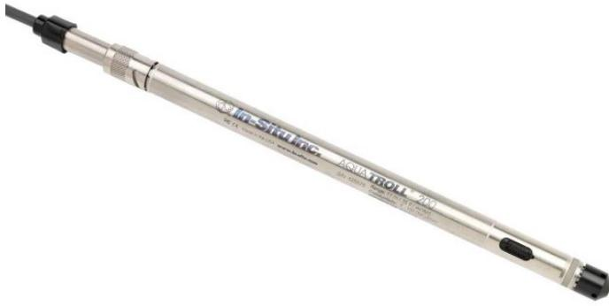
Each of the cables connects the telemetry system to an In-Situ AquaTROLL 200 transducer. This device measures, records, and reports water pressure (depth of water), temperature and conductivity (an indicator of water quality). More information on the telemetry unit and transducers can be found in Appendix B.
