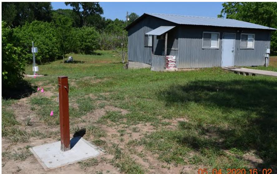
Monitor Wells 1 and two are on the lower portion of the PB-Vista site. This picture shows Monitor Well 3 and the telemetry station installed on the upper portion of the site. Pink flagging shows the location of the buried data cable conduit.
