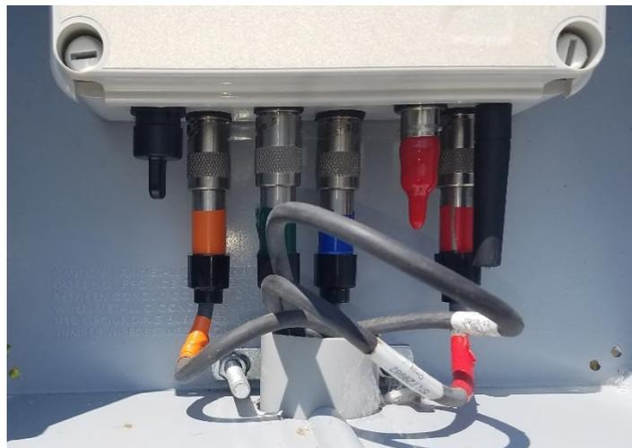
The In-Situ Cube 300 Telemetry unit which measure 7.87 inches wide, 7.1 inches high and 3.35 inches deep. This picture on the right shows the individual connections to each transducer. The connections are color-coded: Red – River Gauge; Orange – Monitor Well 1; Blue – Monitor Well 2 and Green – Monitor Well 3.
