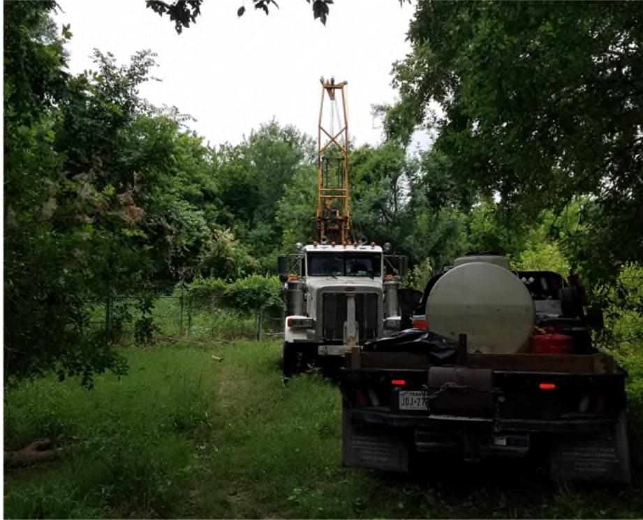
Auger-rig drill truck and support truck on drill location at Study Site No. 1.
