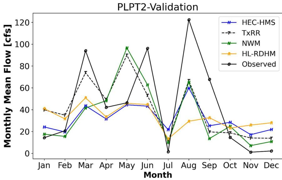
Figure 5-16 Mean monthly observed flow and simulated flow from four member models for each gauged watershed over the validation period.
