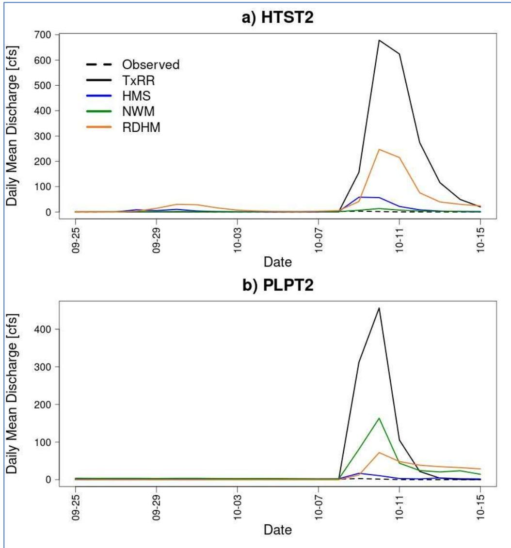
**Figure 5-22 Comparisons of simulated flow from member models and observation for during the drought of 2011 (Part II).**
