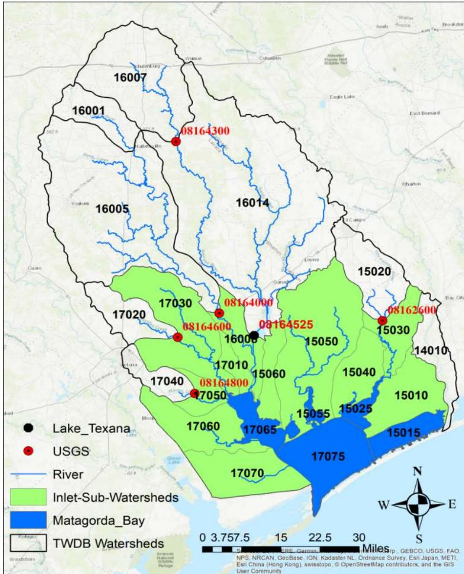
**Figure 3-2** Gauged and ungauged watersheds that drain to Matagorda Bay. The locations of USGS gauging stations and identifiers are marked in red. The outlet for Lake Texana is highlighted in black.
