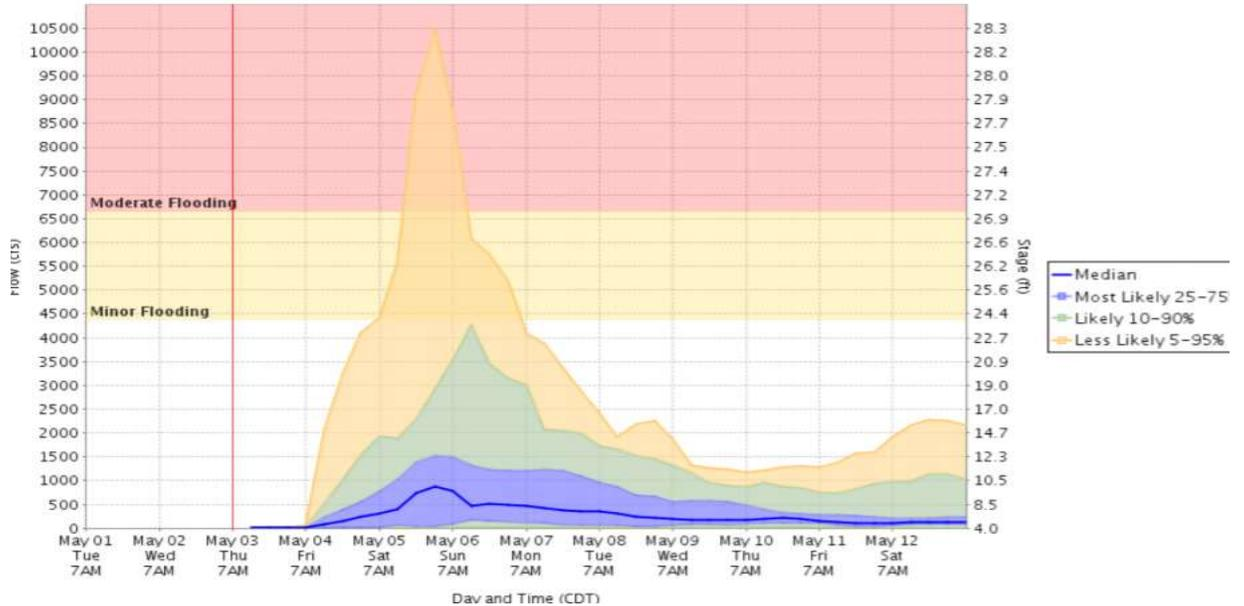
**Figure 6-1** Example of ensemble stage prediction generated by WGRFC. Source: NWS
