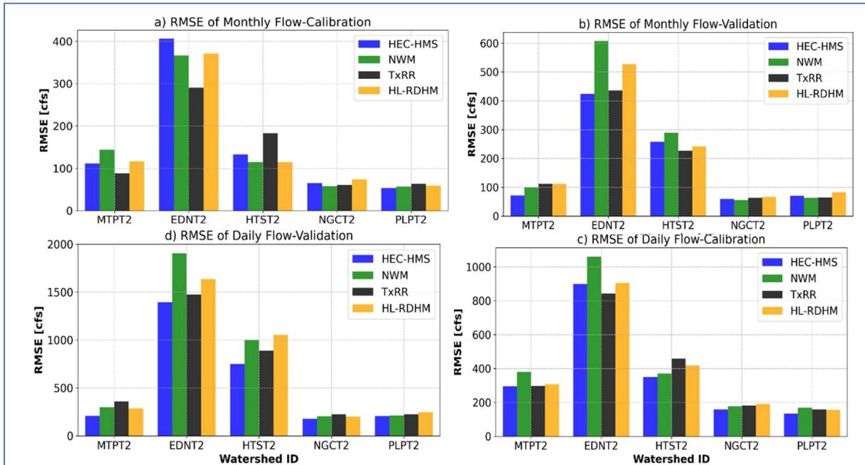
**Figure 5-14 Comparisons of RMSE between simulated flow by the four member models and observed flow at five upstream USGS stations (marked using SHEF ID). Shown are the results computed at monthly and daily scales, and for the calibration and validation periods.**
