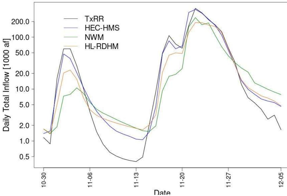
**Figure 5-28** Inflow time series for the event of Oct-Nov 2004. Note that TxRR flow recedes to a lower level after each peak.
