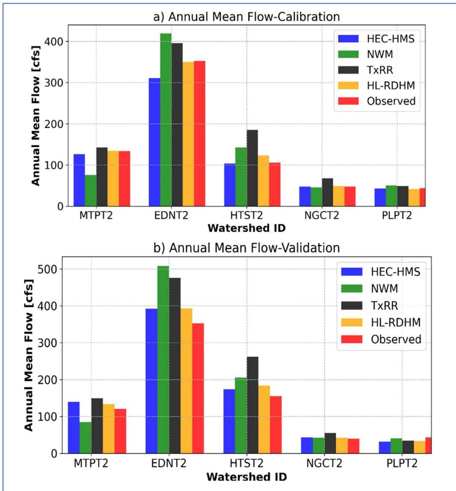
Figure 5-11 Comparisons of annual mean flow produced by the four member models for the five USGS stations. Shaded rectangles mark observed flow.
