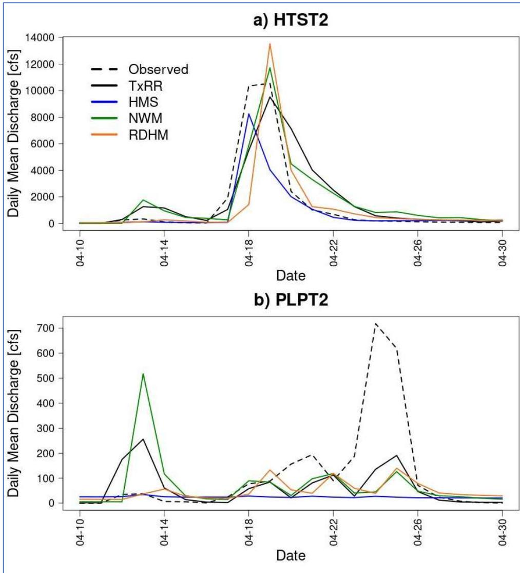
**Figure 5-19** Comparisons of simulated flow from member models and observed for the Apr. 2014 storm event.
