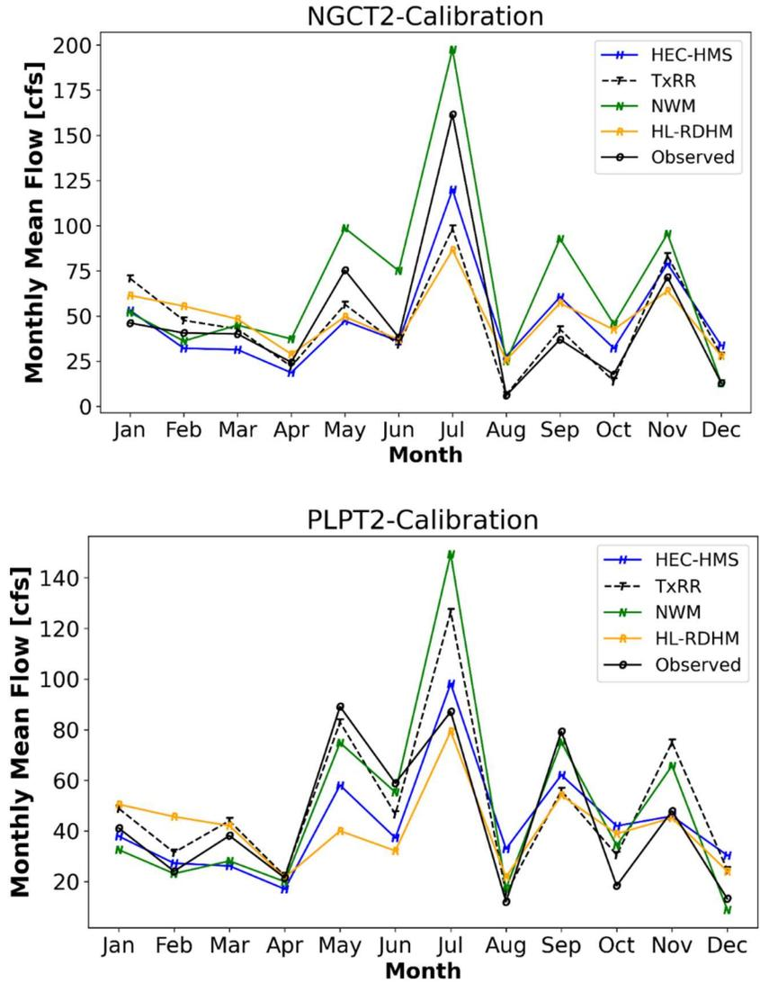
Figure 5-15 Mean monthly observed flow and simulated flow from four member models for each gauged watershed over the calibration period.
