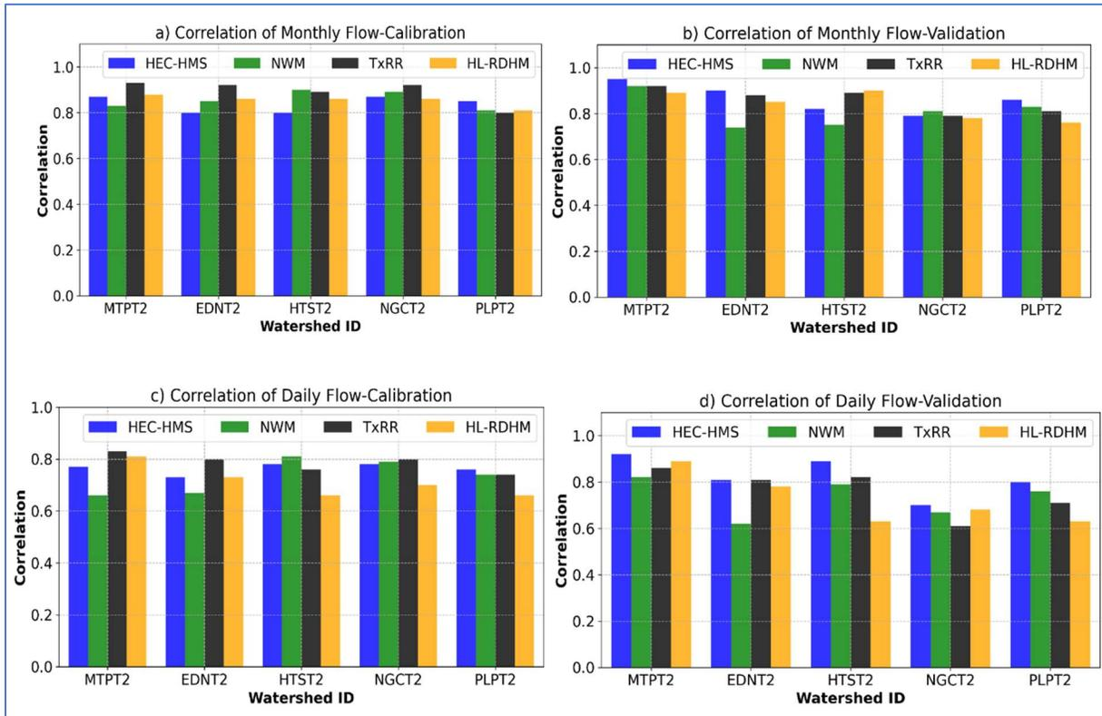
**Figure 5-13** Comparisons of correlation between simulated flow by the four member models and observed flow at five upstream USGS stations (marked using SHEF ID). Shown are the results computed at monthly and daily scales, and for the calibration and validation periods.
