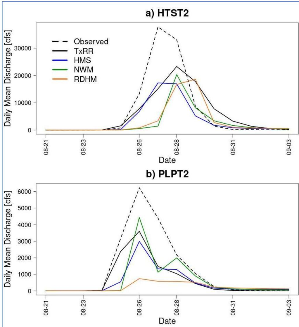
**Figure 5-20** Comparisons of simulated flow from member models and observed for Hurricane Harvey in Aug-Sep 2017.
