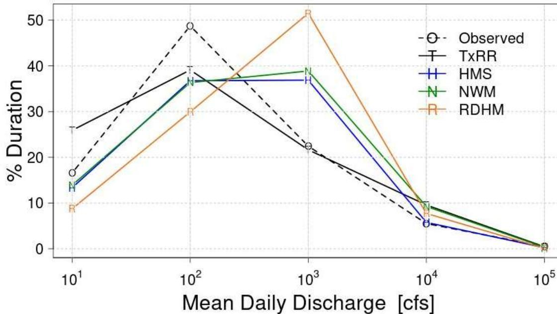
Figure 5-29 Flow duration curves for observed and simulated discharge series at EDNT2 (Lavaca River at Edna).
