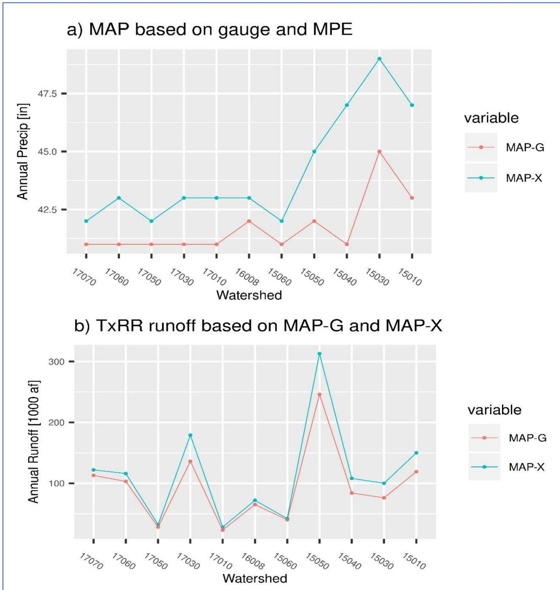
**Figure 4-1** Differences between a) mean annual MAPs based on gauge (MAP-G) and MPE data (MAP-X), and b) simulated inflows using respective data sets for each ungauged watershed that drains to Matagorda Bay. The watersheds are sorted roughly from the west to east. Note that the differences in MAPs tend to be larger toward the east where annual precipitation is higher.
