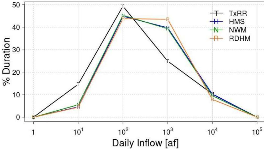
**Figure 5-27** Flow duration curves based on simulated daily inflow by each model. Each point represents the percentage of time that total daily aggregate inflow volume by a given model is within a category marked by the corresponding abscissa and its preceding one.
