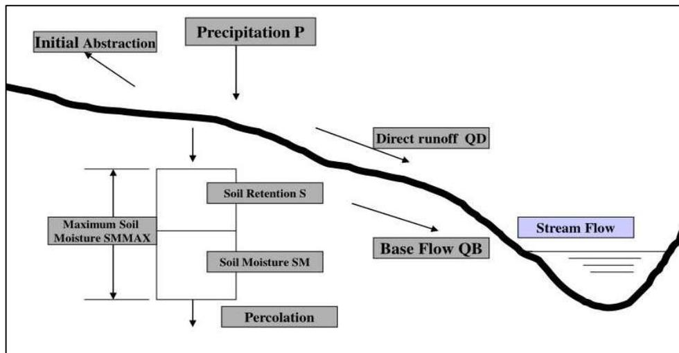
Figure 2-1 Schematic of Texas Rainfall-Runoff (TxRR) model. Source: the TWDB.
