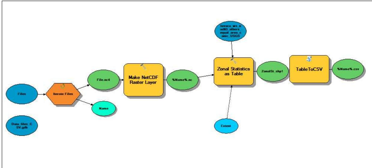
Figure 9-1 Schematic of the process of creating mean areal precipitation for HEC-HMS.
