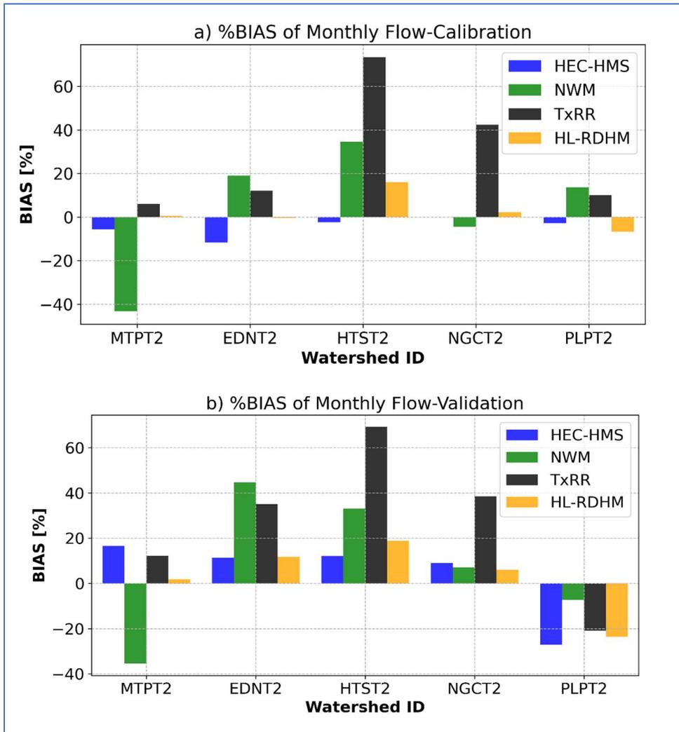
**Figure 5-12** Comparisons of percentage bias between simulated flow by the four member models and observed flow at five upstream USGS stations (marked using SHEF ID). Shown are the results computed at monthly scale, and for a) calibration and validation (b) periods.
