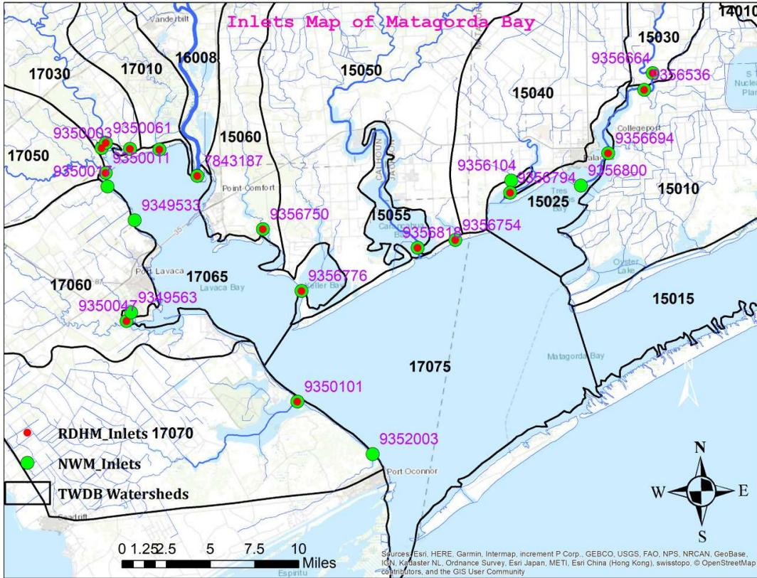
**Figure 5-23** Map of bay inlets identified from NHD-Plus used in NWM (yellow) and HL-RDHM (red). Superimposed in purple are segment identifier from NHD-Plus.
