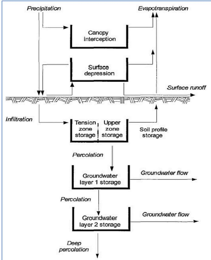
**Figure 5-3** Schematic of HEC-HMS surface and loss models. Note the Soil Moisture Accounting is chosen as the loss model for this implementation.
