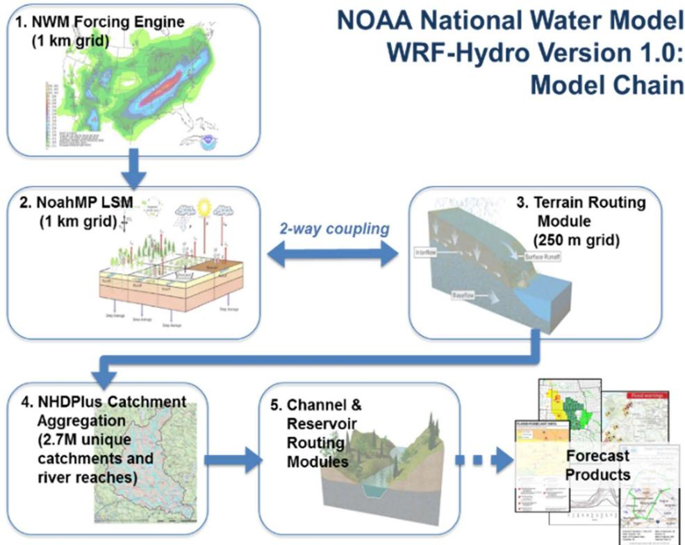
Figure 5-7 Components of NWM and data flow diagram. Note the diagram applies to NWM 2.1 that is the current operational version. Source: NWS OWP.
