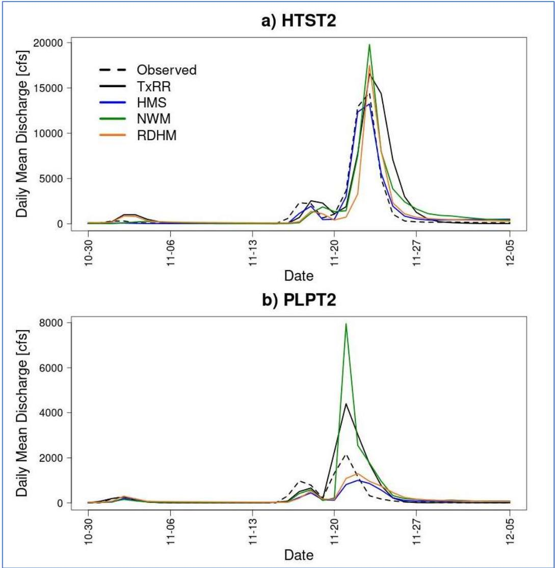
**Figure 5-17** Comparisons of simulated flow from member models and observed for the Nov. 2004 storm event.
