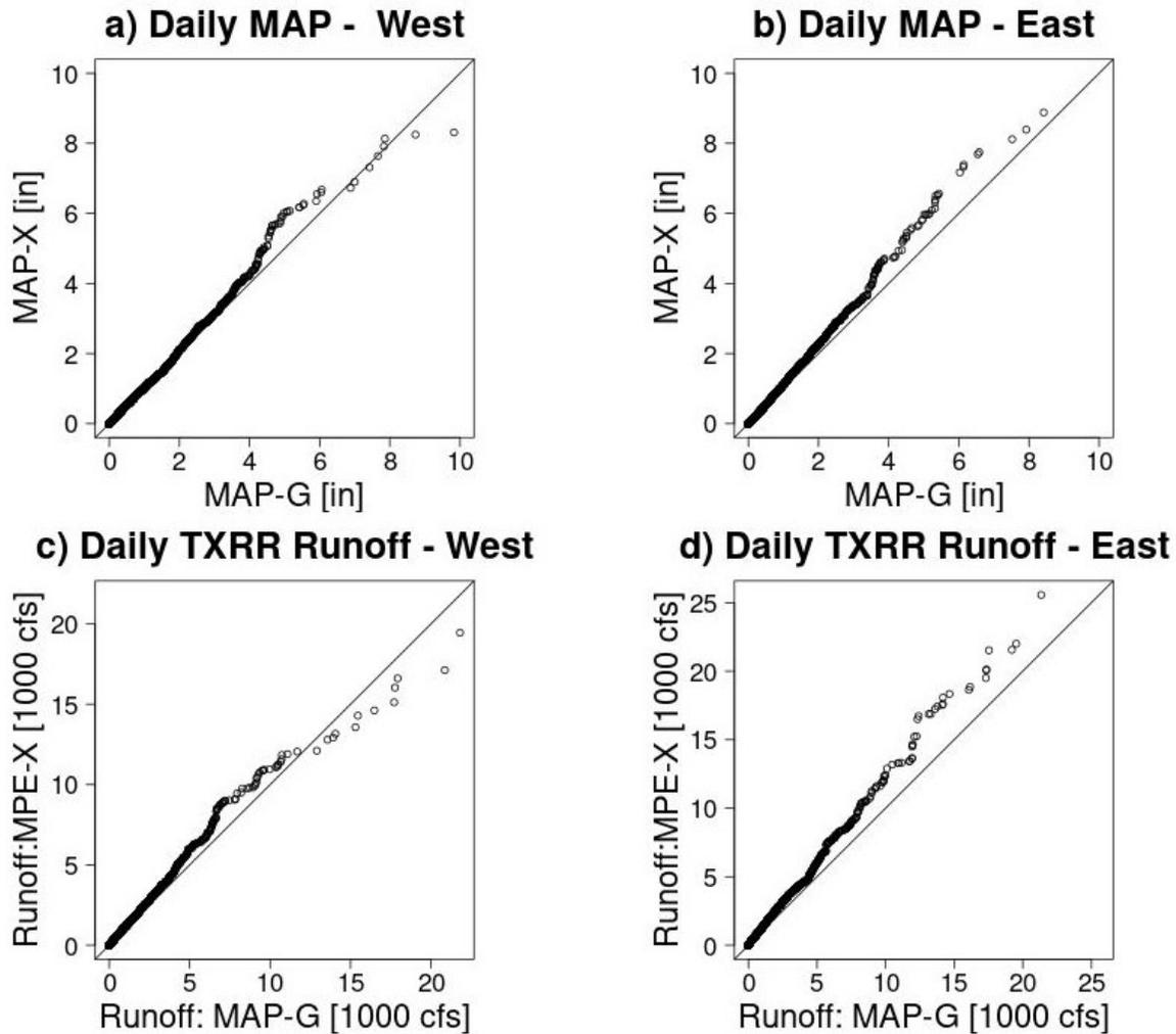
**Figure 4-2** Quantile-quantile plots of daily MAP and corresponding daily TxRR simulated runoff coastal watersheds located over the west and east portion of the bay. The list of watersheds for each group can be found in Table 4-1.
