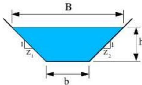
**Figure 9-5** An example of trapezoidal channel cross-section used in HEC-HMS routing calculation.
