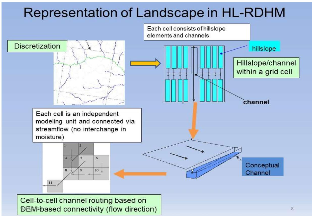
**Figure 5-5** Schematic of HL-RDHM routing model. Upper-left: an example of channel links from NHD-Plus; upper-right: a schematic of hillslope model within each model pixel; lower-left: a schematic of lateral flow from hillslope to the channel; and lower-right: routing of channel flow across model pixels
