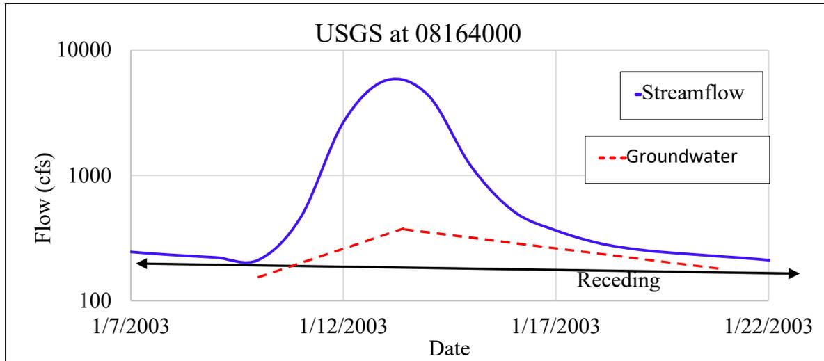
**Figure 9-4 Schematic for separating groundwater contribution to streamflow.**
