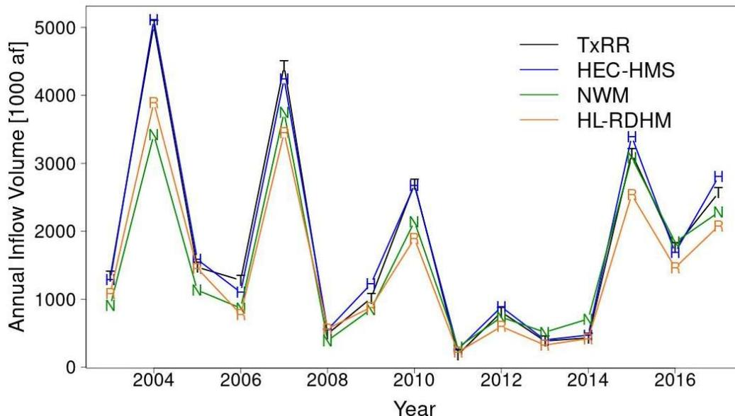
**Figure 5-24 Time series of annual freshwater inflow calculated from the four models that comprise the MMIPS, namely i)TxRR, ii) HEC-HMS; iii) NWM and iv) HL-RDHM.**
