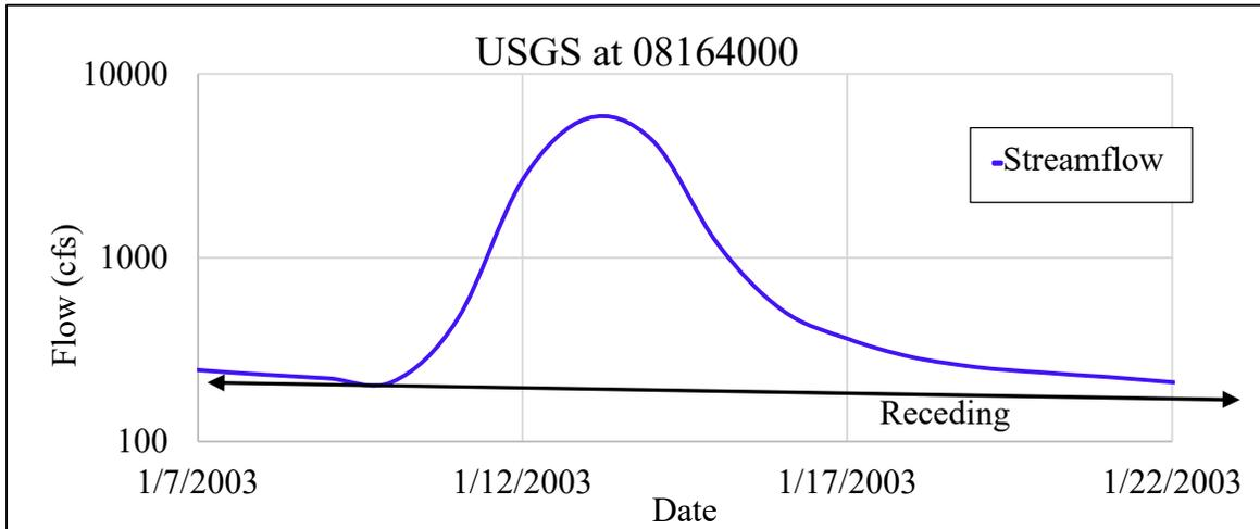
**Figure 9-3** Example hydrograph for recession analysis.
