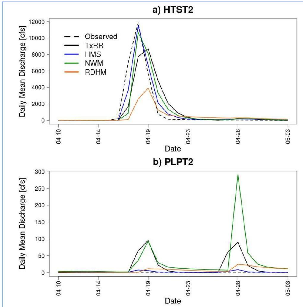
**Figure 5-18** Comparisons of simulated flow from member models and observed for the Apr. 2009 storm event.
