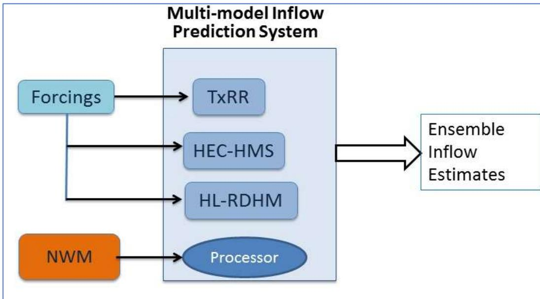
Figure 5-1 Schematic of the multi-model inflow prediction system.
