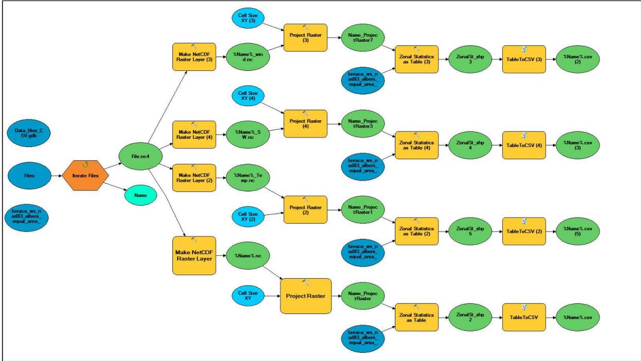
**Figure 9-6** Schematic of Model Builder tool in ArcGIS for computing basin average forcings from NLDAS gridded forcing data set
