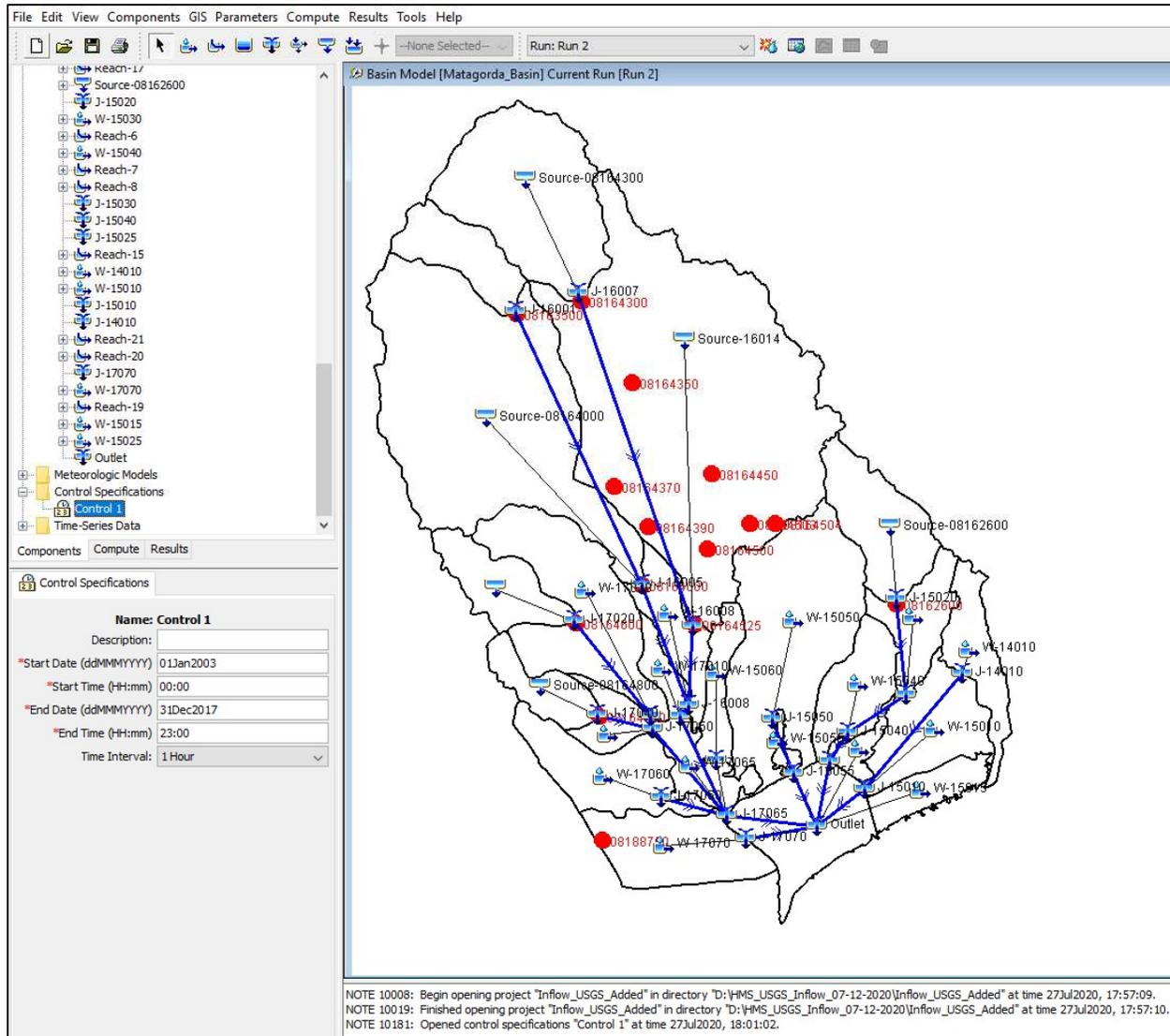
Figure 9-7 Control specification for HEC-HMS model.
