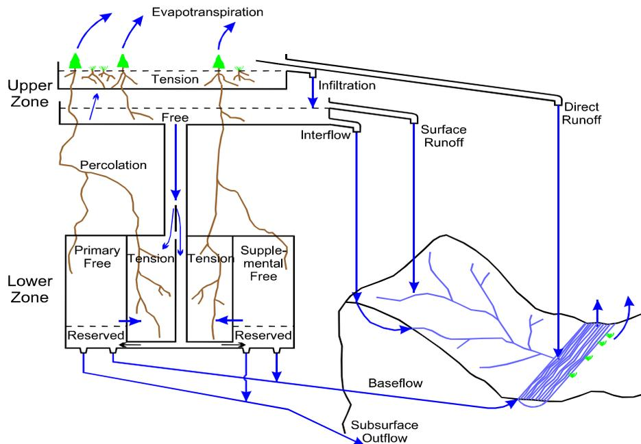
Figure 5-4 Schematic of SAC-SMA model.
