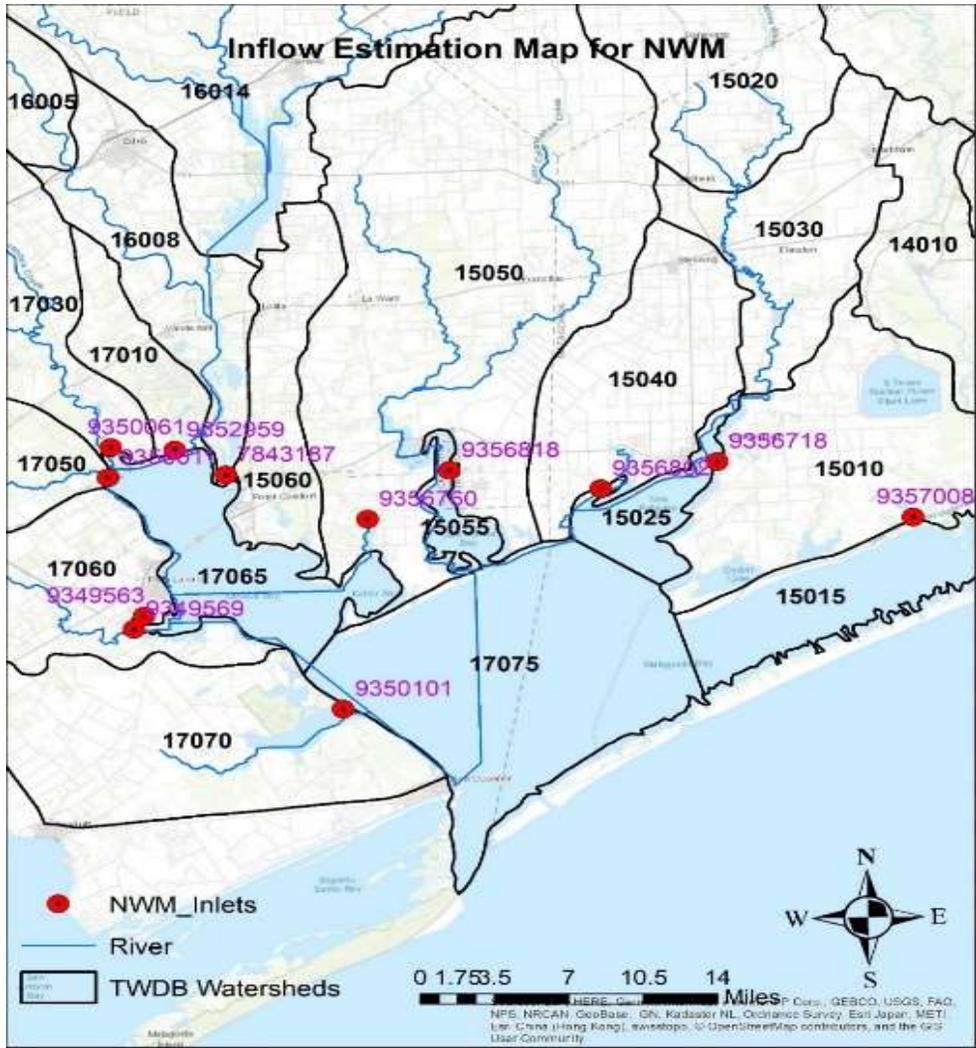
Figure 5-10 NWM inlets to Matagorda Bay. The inlets were determined from the NHD-plus database. Source: NCAR.
