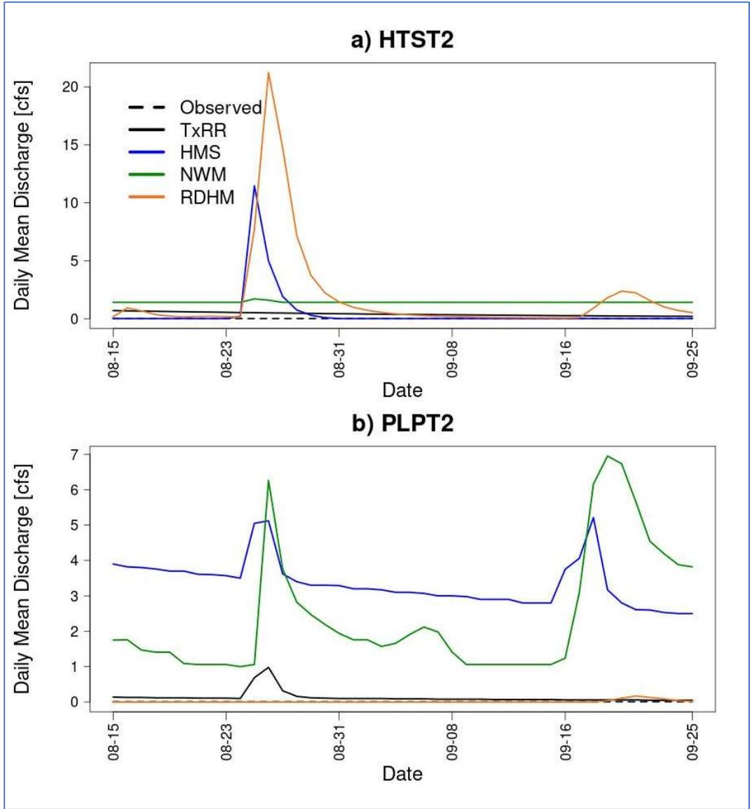
**Figure 5-21** Comparisons of simulated flow from member models and observation for during the drought of 2011 (Part I).
