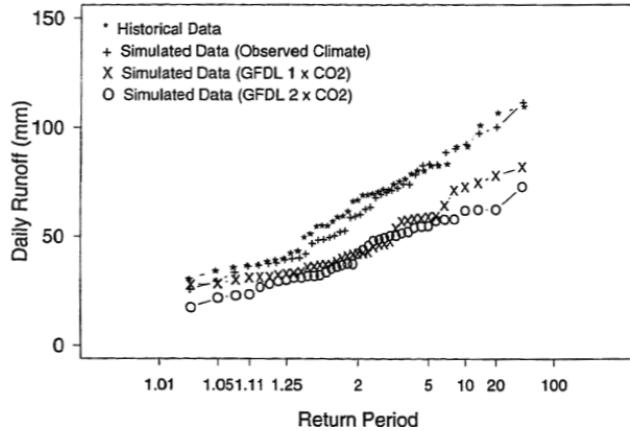
Figure 3.1: Daily flood-flow frequency curve for the Satsop River from Hughes and others (1987).
