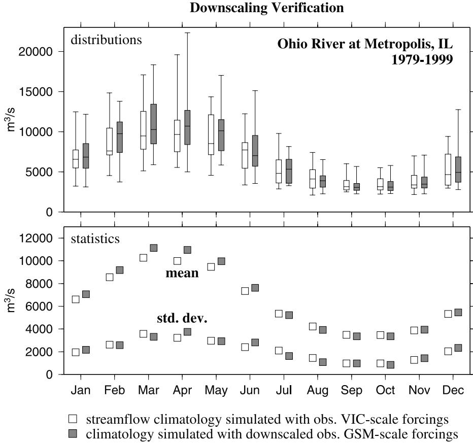
Figure 3.2: Climatology period (1979–1999) streamflow distribution simulated from daily VIC 1/8° observations compared with parallel simulation from monthly GSM-scale ( $2.8125^\circ$ ) spatially-averaged observations after downscaling and disaggregation procedure. (This figure is Figure 5 reproduced from Wood et al. (2002).)
