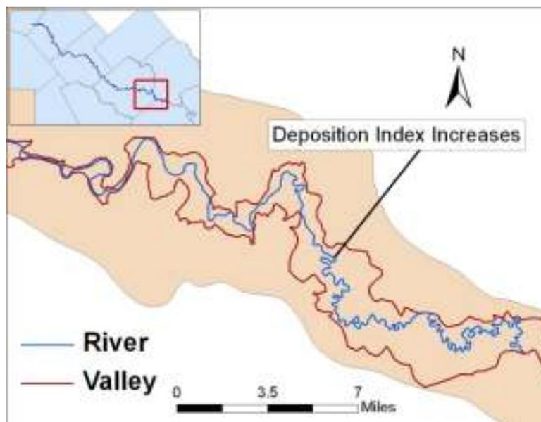
**Figure 23. Deposition Index Increase.** The index increases at river kilometer 284.
