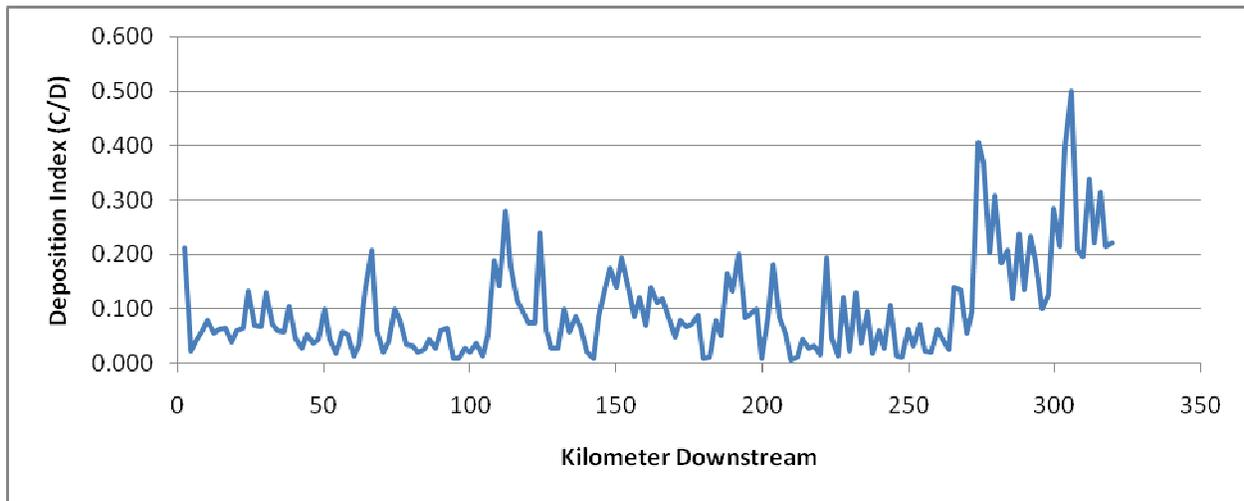
**Figure 22. Deposition Index per Kilometer.** A significant increase occurs at km 274.
