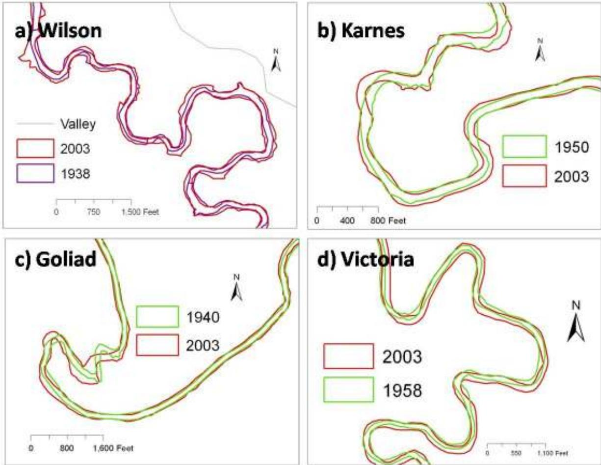
**Figure 24. County Channel Change.** a) Large slumps, widening, and little migration are common in Wilson County. b) Widening and migration at a few bends was observed in Karnes County. c) Migration and channel widening were observed in Goliad County. d) The fastest migration rates were observed in Victoria County. Nearly all of the bends had migrated.
