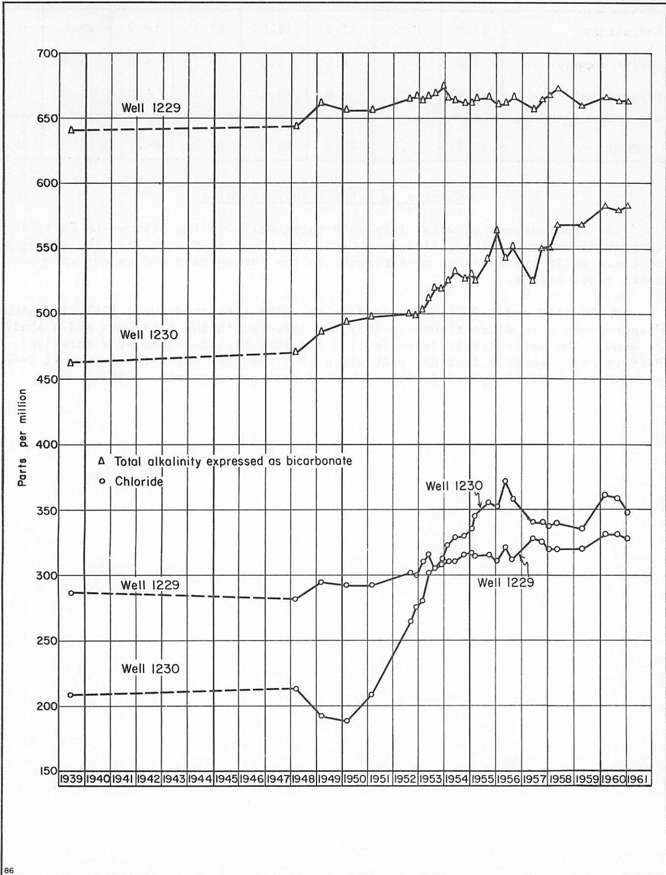
FIGURE 23.- Chloride content and total alkalinity of water from Harris County wells 1229 and 1230
