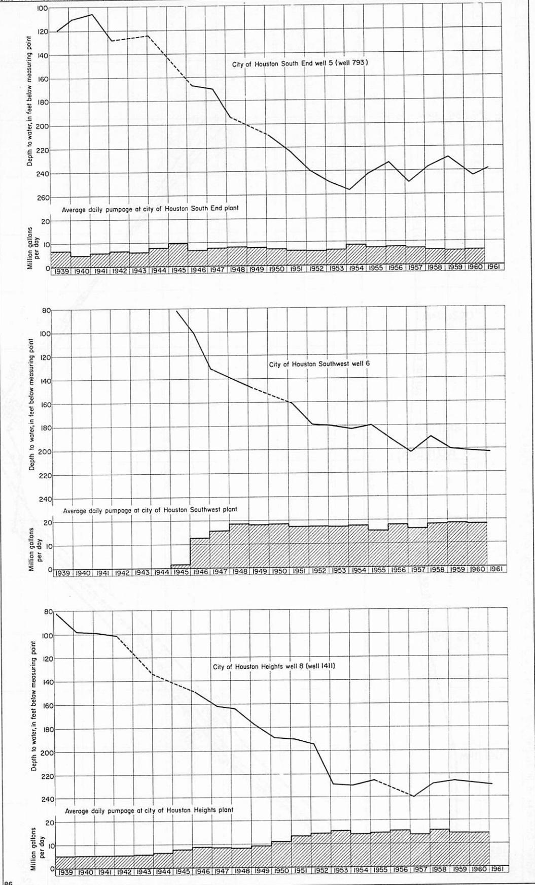
FIGURE 8.—Relation of pumpage to depth to water in the South End, Southwest, and Heights well fields of the city of Houston
