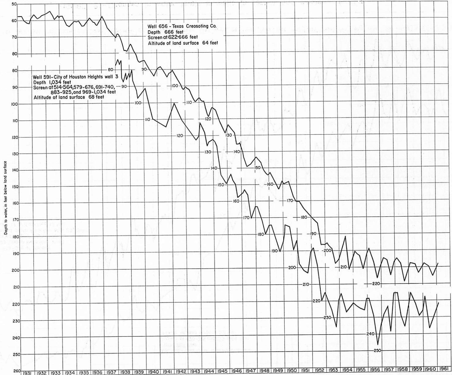
FIGURE 20.—Changes in water levels in wells in northern Houston
