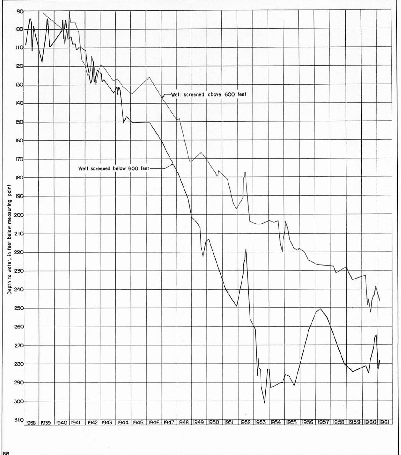
FIGURE 16.—Changes in water levels in a shallow well and a deep well in the eastern part of the ship-channel subarea
