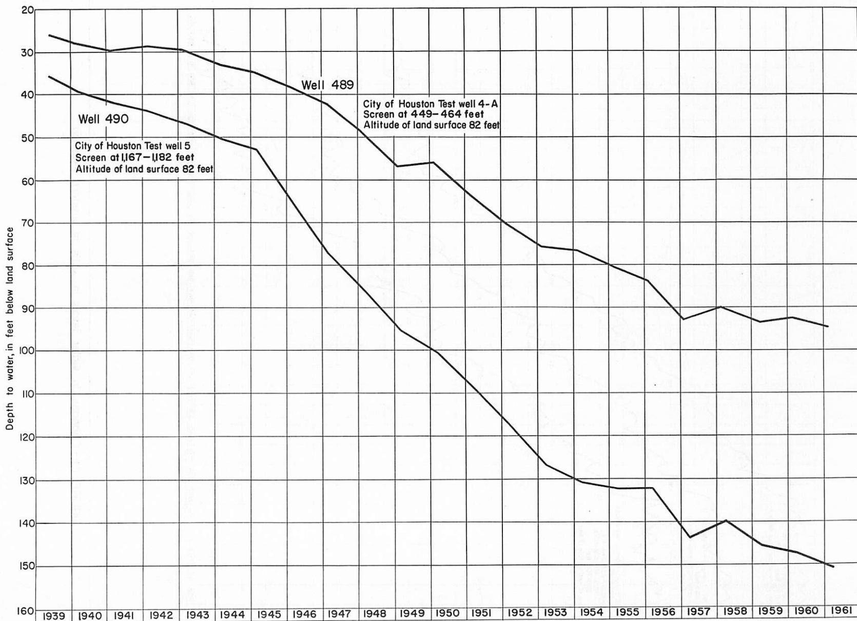
FIGURE 18.—Changes in water levels in two single-screened wells of different depths near Alief
