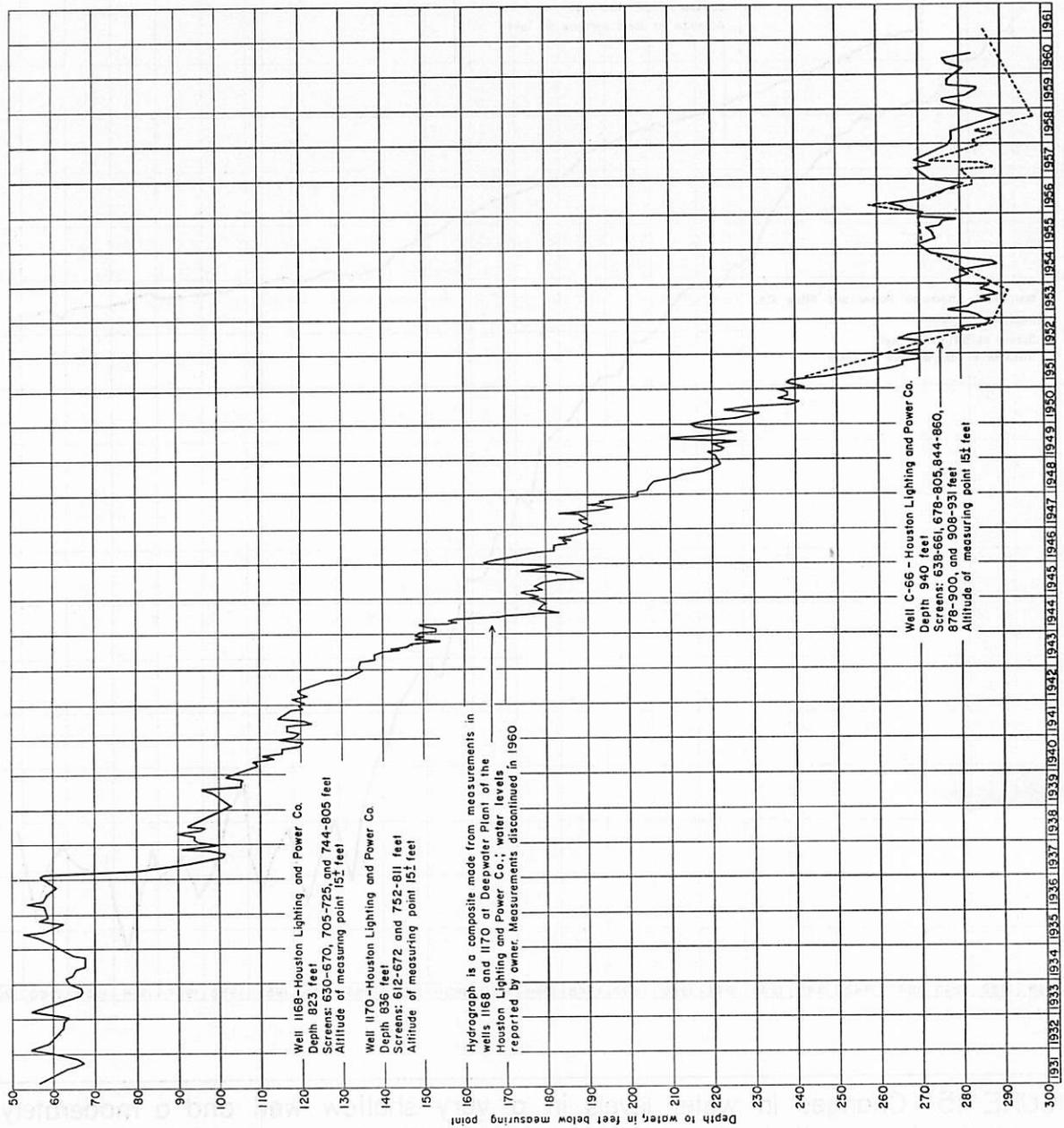
FIGURE 14.- Changes in water levels in Harris County wells 1168, 1170, and C-66
