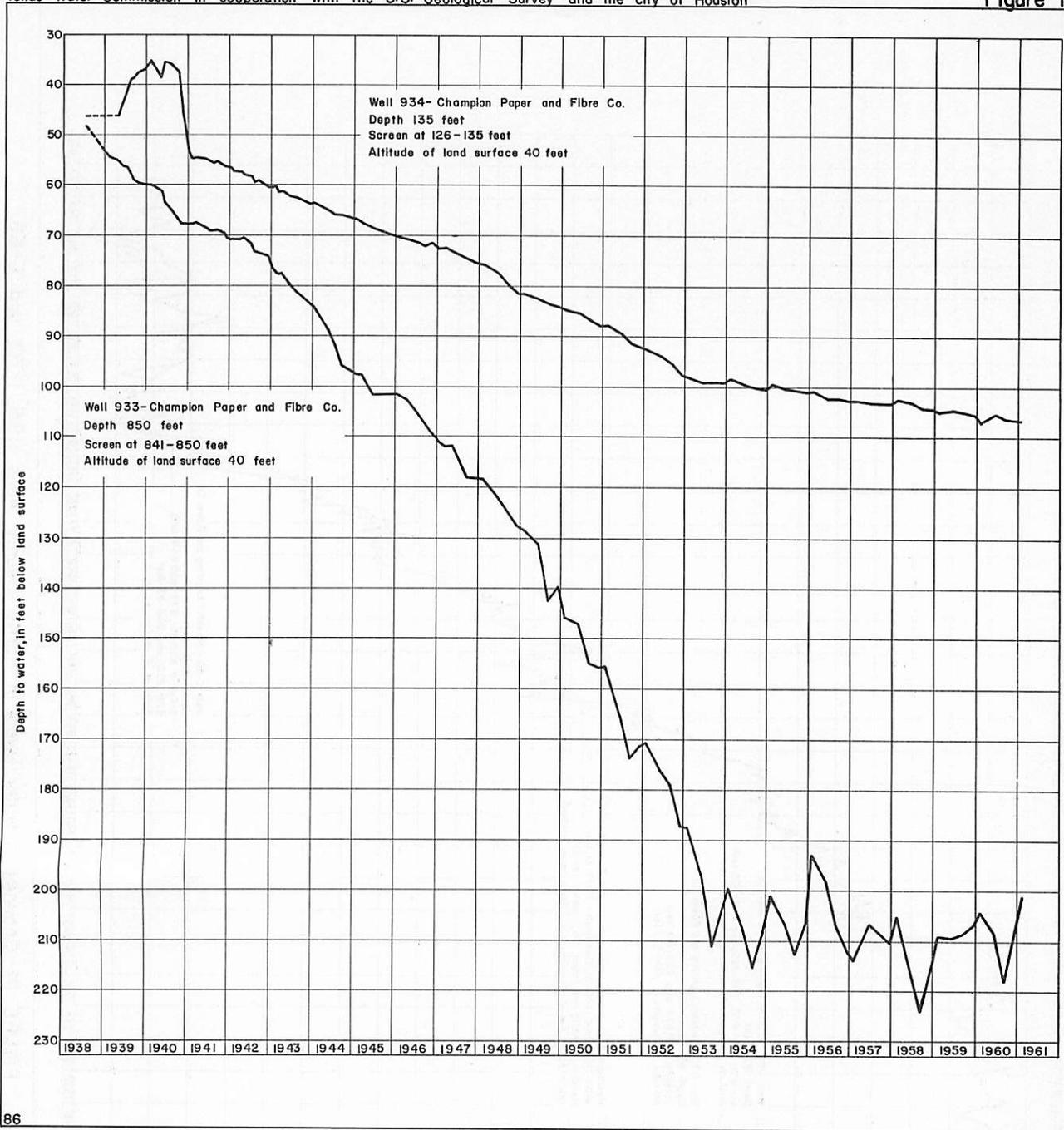
FIGURE 15.-Changes in water levels in a very shallow well and a moderately deep well in the northern part of the Pasadena area
