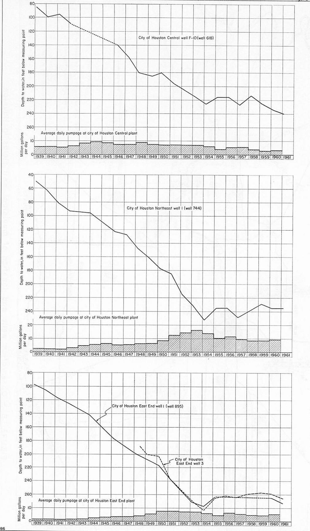
FIGURE 7--Relation of pumpage to depth to water in the Central, Northeast, and East End well fields of the city of Houston
