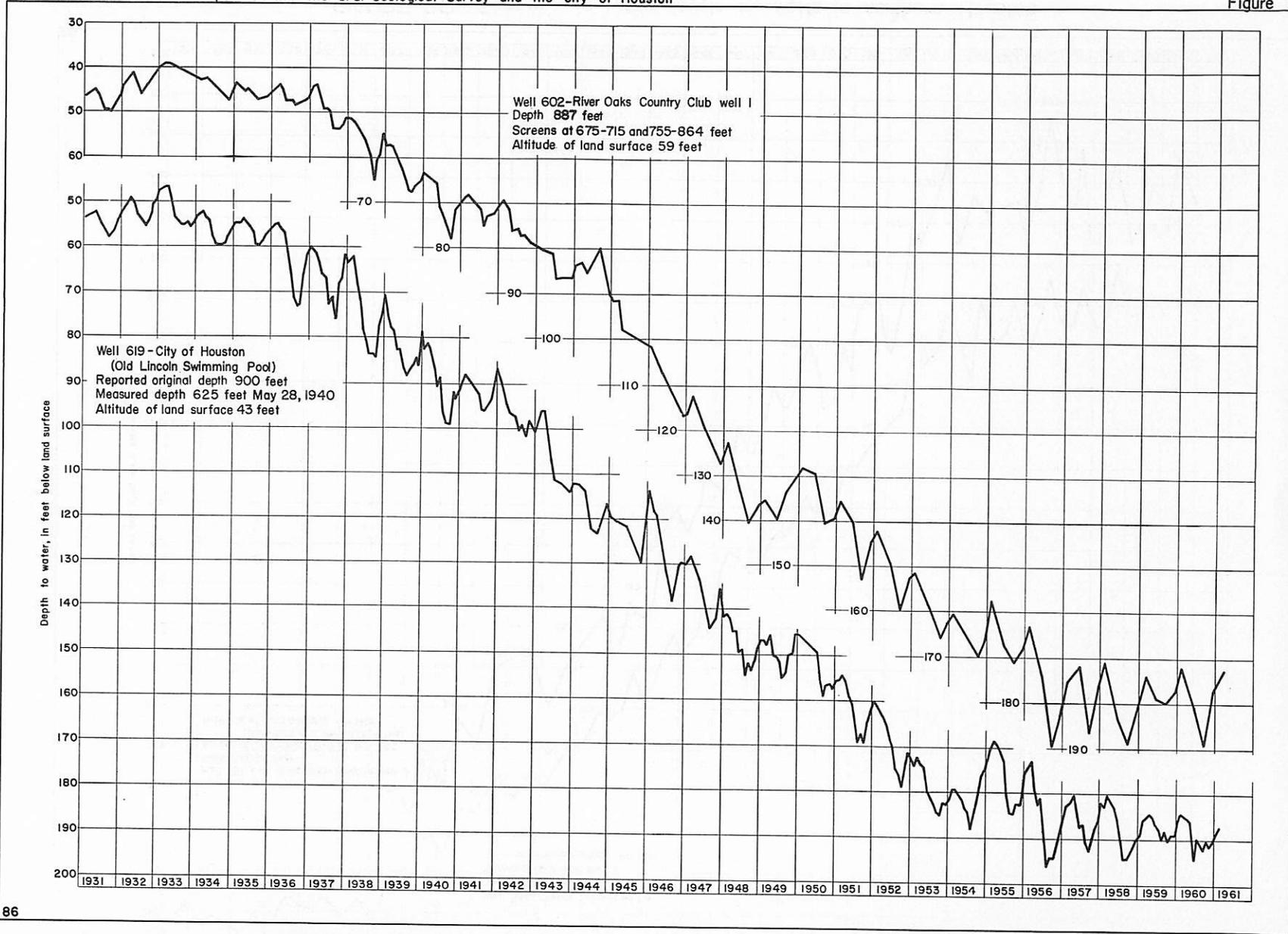
FIGURE 21.-Changes in water levels in wells in central and western Houston
