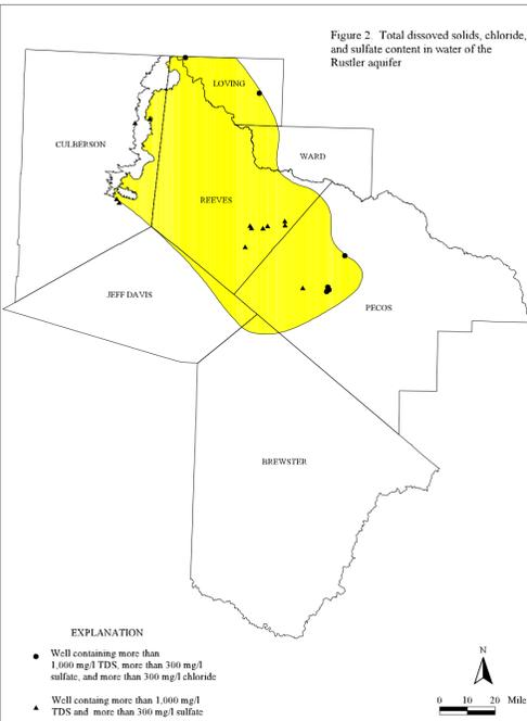
Figure 2. Total dissolved solids, chloride, and sulfate content in water of the Rustler aquifer.
