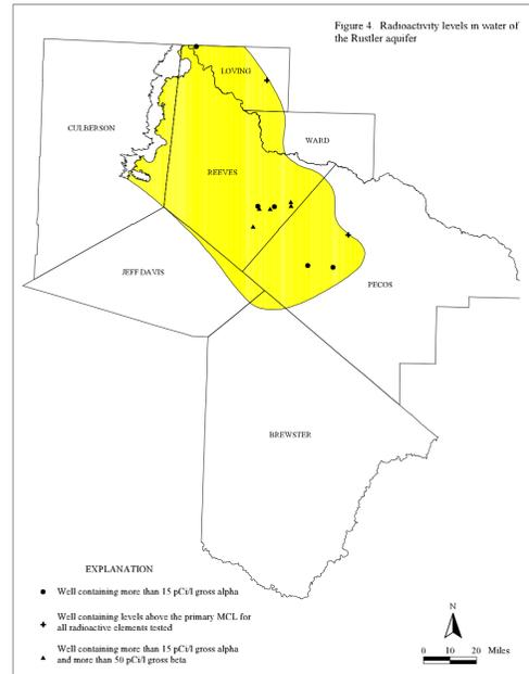
Figure 4. Radionuclide levels in water of the Rustler aquifer.
