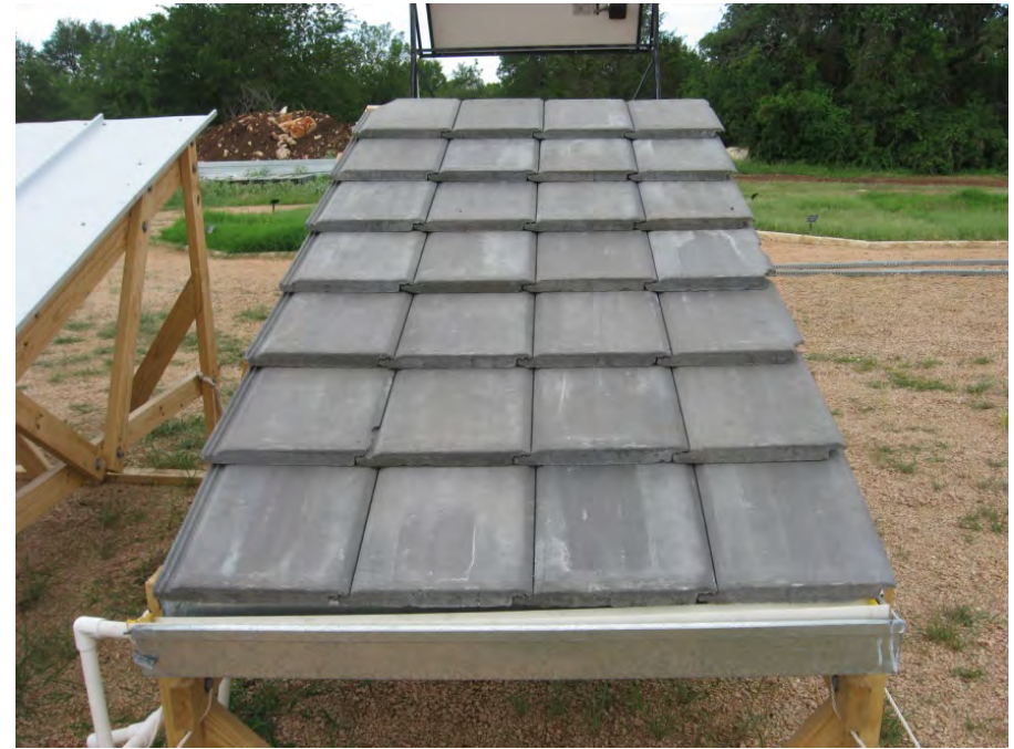
Concrete tile roof (Lady Bird Wildflower Center, Austin)
