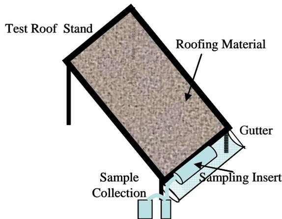
**Figure 1. Sampling Apparatus and Test Roof Set Up for Harvesting Rainwater**
