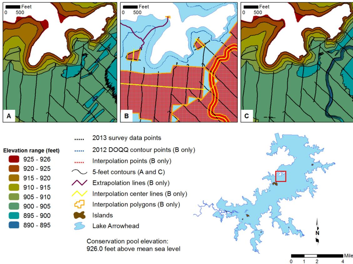
**Figure 3. Anisotropic spatial interpolation and linear extrapolation of Lake Arrowhead sounding data - A) bathymetric contours without interpolated points, B) sounding points (black) and interpolated points (red), C) bathymetric contours with the interpolated points**
