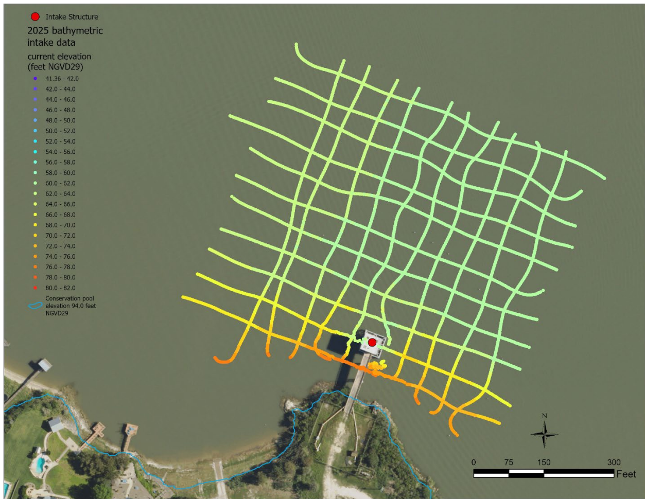
Figure 6. Alice intake bathymetric data. Background photography collected on April 29, 2023, while the daily average water surface elevation measured 90.37 feet.
