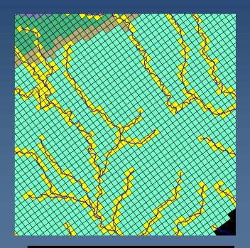
Streams are discretized unto The model grid
